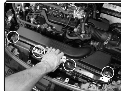
7. Loosen the 4 bolts holding in the OEM air box ram scoop and remove.
