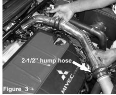
Install the 2-1/2" hump with clamps provided to the factory intercooler pipe. Install the longer pipe and connect the 2 pipes together. Position for best fit, re adjust if necessary. Tighten all clamps using 8mm nut driver. Your installation is now complete.
