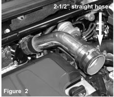
Install the short pipe to 2" straight hose. Attach the 2-1/2" straight hose with clamps provided to other end of pipe. Do not tighten.
