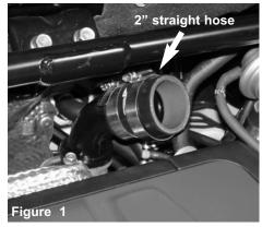
Loosen and remove the OEM intercooler pipe. Install the provided 2" staight hose with clamps provided to turbo housing. Tighten clamp on housing only
