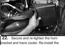
trans cooler cover. Re-install bumper cover and re-connect sensors and camera.
