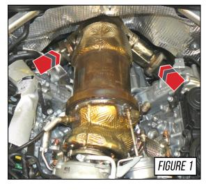
Start by removing the two (2) 12mm nuts on the driver side flange along with the three (3) 12mm nuts on the passenger side flange, as shown by the arrows in **Figure 1**. Five (5) nuts in total can be accessed from the engine bay.
