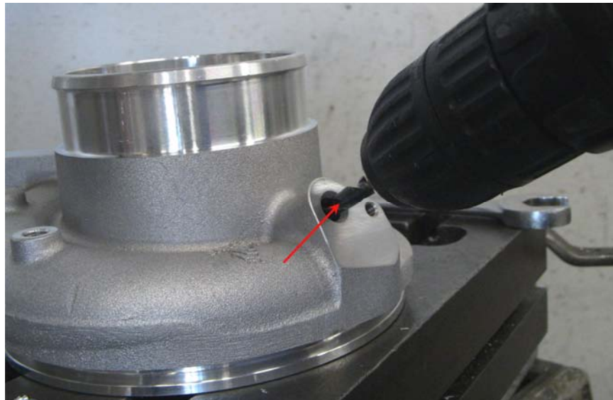
Figure 66: Drilling the 1/4" Hole
