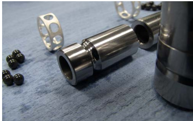
Figure 25: Bearing Disassembled; M50 Races, Metal Cages, Ceramic Balls
