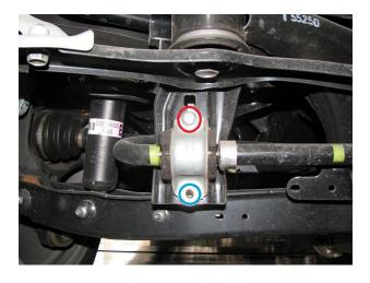
**6.5.** Install the front bracket into the lower sway bar mount location as shown below.
