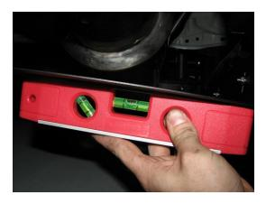
6.16. To keep the bottom of the outside strakes on the same plane as the bottom of the inside strakes, you need to line up the slots. This ensures that the strakes all hang down approximately the same amount. Once this is confirmed, you can tighten these (6) bolts and nuts. Below is a picture of the slots lined up and the strake installed with the diffuser installed at the lowest position.
