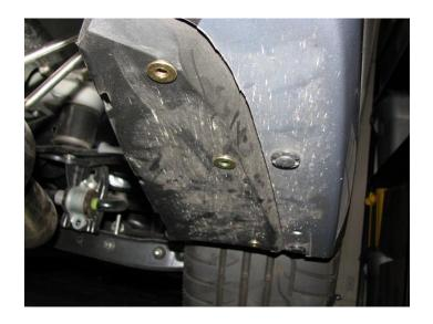
**6.10.** At this point, the main portion of the diffuser is ready to install. To install it, starting with the front brackets, we use a small BHCS, washer, and nut to bolt on the diffuser to the front tab.
