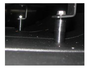
**6.12.** Loosely install the side mounting plates with the provided M6x1.0 x 16mm length BHCS with a washer above each. Place the side strakes between the main diffuser portion and the side mounting plate and using the M6x1.0 x 16mm BHCS, washers, and serrated nuts install it loosely as well. Below is a picture of the side plate installed loosely.
