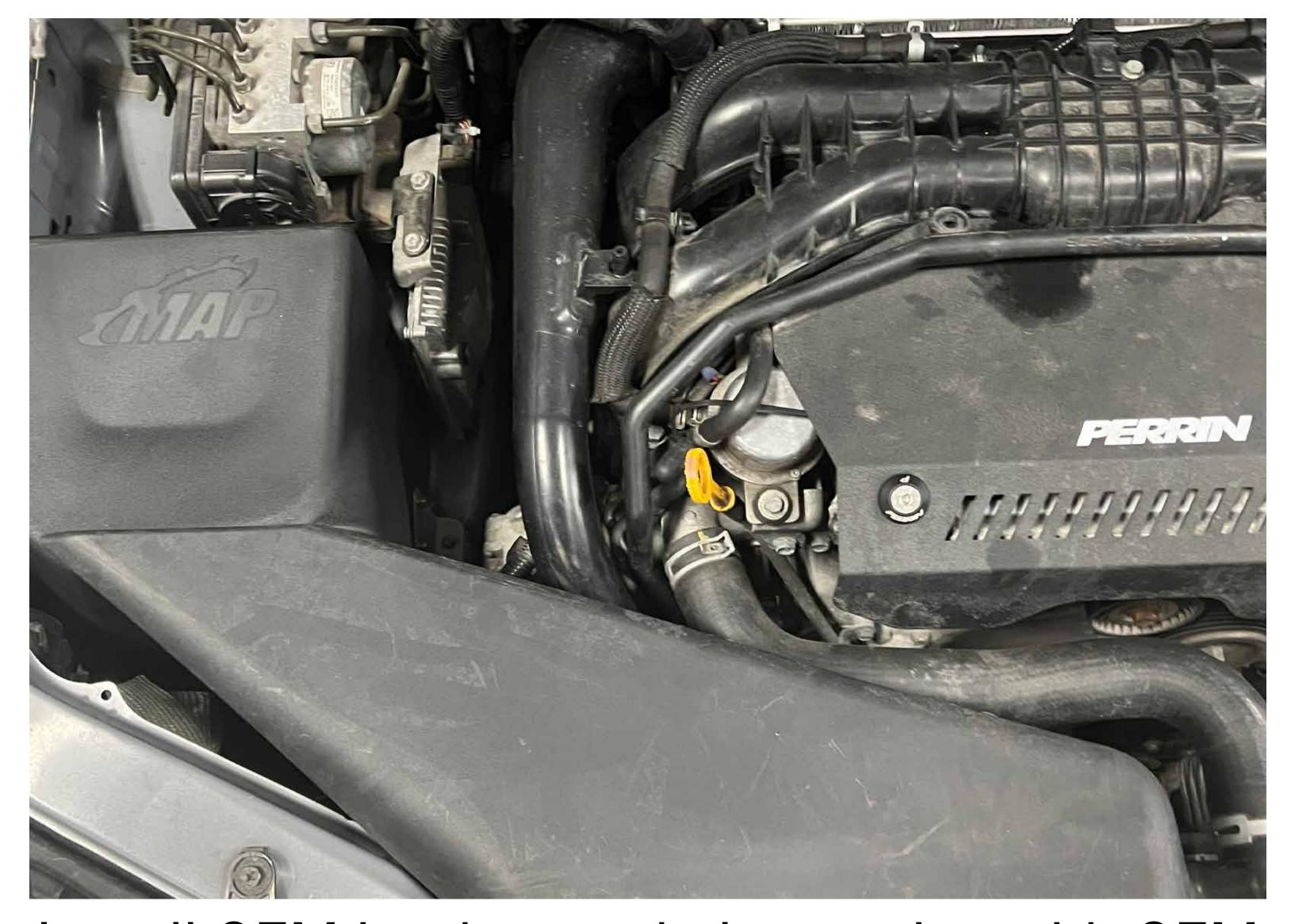
Install OEM intake snorkel, securing with OEM push pins
