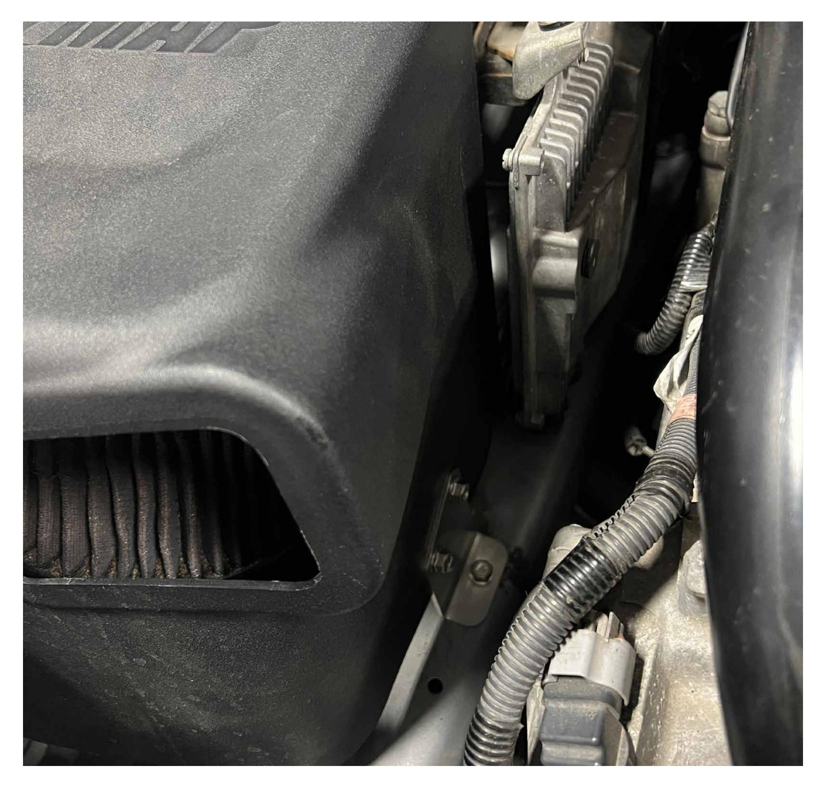
Install included 10mm bolt onto the vehicle, securing with the bracket
