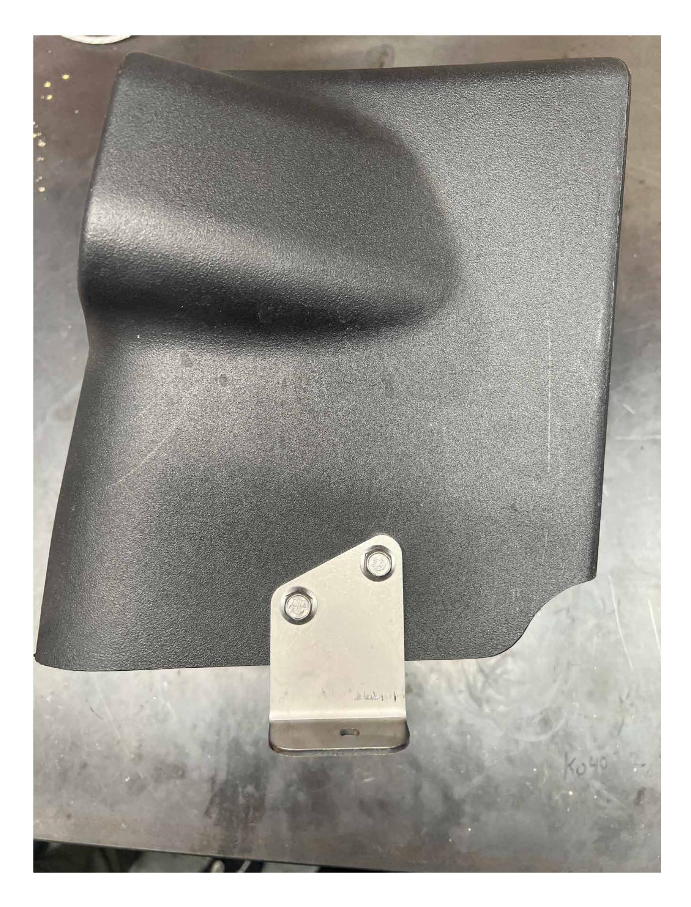
Install included bracket to airbox, securing using included hardware. Be sure to place washers on the inside of the airbox.
