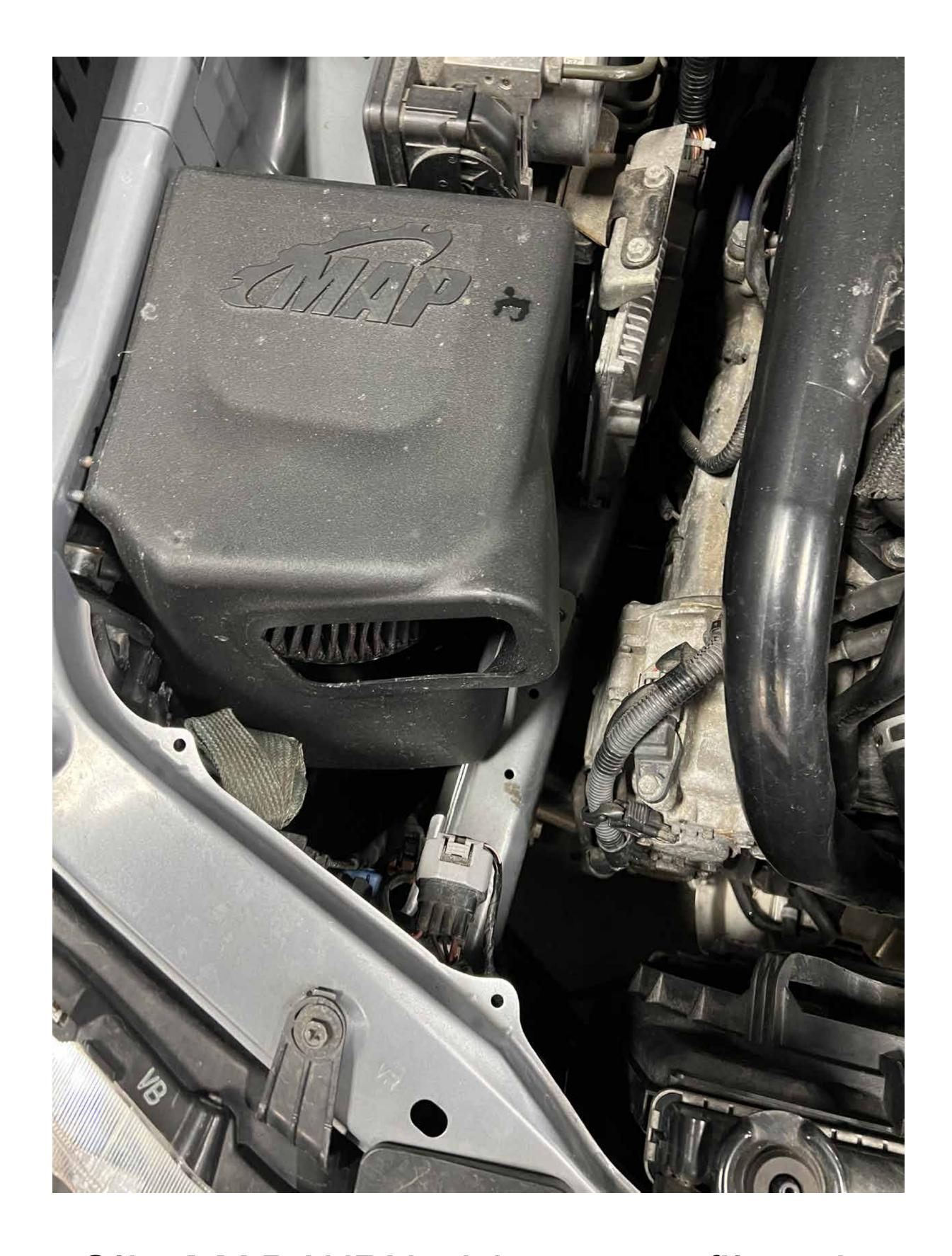
Slip MAP WRX airbox over filter, be sure the studs from the OEM filter bracket key into the holes on the MAP airbox
