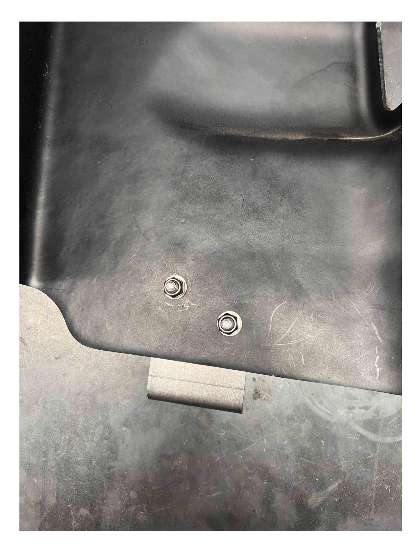
Install included bracket to airbox, securing using included hardware. Be sure to place washers on the inside of the airbox.
