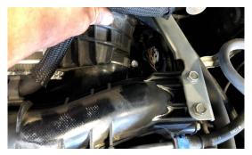
5. SLIDE INTERCOOLER AWAY FROM COUPLERS AND UP AND OUT OF THE ENGINE BAY
