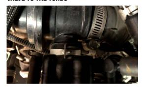
13. REMOVE VACUUM LINE FROM DIVERTER VALVE
