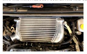
18. REINSTALL BRACKETS AND HOLDING BOLTS ONTO INTERCOOLER
