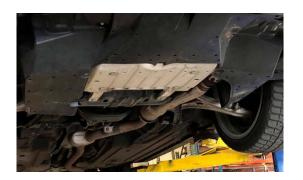
2. REMOVE ENGINE INTERCOOLER COVER
