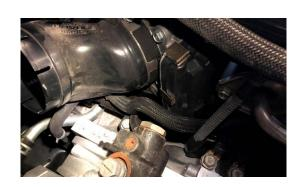
9. INSTALL NEW PROVIDED COUPLER ONTO THE THROTTLE BODY, REUSING WORM DRIVE CLAMP
