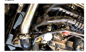
23. REMOVE YOUR STOCK DIVERTER VALVE FROM STOCK CHARGE PIPE
