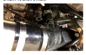
12. LOOSEN CLAMP FROM STOCK DIVERTER VALVE TO THE TURBO
