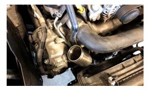
17. SLIDE NEW INTERCOOLER INTO ENGINE BAY, BE SURE THAT THE COLD SIDE SLIDES INTO THE THROTTLE BODY COUPER AND AND CLAMP IS INSTALLED
