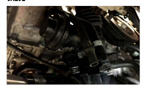
14. REMOVE STOCK CHARGE PIPE FROM ENGINE BAY
