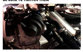
27. INSTALL NEW VACUUM LINE ONTO DIVERTER VALVE. ENSURE IT RUNS TO THE VACUUM REFERENCE YOU REMOVED EARLIER. SECURE WITH INCLUDED ZIP TIES
