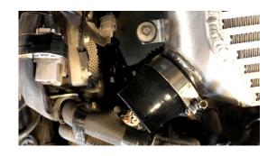
20. INSTALL EXPANDING ELBOW COUPLER ONTO LOWER CHARGE PIPE AND TIGHTEN CLAMPS
