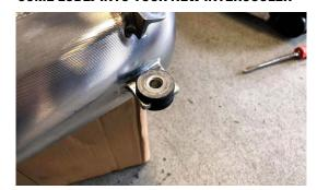
8. REMOVE OEM COUPLER FROM INTAKE
