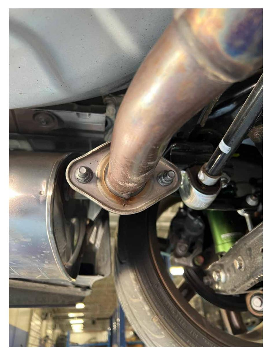
2. Remove 4 y-pipe bolts from both mufflers (14mm socket)
