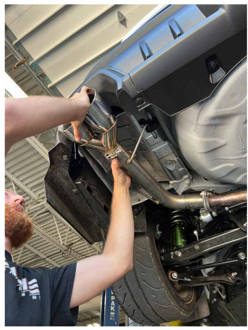
6. Install included exhaust tips, securing with included clamps
