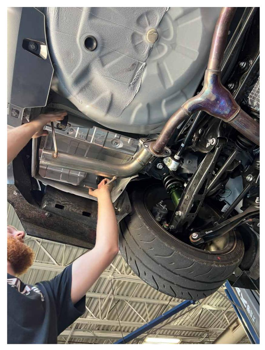
4. Ensure gasket is still in place on the y pipe ends and place MAPerformance muffler delete in place securing with factory hangers
