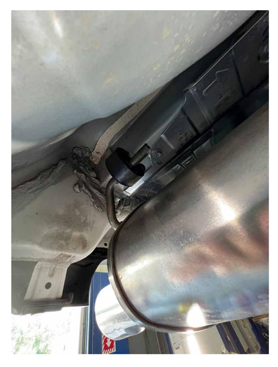
3. Remove 4 rubber hangers from both mufflers and remove mufflers
