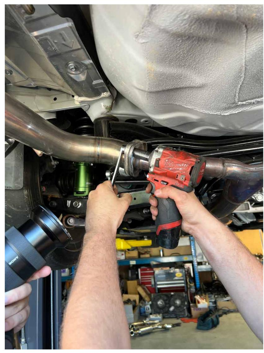
5. Secure MAP muffler delete to factory Y pipe with oem bolts you removed in step 4
