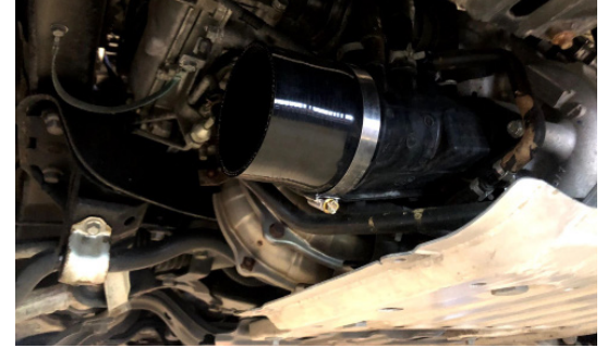
15. INSTALL COUPLER ONTO TURBO AND TIGHTEN CLAMP
