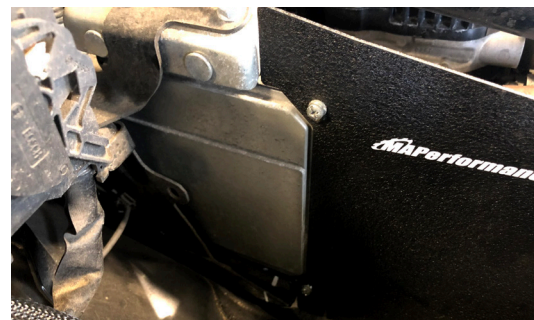
14. REMOVE 10MM (HEAD) BOLT PICTURED, INSTALL MAP INTAKE HEAT SHIELD USING PHILLIPS HEAD SCREWS AND BOLT YOU REMOVED EARLIER
