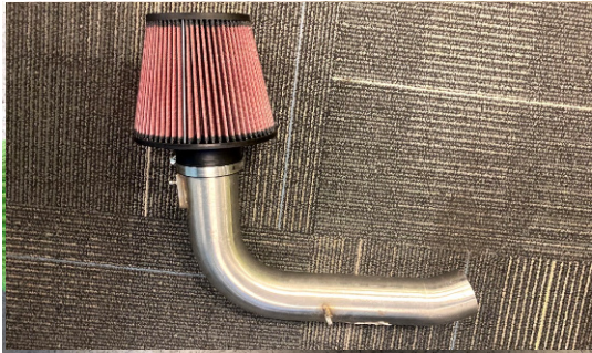
12. ASSEMBLE INTAKE. INSTALL MAF INTO NEW TUBE WITH HARDWARE AND SET TO THE SIDE
