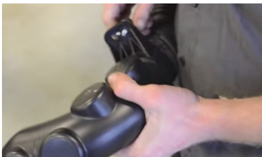
16. REMOVE STUD FROM FACTORY INTAKE
