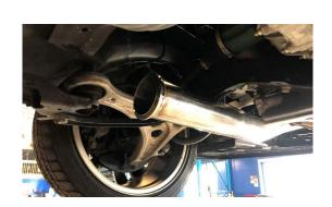
12. INSTALL LOWER BRACKET YOU REMOVED EARLIER AND THREAD THE BOLTS IN BY HAND
