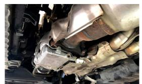
7. REMOVE 4 DOWNPIPE NUTS, USE OF EXTENSIONS AND SWIVEL SOCKETS WILL MAKE THIS MUCH EASIER (14MM NUTS) NOTE- IMPACT TOOLS, HEAT AND PENETRATING OIL WILL MAKE THIS PART MUCH EASIER AND WILL AID IN NOT SNAPPING THE STUDS, IT IS HOWEVER COMMON THAT THE ENTIRE STUD WILL PULL OUT AND NOT JUST THE NUT. THIS IS FINE
