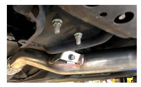
19. INSTALL GROUND STRAP W/ PROVIDED HARDWARE ONTO TAB ON DOWNPIPE
