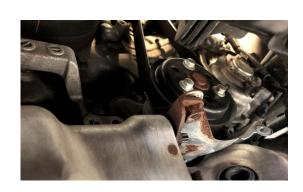
6. REMOVE FURTHEST FORWARD DOWNPIPE HEAT SHIELD
