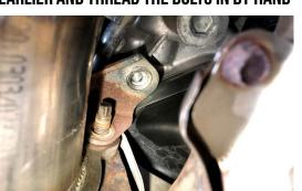
13. REINSTALL DOWNPIPE BOLTS AND STUDS
