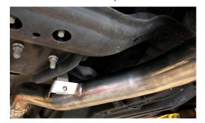
17. CONNECT BOTH ENDS TOGETHER VIA V-BAND CAMP, DO NOT FULLY TIGHTEN V-BAND CLAMP YET NOTE: IT MAY BE NEEDED TO USE AN ADAPTER TO ADAPT OUR DOWNPIPE TO THE FACTORY CATBACK -INSTALL 2 BOLT GASKET AND BOLTS INTO THE 2 BOLT FLANGE (WE HAVE OPTED TO ALSO USE A GRIMMSPEED ADAPTER) TIGHTEN THESE BOLTS AND THE V-BAND CLAMP
