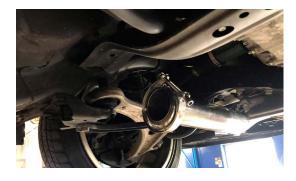
16. PLACE REAR HALF OF DOWNPIPE ONTO TRANS HANGER BRACKET, DO NOT INSTALL BOLT
