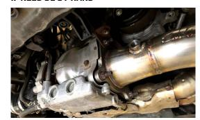
14. SNUG ALL NUTS AND BOLTS DOWN THAT YOU JUST INSTALLED BY HAND
