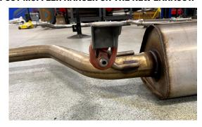
7. INSTALL THE REAR Y PIPE ONTO THE CAR
