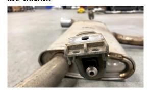
NOTE: WE INCLUDE ONE EXHAUST HANGER BECAUSE THE GTI HAS AN EXTRA UNUSED HANGER.
