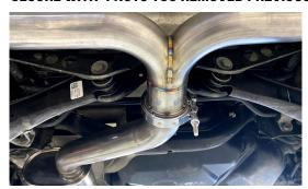
8. INSTALL THE RESONATED SECTION ONTO THE DOWNPIPE AND BE SURE THE PIPE IS CLOCKED IN THE CORRECT ORIENTATION (AS PICTURED)
