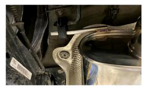
11. TIGHTEN ALL VBAND CLAMPS STARTING FROM THE DOWNPIPIE TO RESONATED CONNECTION, THEN RESONATOR TO MUFFLER SECTION, AND LASTLY MUFFLER TO
