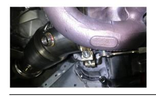
12. REINSTALL 2 BOLTS HOLDING DOWNPIPE ONTO THE BRACKET
