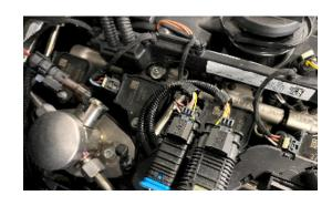
2. CONTINUED - YOU WILL NEED TO UNSECURE THE CONNECTORS FROM THEIR BRACKET. TO DO THIS USE A SMALL PICK TO MOVE THE LOCKING TAB TOWARDS THE BACK OF THE CAR AND SLIDE THE CONNECTOR TOWARDS THE VALVE COVER (TO THE RIGHT IF STANDING DIRECTING INFRONT OF THE CAR)
