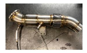
9. INSTALL THE MAP DOWNPIPE IN THE CAR BY SLIDING IT IN AND ROTATING INTO PLACE ON THE BRACKET, BE SURE TO GET THE TURBO OUTLET AND DOWNPIPE FLANGE LINED UP.
