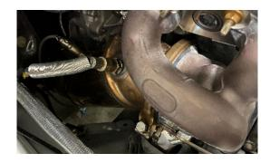
4. LOOSEN THE PINCH CLAMP (13MM) SECURING THE DOWNPIPE TO THE EXHAUST, AND REMOVE THE 13MM BOLT HOLDING THE EXHAUST TO THE FRONT EXHAUST HANGER, THIS WILL GIVE YOU ROOM TO SLIDE THE DOWNPIPE OUT OF THE EXHAUST
