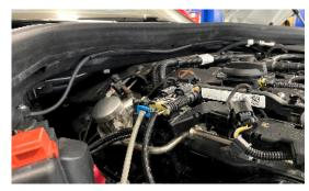
3. LOOSEN THE "VBAND" CLAMP SECURING THE THE DOWNPIPE TO THE TURBO (13MM)
