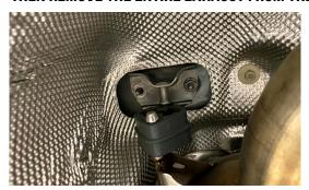
7. REMOVE THE EXHAUST HANGERS FROM THE REMOVED EXHAUST
