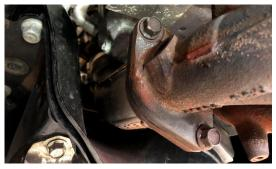
4. REMOVE 2 BOLTS SECURING FACTORY Manifold to your up-pipe 5. REMOVE 6 14MM NUTS SECURING FACTORY MANIFOLD
