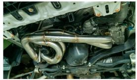
8. INSTALL 2 BOLTS SECURING MAP ELH TO THE UP PIPE
