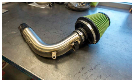
18. ASSEMBLE INTAKE WITH SUPPLIED COUPLERS AND CLAMPS
