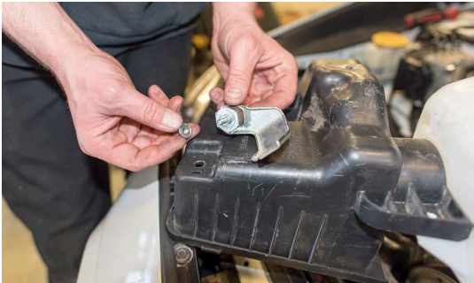
17. REINSTALL MAF SENSOR ONTO MAP INTAKE WITH SUPPLIED HARDWARE
