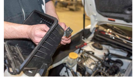
16. REMOVE MAF SENSOR FROM STOCK AIR BOX
