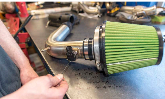
17. REINSTALL MAF SENSOR ONTO MAP INTAKE WITH SUPPLIED HARDWARE
