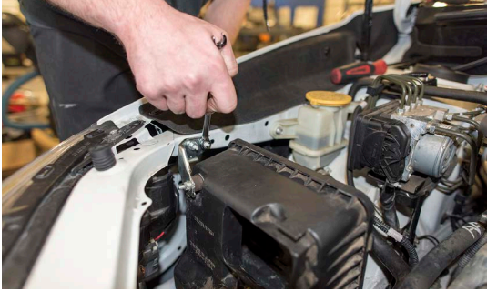
12. REMOVE TWO 10MM NUTS FROM AIR BOX BRACKET
