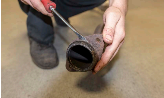
21. REMOVE STOCK DOUGHNUT GASKET CAREFULLY
