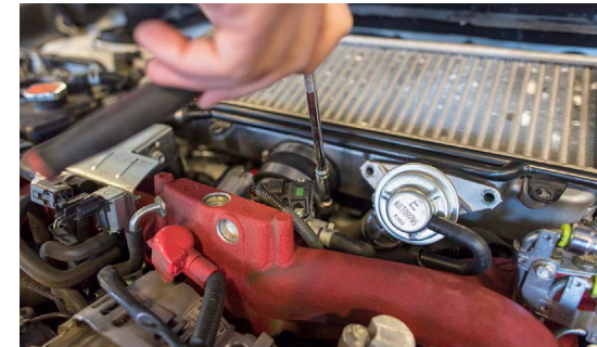
25. REINSTALL INTERCOOLER, 8MM CLAMP TO TURBO OUTLET AND THROTTLE BODY
