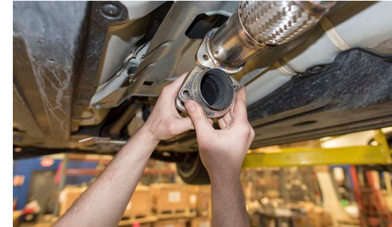
23. INSERT BETWEEN EXHAUST AND MAP DOWNPIPE
