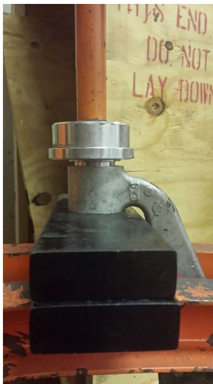
Make sure the bushing goes in straight.
