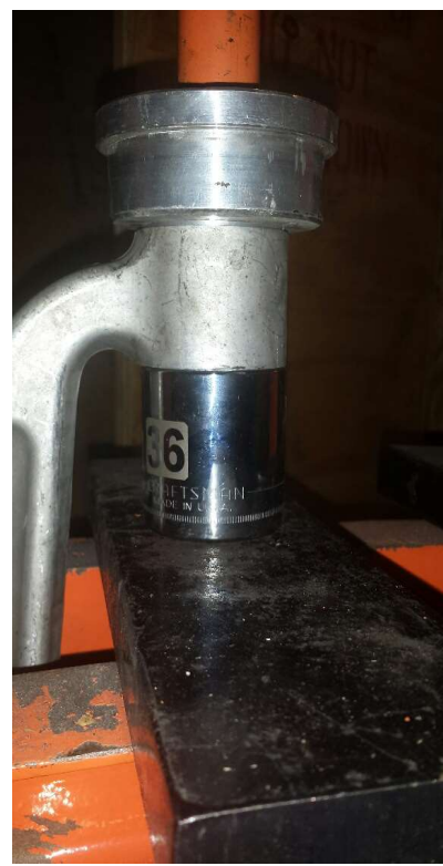
SPL diff bushing driver on top, 36mm socket as receiver on bottom.
