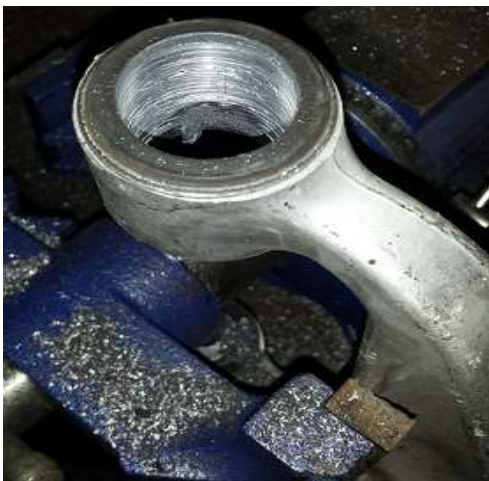
Sleeve ready to be cut.
