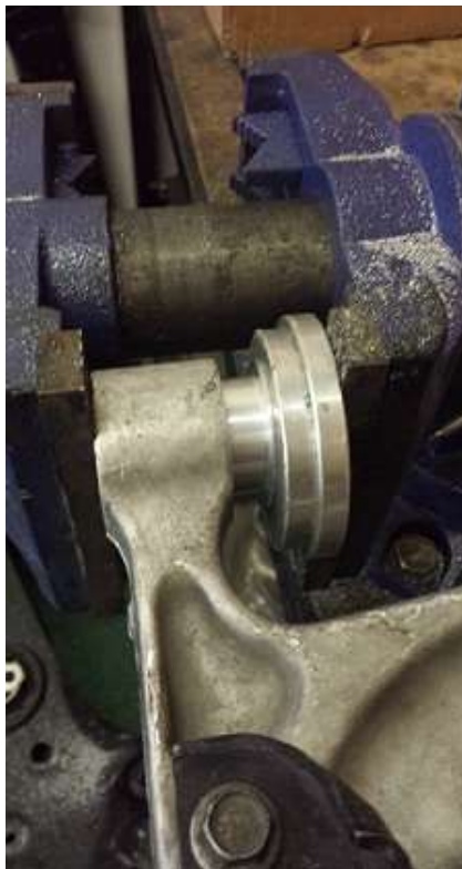
A large vice can be used if you don't have a press.
