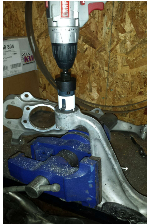
Proper alignment of hole saw.
