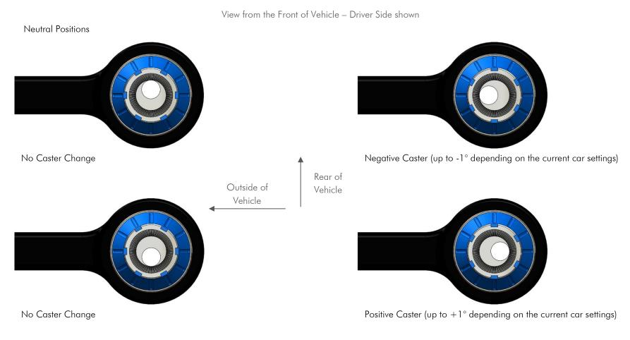
Figure 03 - View from the Front of Vehicle, Driver Side shown
