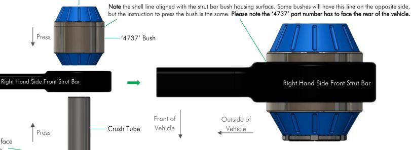
Figure 02 – '4737' bushing installation
