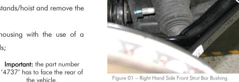
Note the shell line aligned with the strut bar bush housing surface. Some bushes will have this line on the opposite side,
