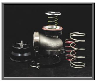
4. Orient the wastegate can top to the desired position and compress the wastegate can top until it is seated with the wastegate can bottom. Use of a press or vice may be necessary depending on spring selection. With the v-band flanges properly aligned, install the v-band clamp. If you need to re-align the upper can, relieve tension on top, rotate and recompress. Once aligned properly, tighten the clamp screw to 51-55 inch lbs or 5 ft lbs. (5.8-6.2 Newton Meters)
