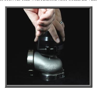
2. WARNING! THE WASTEGATE CAN TOP IS UNDER HIGH SPRING TENSION. USE SAFETY GOGGLES AND REMOVE WITH CARE. Using a 4mm hex key, loosen and remove the wastegate v-band clamp. The use of a press or vise may be used to hold down the wastegate can top while loosening the clamp. If using a press or vise for disassembly, use a cloth or micro fiber rag to protect the surface finish from scratches. Remove the clamp and cap slowly, using care to secure the spring top plate and spring/springs upon removal.
