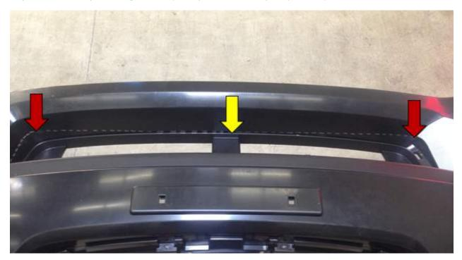
3. Now from the bottom of the bumper looking up, draw/mark/tape a straight line from where the center brace in the bumper opening meets the bumper to the points marked in step one as well (red arrows.)
