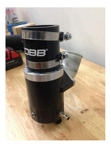
2. Next, Slip the BPV nose into the BPV return hose. Tighten the hose clamp using an 8MM socket or nut driver.
