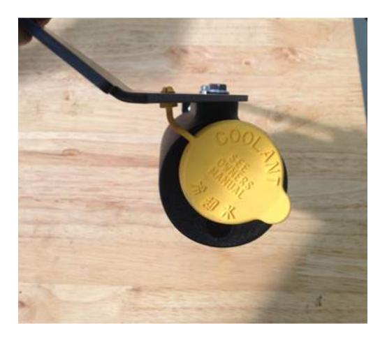
4. Remove the reservoir cap from the factory overflow tank and install it on the new tank.
