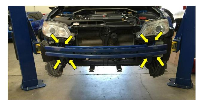
5. Now remove the two lower bumper cover braces from the bottom of the core support with a 12mm socket and ratchet.
