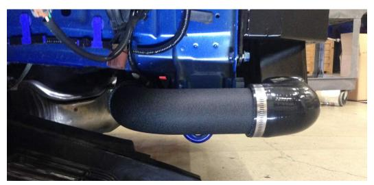
4. It's now time to trim the inner fender liner. With the pipe in place, hold the fender liner into position to see where it needs to be trimmed. This can be done with a variety of tools. We had best luck with an air saw, but a rotary tool, sheet metal snips or side cutting pliers can be used. Be sure to wear appropriate eye protection. Here is an example of the passenger side of our car once completed.
