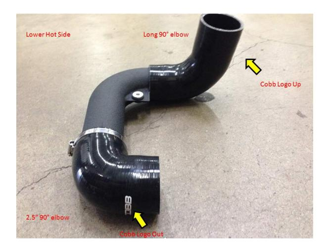
2. Slip the 2.5" 90° end of the pipe over the passenger side core outlet. Place the clamps over each end of the silicone before installation. Only loosely tighten as the fitment may need to be adjusted. The bracket with the bushing/grommet assembly should be on top of the square hole core support. Place the bolt through the top of the bushing->fender liner core support washer then tighten with an M6 flange nut with a 10MM socket and ratchet.
