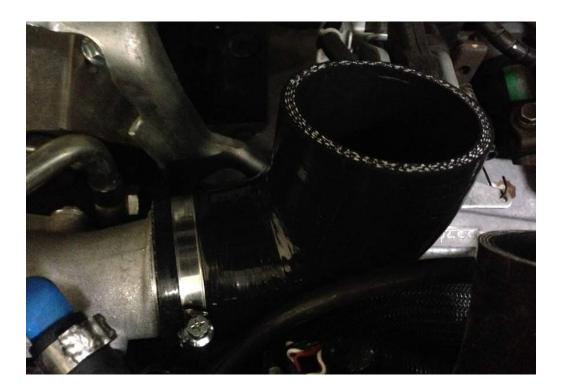
4. Now slide a 2.5" coupler over the straight end of the hot pipe. Add a clamp on the 90° end of the hot pipe and install it on the vehicle as shown below.
