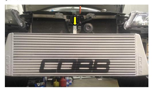
3. Install the front bumper braces on the bottom of the intercooler. Do this by holding the front bumper braces in position and hand tightening the supplied M6x25mm flange bolts to capture both the bottom intercooler bracket as well as the front bumper brace. Leave the bolts a little loose to tighten later.
