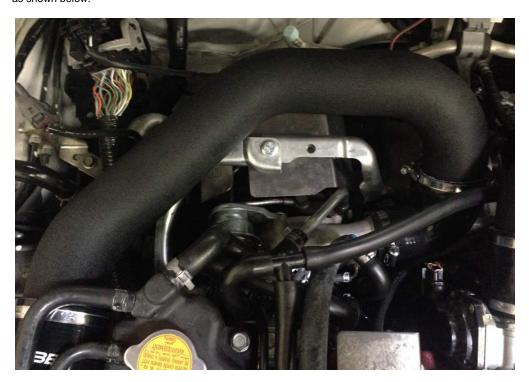
5. Next, slide clamps over the straight silicone coupler and the long 90° coupler Install the mid hot pipe. The long end of the mid hot pipe will attach to the lower hot pipe; the short end will attach to the upper hot pipe. Check for clearance between the front of the engine, the chassis, and the radiator fan assembly. Tighten all the clamps with an 8mm wrench or socket once you've determined you like how it is fitting.
