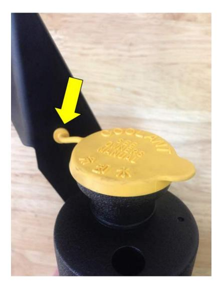
5. To install the tank in the car, place the bottom bung of the bracket into the mounting hole on the radiator shroud. Bolt the top of the bracket to the radiator using the provided M6x25 flange head bolt. Make sure to install the 1/4"x3/4" spacer between the bracket and radiator. Tighten the bolt with a 10mm socket or wrench.
