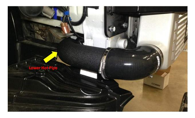
TIP: Due to limited clearance when tightening the clamp on the lower portion of the mid hot pipe it may be necessary to mark the tube when in place, pull from the vehicle, install the long silicone 90° on the mid hot pipe and reinstall it into the vehicle in that order.
