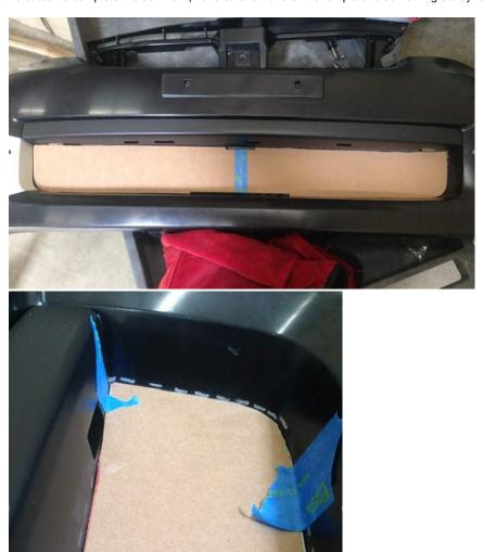
5. After double checking all measurements, use the method most comfortable (air saw, utility knife, cutoff wheel, etc.) to you to cut the bumper along the cut line.
