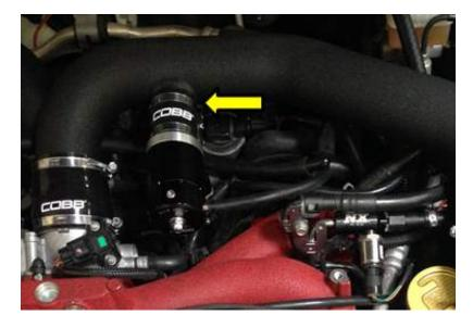
4. Reattach the vacuum line to the barbed fitting on the BPV body.
