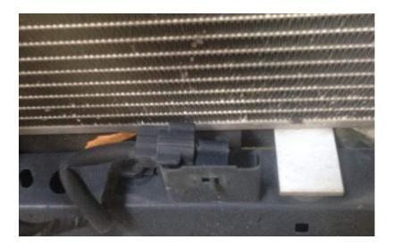
3. Remove the two foam pads from the sides of the core support with a plastic clip removal tool.
