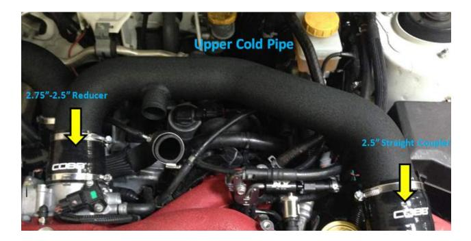
4. Next, slide clamps over the straight silicone coupler and the long 90° coupler. Install the mid cold pipe. Check for clearance between the front of the engine, the chassis, and the radiator fan assembly. Tighten all the clamps with an 8mm wrench or socket when you like how it is fitting.
