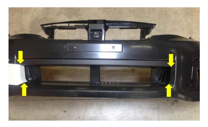
2. Looking downward at the bumper from the top side, draw/mark/tape a straight line from the edge of where the painted portion of the bumper meets the black plastic area(yellow arrow) to the points marked in step one (red arrows).
