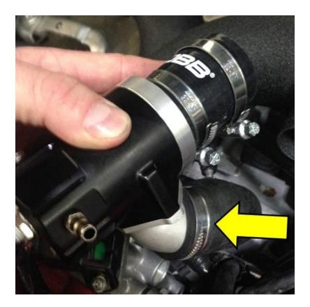
3. Now slip the silicone BPV coupler onto the BPV outlet on the upper cold pipe.
