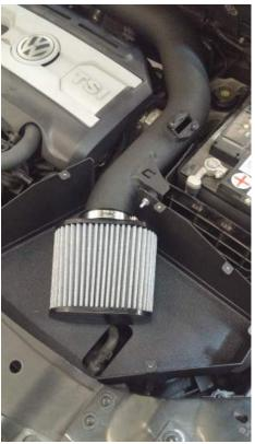
9. Using six M4 button head screws and six 4mm nylon washers, fasten the lid to the airbox. Use the provided 2.5mm hex key to do so.
