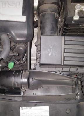
9. Now pull the remainder of the tube out of the side of the airbox. Make sure the tube is unclipped, it should just wiggle out.
