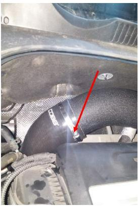
4. To get the open ends of the spacers through the corresponding slots on the airbox, pull the back wall of the airbox inward to allow the intake tube to slide down to the slots. Once the spacers are through the slots, place 6mm serrated nuts on the end.
