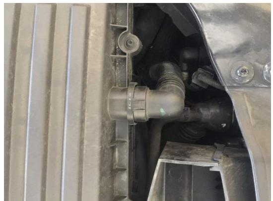
11. Using a 5mm hex key to loosen the mounting screw.
