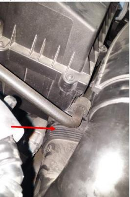
10. For a CBFA car, unclip the air pump hose from the stock airbox.
