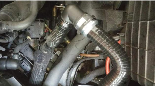
8. Now place the custom COBB filter on the open end of the intake pipe and tighten the worm clamp around it using an 8mm socket or flathead screwdriver. NOTE: Make sure the filter sits parallel to the bottom of the airbox and is sitting as low as possible for correct fitment.
