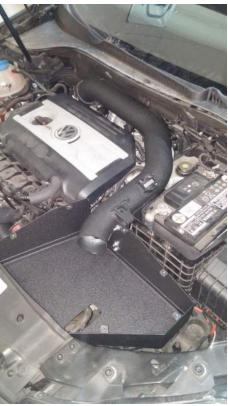
7. Now place the custom COBB filter on the open end of the intake pipe and tighten the worm clamp around it using an 8mm socket or flathead screwdriver. NOTE: Make sure the filter sits parallel to the bottom of the airbox and is sitting as low as possible for correct fitment.
