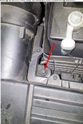
12. Remove the front two mounting screws using a T25 torx screwdriver or socket. NOTE: Keep these stock screws for the installation of the COBB Intake.
