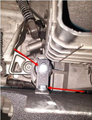
3. Tighten all above steps! Make sure that the slot on the bracket is in line with the slot on the airbox.
