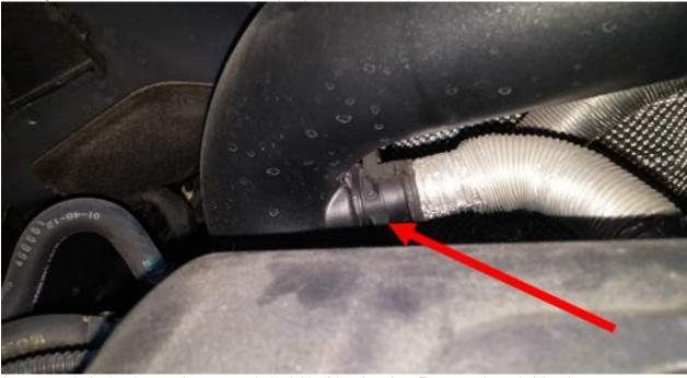
4. Now unscrew the intake tube mounting screw on the backside of the tube using a T30 torx socket and 3/8" ratchet.
