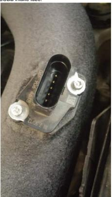
12. Plug the MAF sensor into the MAF housing.13. Check to make sure all nuts and bolts are tight along with ensuring no steps were skipped. Enjoy your COBB Tuning Volkswagen MK6 Intake!
