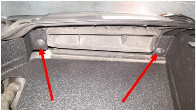
2. Place one M6 x 12 flange bolt through the bottom hole on the COBB airbox bracket and then through the bottom hole on the back side of the airbox as shown. Place a 6mm serrated nut on the end of the bolt and loosely thread on. Then place another M6 x 12 bolt through the slotted section of the bracket into the mounting bung.
