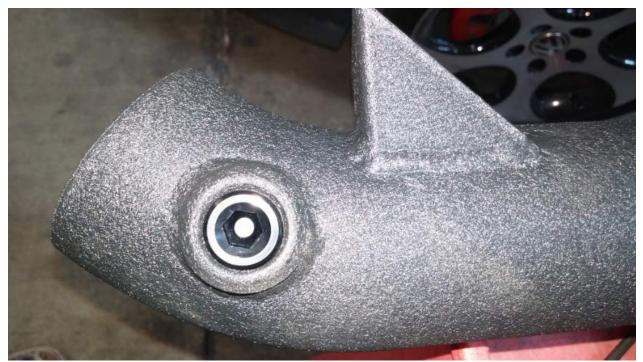
2. Attach the silicone adapter to the opposite end of the intake tube. Use a 7mm socket or flathead screwdriver to tighten the 3"-3.5" worm clamp that fastens the silicone to the tube. Loosely place the 2.5"-2.75" worm clamp around the smaller end of the silicone.
