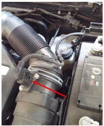
3. Remove the stock intake tube by first unplugging the the PCV. This may be easier if you pry one side of the tab over the lip of the PCV bung with a flathead screwdriver. NOTE: This step may be easier after step 5.
