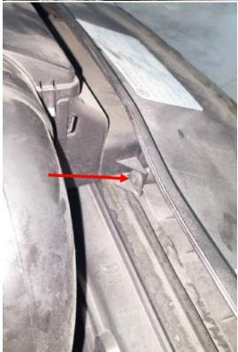
13. With the 5mm hex mounting screw completely loosened and the front two screws removed, pull the stock airbox out of the car. The airbox is held down by ball sockets and grommets so you will need to pull hard enough to pop the ball sockets out of place. There is also a drain hose that will pull out of the car with the airbox, you do not need to disconnect it!
