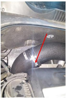
5. To get the open ends of the spacers through the corresponding slots on the airbox, pull the back wall of the airbox inward to allow the intake tube to slide down to the slots. Once the spacers are through the slots, place 6mm serrated nuts on the end.
