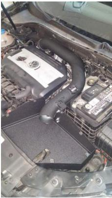
6. Take the 90° hose and install the air pump adapter to the longer end. Reach up from underneath the airbox, through the hole cutout, and to the 1/2" NPT hose barb with the open end of the 90° hose. Push the barbed end through the hose to connect the hose to the intake tube.
