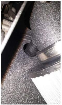
7. Now attach the air pump adapter to the air pump. This should just click right over the adapter. NOTE: The picture shown is for clarity reasons only (airbox not shown).
