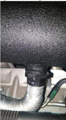
10. Remove the stock MAF housing using a T20 security torx drive. Using the same screws and MAF housing, correctly install onto the COBB intake tube.
