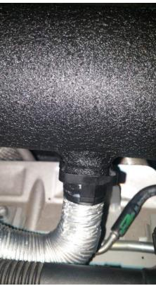
11. Remove the stock MAF housing using a T20 security torx drive. Using the same screws and MAF housing, correctly install onto the COBB intake tube.
