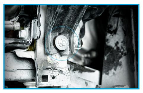
21. Remove the (1) 10mm from the upper bracket at the top of the resonator. After these are removed the resonator will come free. It is easier to remove the hose on the charge pipe by pulling on the whole resonator assembly.
