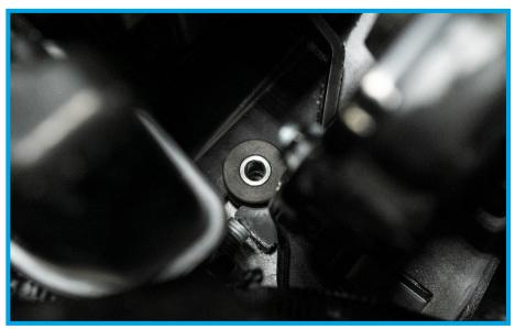
16. Remove the top resonator from the side of the curved hose that faces away from the airbox towards the front of the car. Simply wiggle and pull it to free it from the hose. This is where the PRL Billet 30mm plug will be placed.
