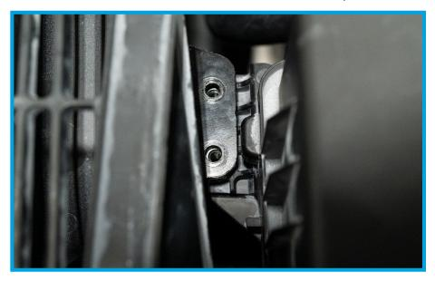
15. Using a 12" extension remove the (1) 10mm bolt on the right side of the airbox. We advise using a magnetic socket/magnetic pick so to not drop the bolt into the engine bay. Lift the airbox out of the engine bay.
