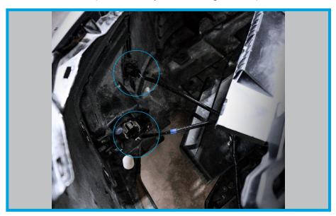
12. Pull outwards, and down to clear the headlights and then place the bumper on a flat, covered surface to avoid scratching the underside of the bumper.
