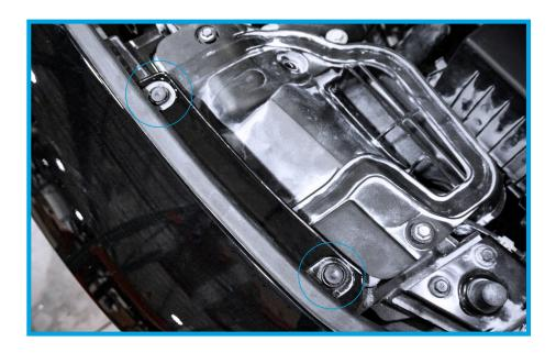
7. Remove the (1) Phillips head screw inside each of the wheel well arches. This holds the bumper to the fender liners. Check your hardware for any type of corrosion during this time as an extra step in vehicle maintenance.
