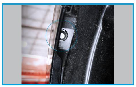
9. On the underside remove (10) bumper clips along the front section. They are circled in blue in the image below. There are (2) 10mm bolts per side that need to be removed. They are circled in white in the image below.
