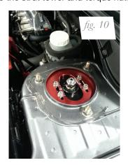
3. Reinstall the lower mount bolts through the strut mount connection (figs. 11 & 12). Torque to 167 Nm (123 ft-lbs.).
