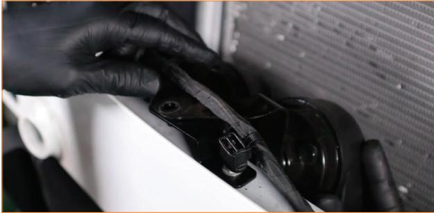
30. Remove the two pop-clips that secure the air diverter to the ducting. (2x pop-clips)
