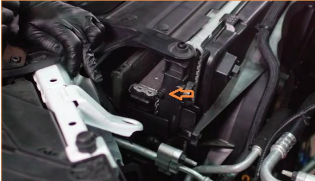
43. Locate the hose in your kit with two straight fittings. Pass one end of this hose through the ducting on the side of the radiator.
