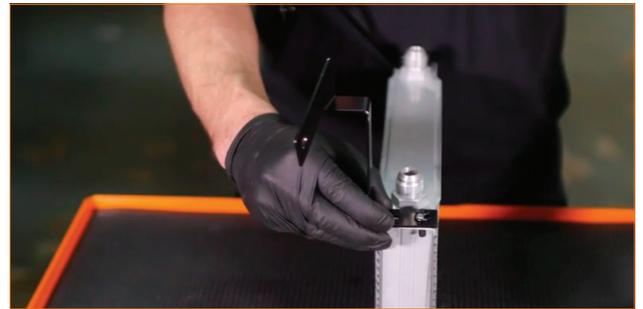
34. Locate the last bracket in your kit. Attach this bracket to the forward-most hole on the bottom of the driver side of the cooler with the provided hardware. Thread the bolt in, but do not fully tighten it. (1x 10mm bolt, 1x Nyloc nut)
