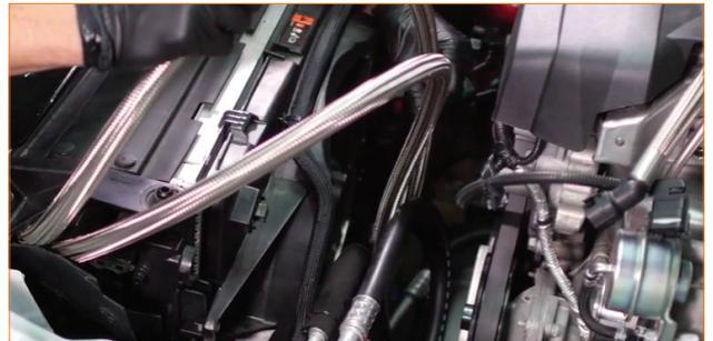
48. Locate the silicone sleeve in your kit. Slip the sleeve over the stabilizer bar where the oil lines cross under it, and secure the sleeve with the short zip ties included with your kit.
