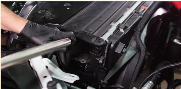
44. Locate the hose in your kit with a 45° fitting. Pass the end with the 45° fitting alongside the first hose.
