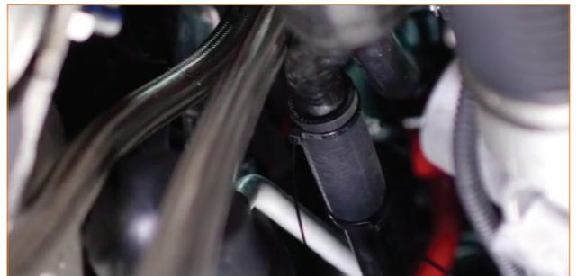
49. Lead the oil lines over the steering rack, back to the sandwich plate. Attach the lines to the fittings on the sandwich plate, and tighten them completely.
