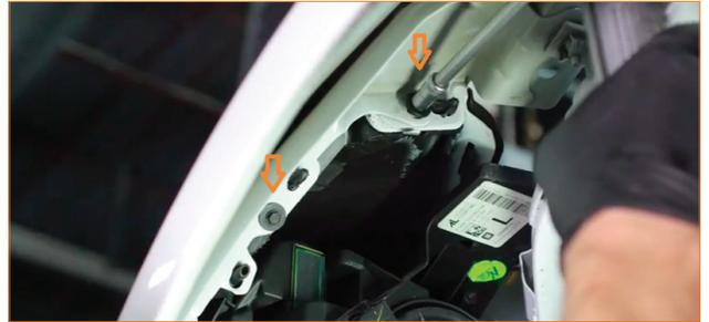
15. Remove the two screws that secure the bumper to the fender, and loosen the inner screw. (3x 7mm screws)
