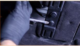
03. Remove the eight Torx screws and two pop-clips that secure the undertray to the bottom of the vehicle. Slide the undertray forward and remove it from the vehicle. (8x T30 Torx screws, 2x pop-clips)
