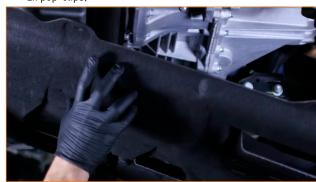
04. Remove the seven Torx screws that secure the rear edge of the splash panel to the vehicle. (7x T30 Torx screws)
