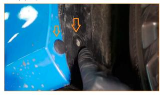
**06.** Remove the seven Phillips pop-clips that secure the front edge of the splash panel to the bumper. (7x Phillips pop-clips)
