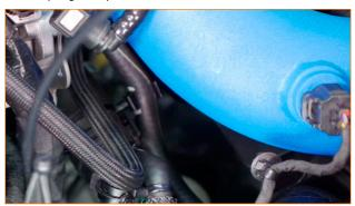
16. Compress the clamp that secures the upper radiator hose to the radiator, and then separate the hose from the radiator. [1x spring-clamp]
