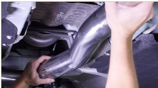
09. Slide a clamp over the mid pipe. Then install the rear pipe, which has a hanger welded to it, over the open end of the mid pipe. (1x exhaust band clamp)
