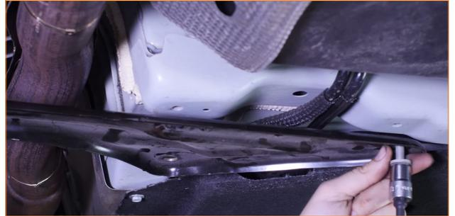
02. Remove the two nuts from the flange that attaches to the downpipe. (2x 15mm nuts)
