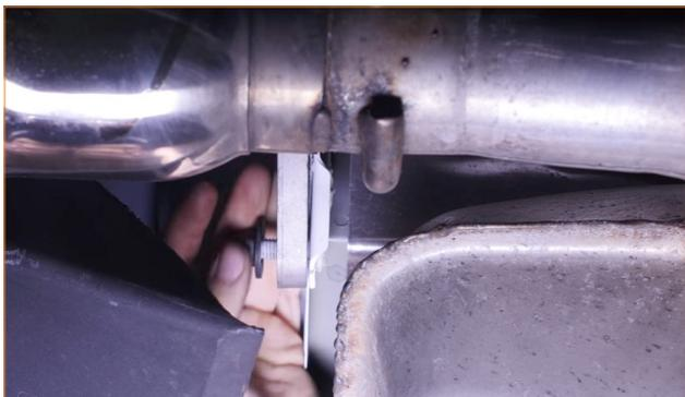
05. Lower the exhaust system from the vehicle. The exhaust system is long and awkwardly shaped, so it's best to have someone else on hand to help with its removal.
