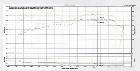
Figure 7: Stock intake vs. Mishimoto intake after the vehicle was driven for 200 miles and the ECU was fully adjusted.
