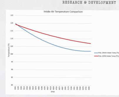
Figure 8: Comparison of stock and Mishimoto intake air temperatures
