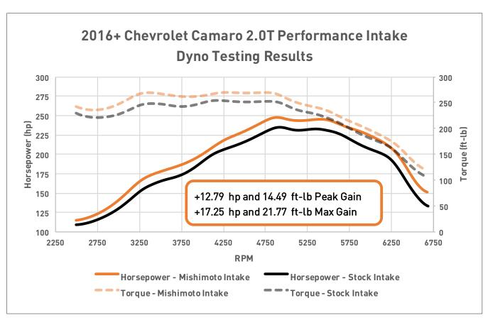
FIGURE 5: Dyno results (horsepower and torque)
