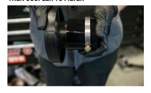
14. CONNECT AIR FILTER TO CHARGE PIPE AND TIGHTEN
