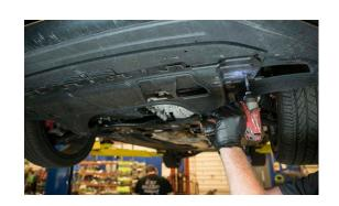
16. DISCONNECT AND REMOVE SECONDARY AIR PUMP HOSE
