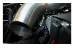
13. INSTALL COUPLER TO VELOCITY STACK THEN COUPLER TO FILTER
