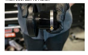
14. CONNECT VELOCITY STACK TO CHARGE PIPE AND TIGHTEN
