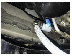
7. Attach tail end of long transparent braided tube from catch can to straight ¼" NPT fitting barb on drain valve. Lock in place using spring clamp.
