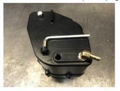
2. Clean threads of remaining sealant and install 90\* ¼" NPT fitting into base using preferred sealant. Use alignment notch to set fitting trajectory. (Early catch cans did not
