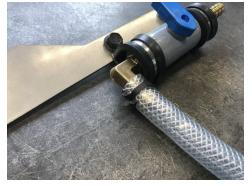
6. Mount bracket and drain assembly to lower core support aligning horizontally with the ground. Use 8x1.25 bolt and spacer in singular corresponding threaded hole to mount.
