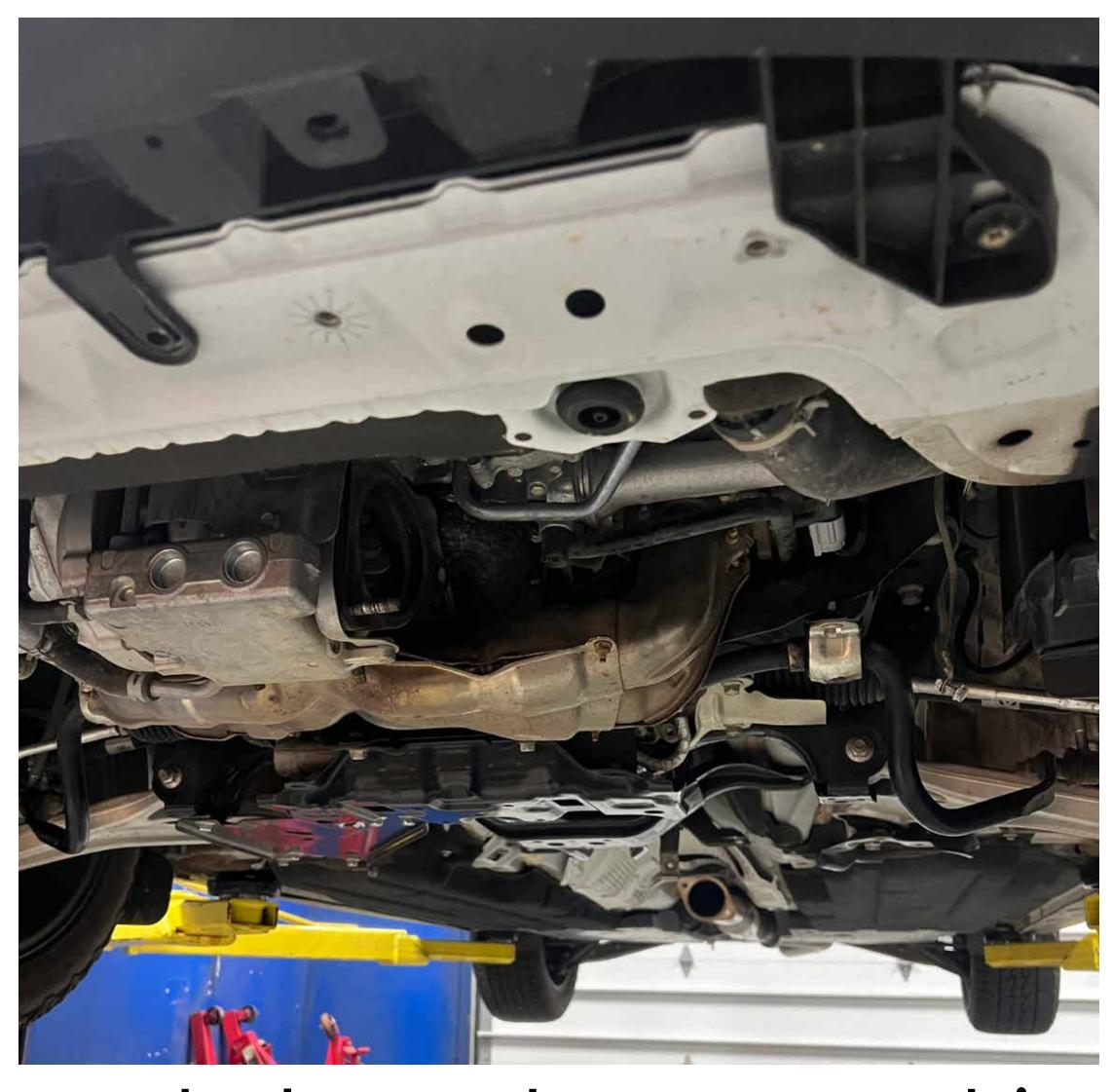
Remove bolts and nuts attaching the downpipe to catback and turbo and remove entire downpipe
