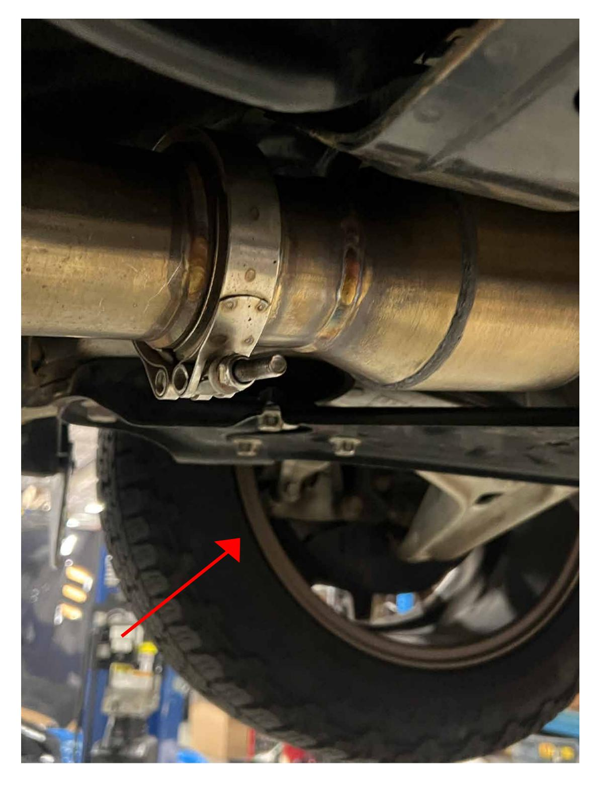
Install rear section of downpipe to the front with vband clamp and attach to catback exhaust (if using factory exhaust, use included adapter to adapt donut gasket to downpipe)
