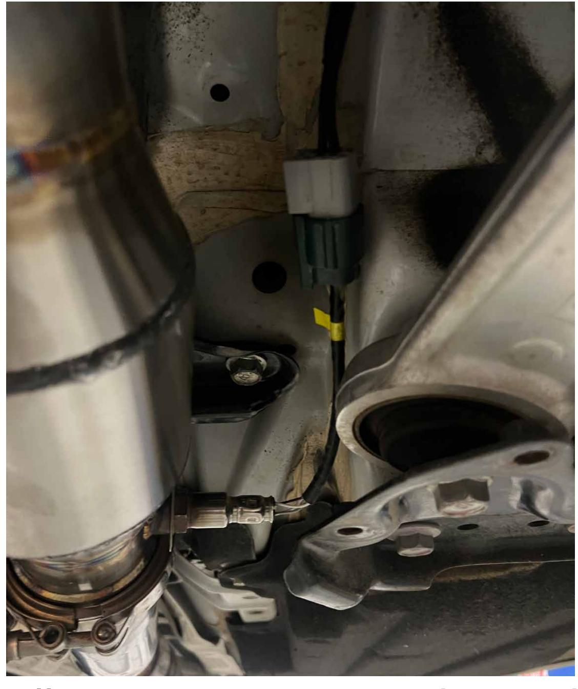
Install rear 02 sensor and attach to extension harness
