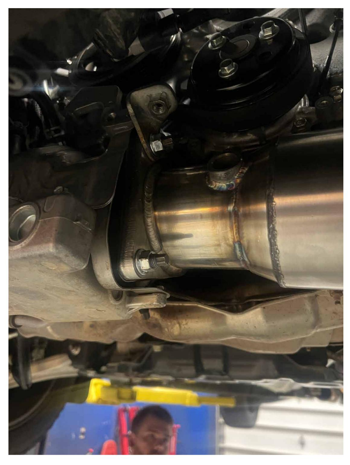
Install map downpipe onto the turbo outlet and reinstall removed nuts and bracket
