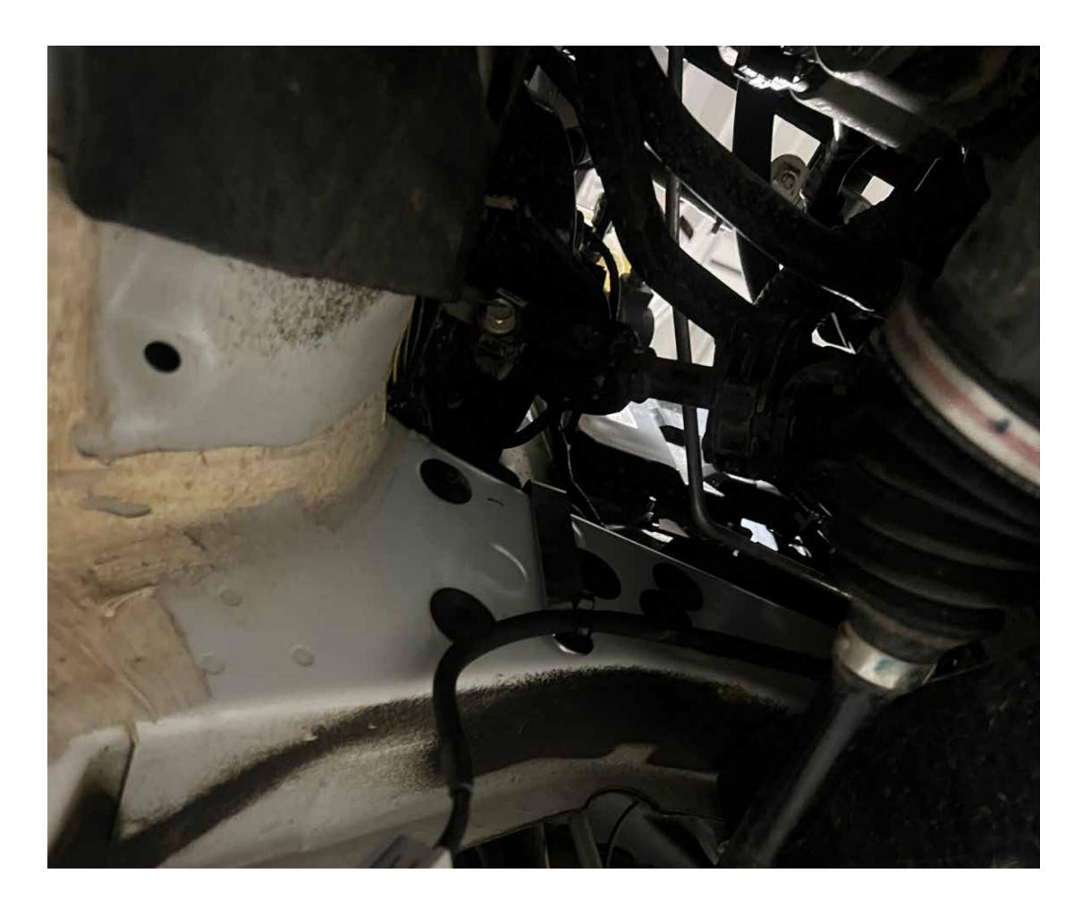
Install rear 02 sensor harness bracket and extension harness, it attaches to the factory engine harness under the brake booster
