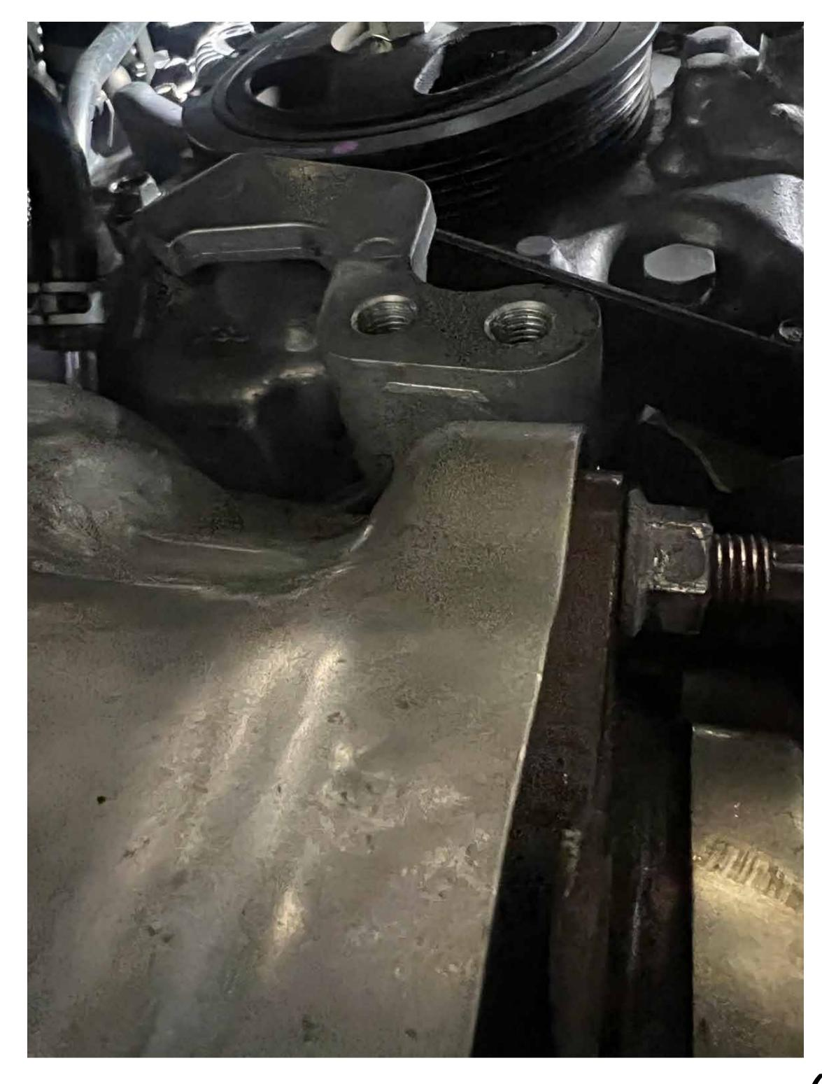
Remove turbo support brackets (you will only be able to physically remove 1 half of it until the rest of the oem downpipe comes out)
