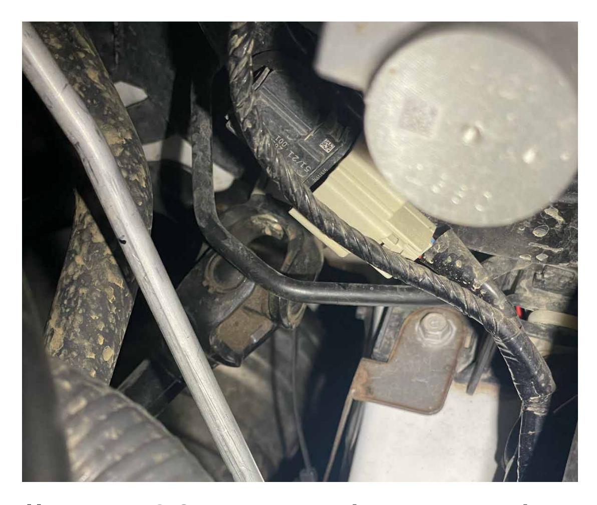
Install rear 02 sensor harness bracket and extension harness, it attaches to the factory engine harness under the brake booster
