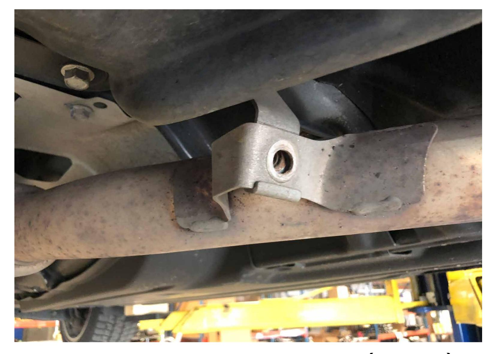
Remove trans bracket bolt (14mm)
