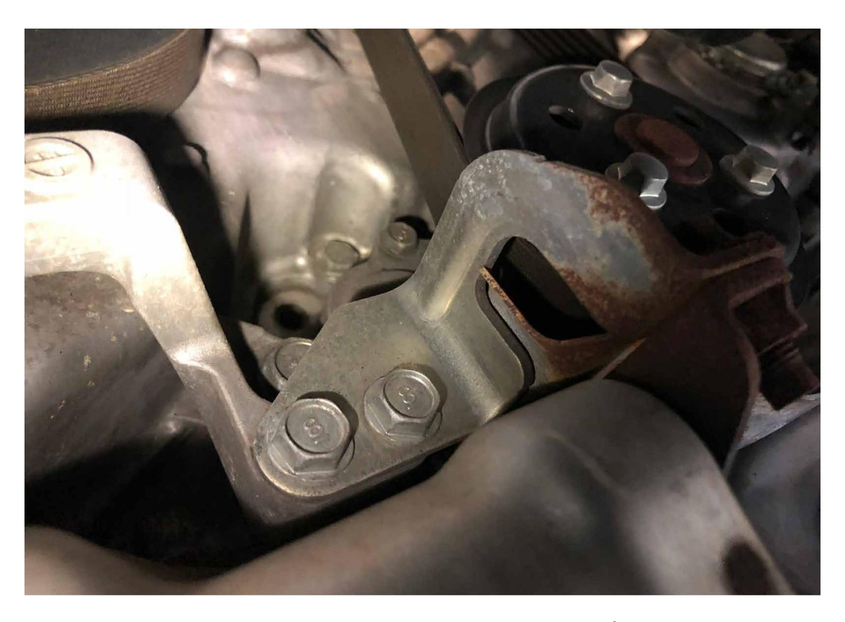
Remove bracket and heatshield under water pump as pictured (3 12mm and 2 14mm)
