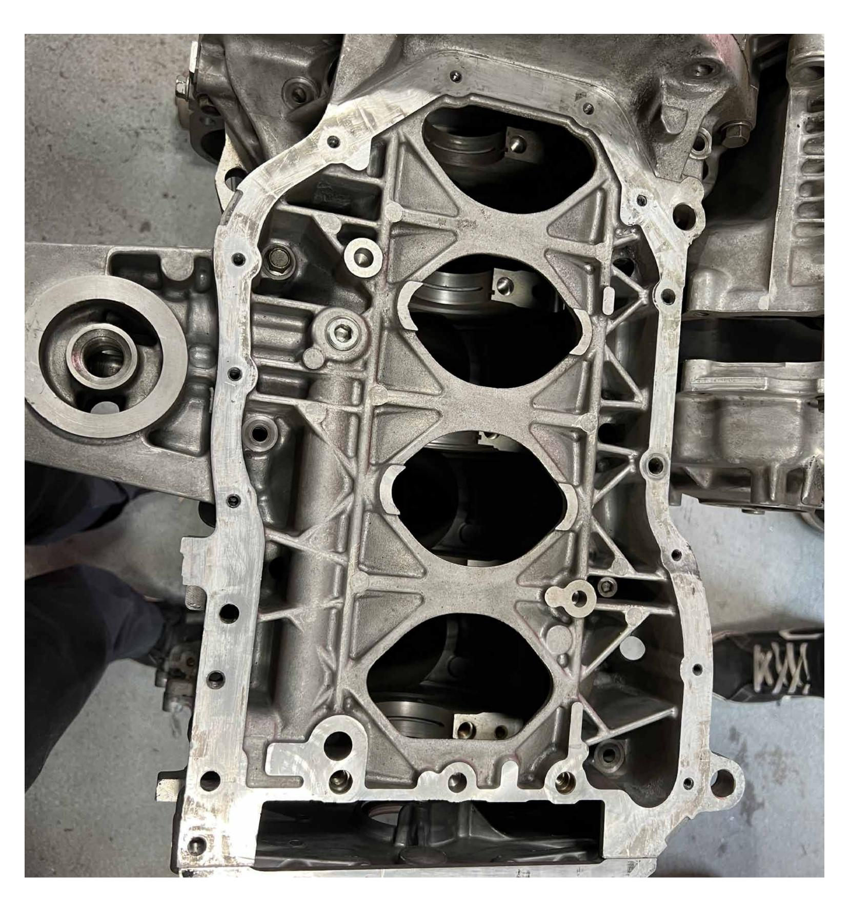
Remove oil pan, some prying may required to remove oil pan
