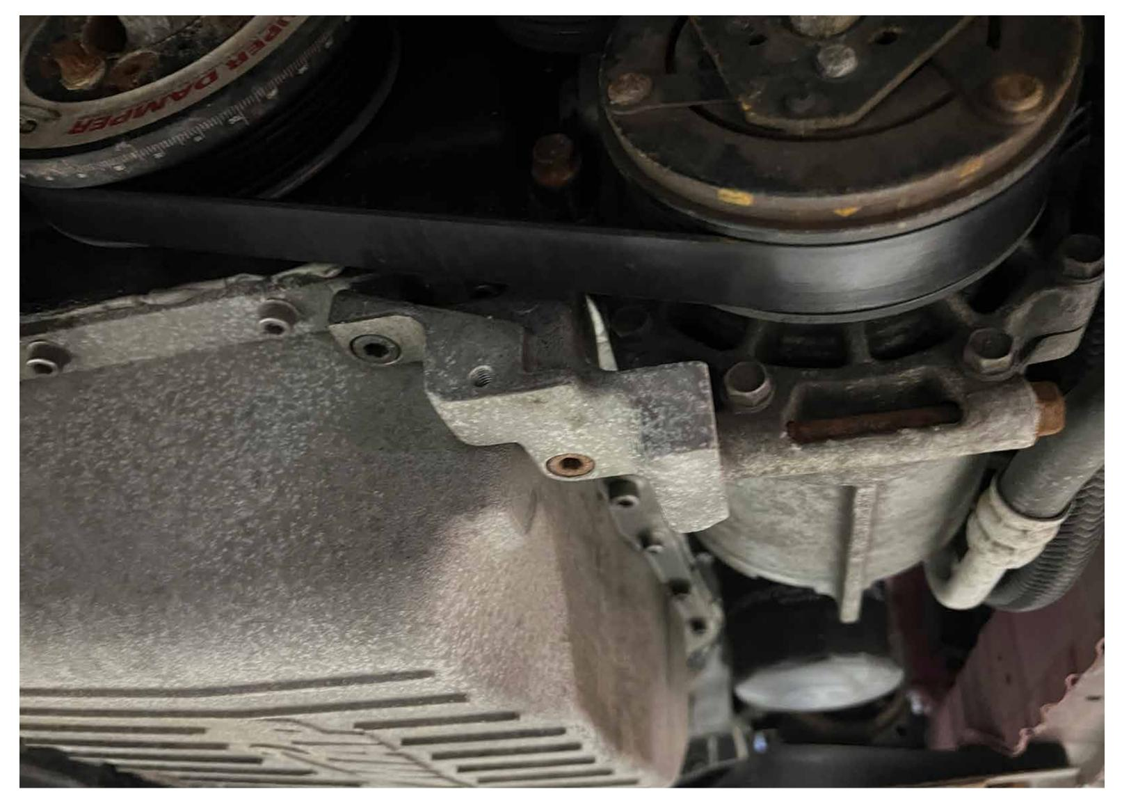
Install MAPerformance EVO x oil pan AC compressor bracket, install all bolts hand tight, and then tighten ac compressor bolts then oil pan bolts
