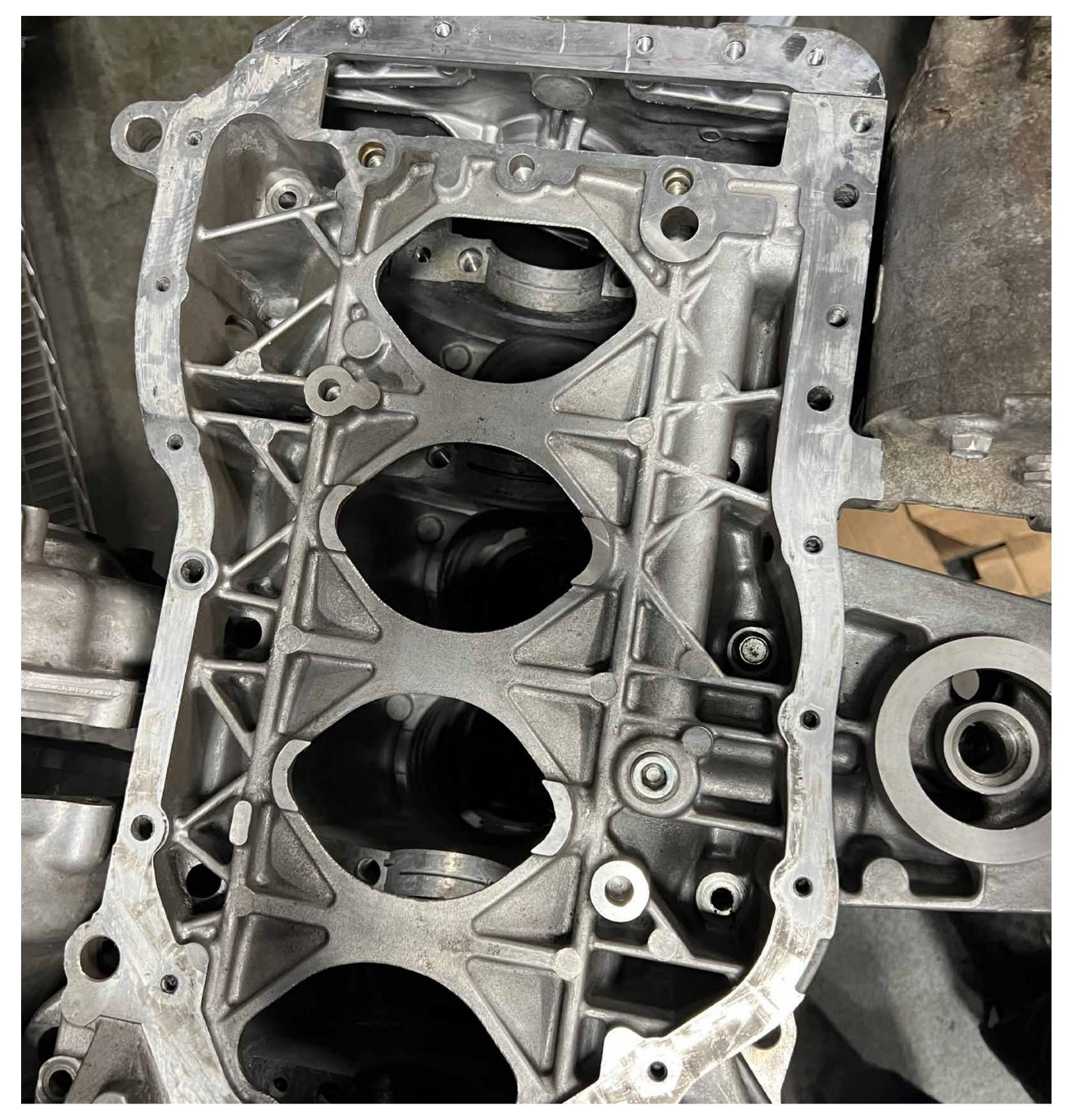
Clean gasket surface on oil pan, using gasket scraper or new razor blade at 90\* angle
