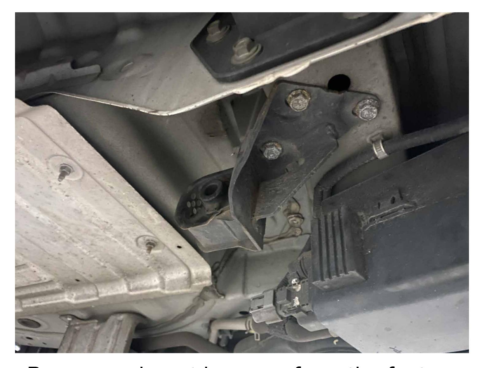
Remove exhaust hangers from the factory muffler and reinstall onto the vehicle
