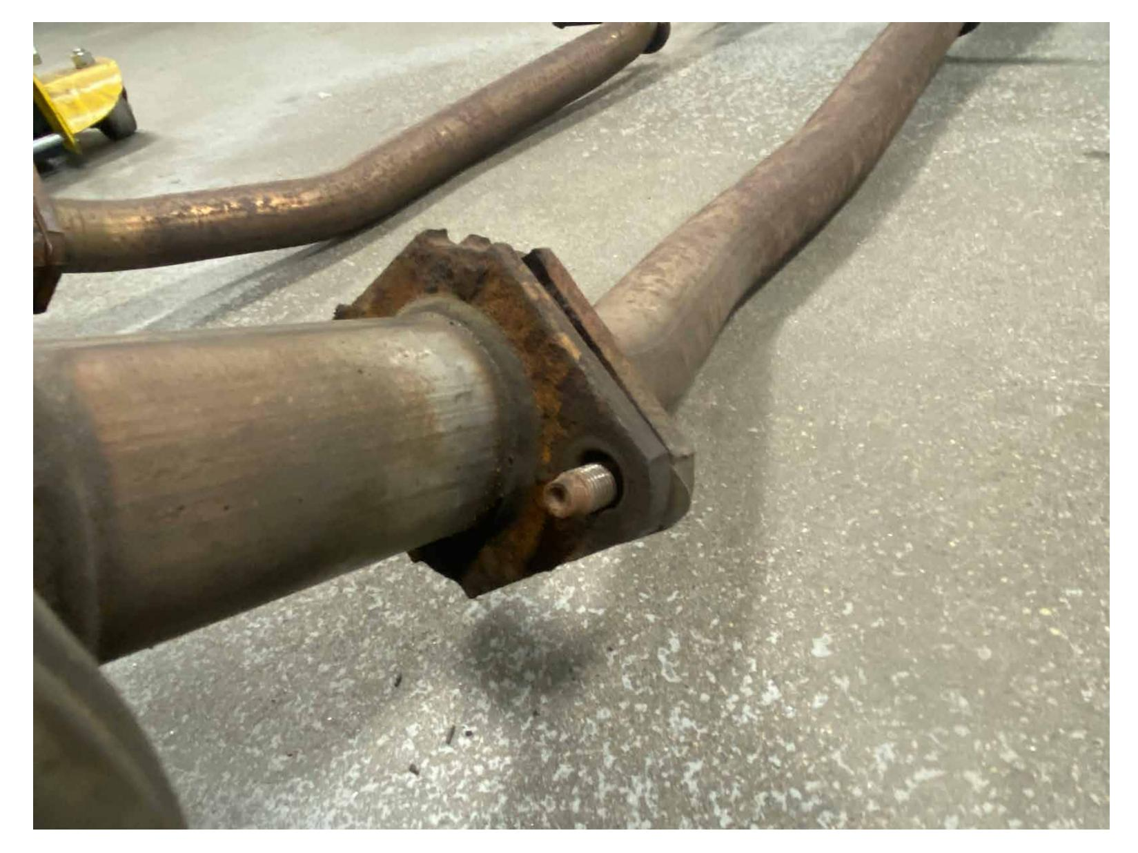
Remove 4 14mm nuts securing the factory muffler to the factory exhaust
