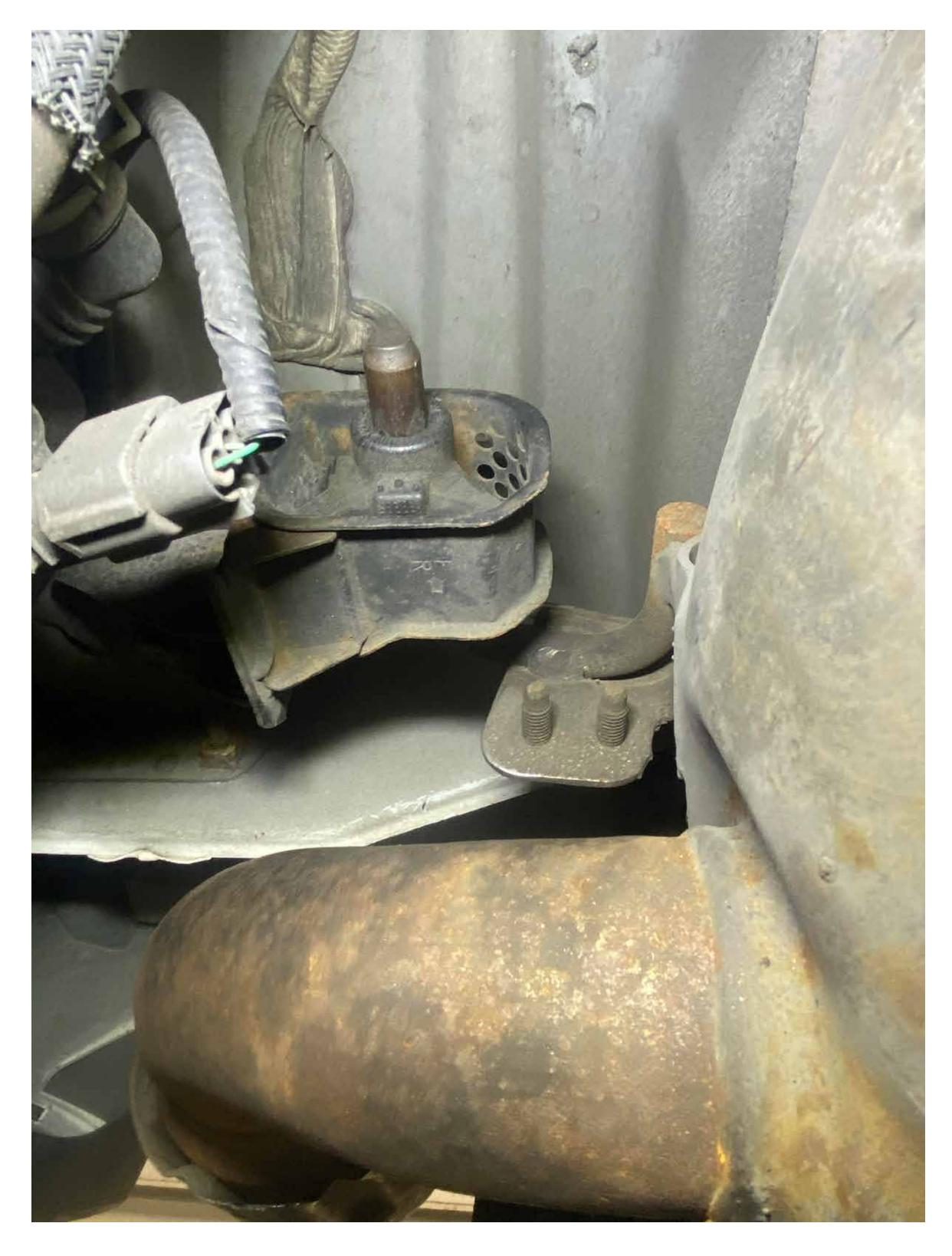
Remove 6 12mm bolts holding exhaust hanger to the vehicle
