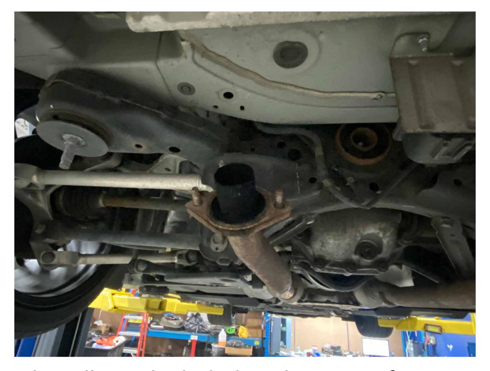
Install new included gaskets onto factory exhaust, then slide MAP Q60 Rear Muffler deletes into place
