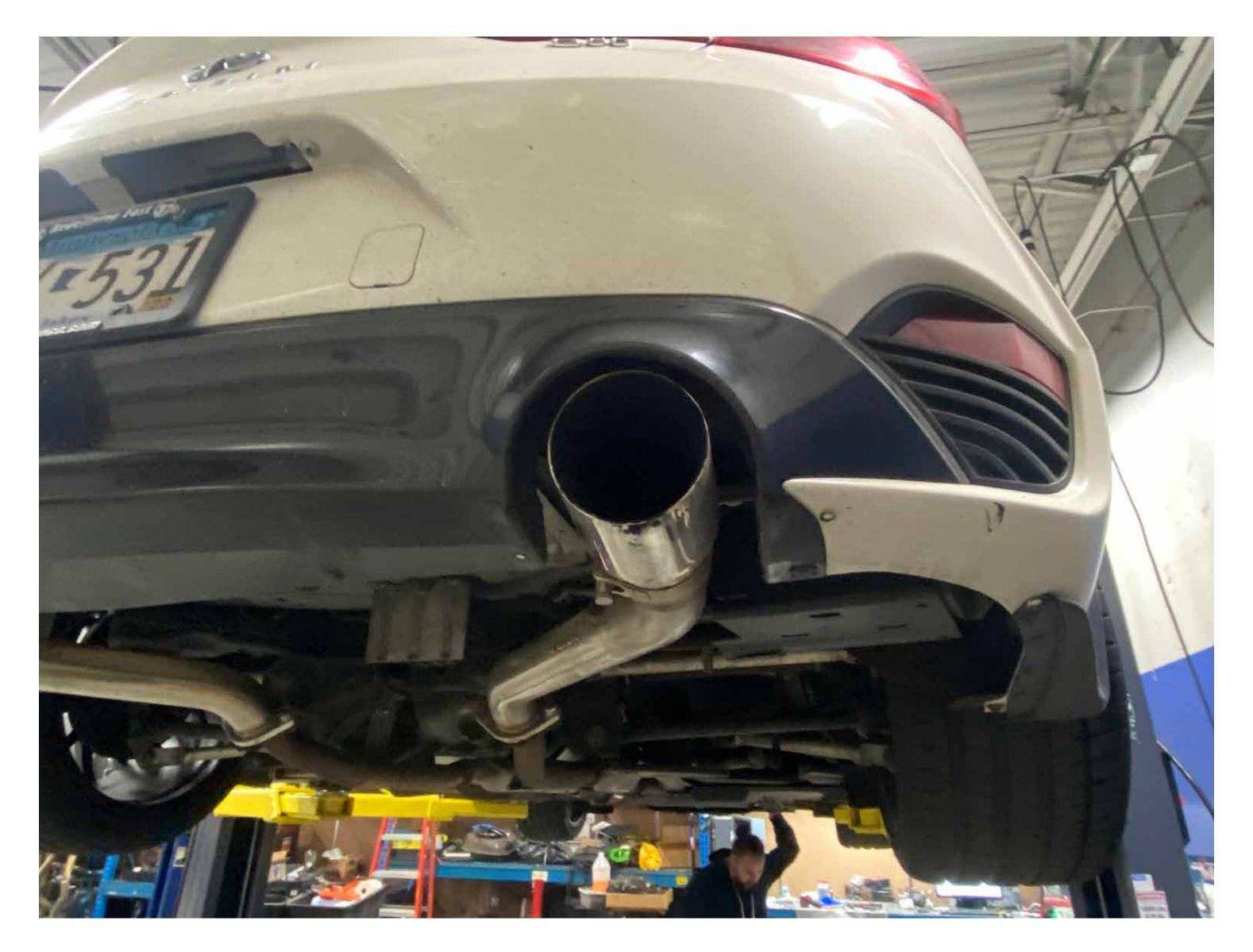
Install included tips and secure with included clamps. Be sure to use a dab of anti seize on the clamp threads to prevent galling
