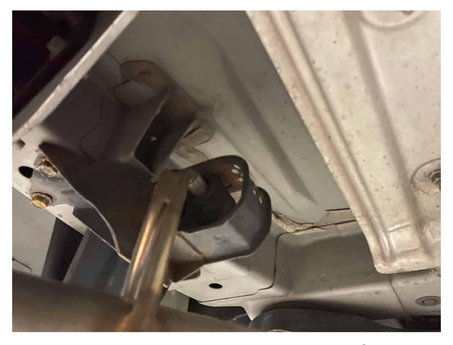
Install new included gaskets onto factory exhaust, then slide MAP Q60 Rear Muffler deletes into place
