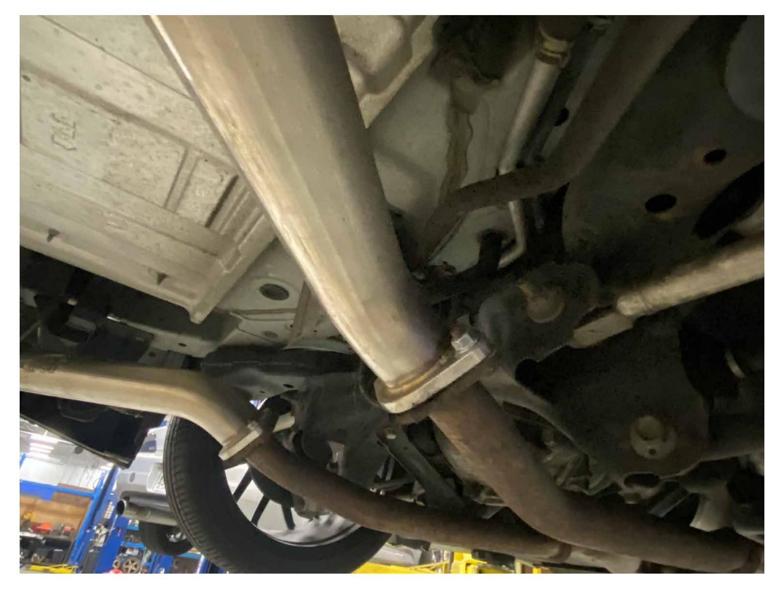
Secure to factory exhaust with included hardware and tighten to 35 FTLBS
