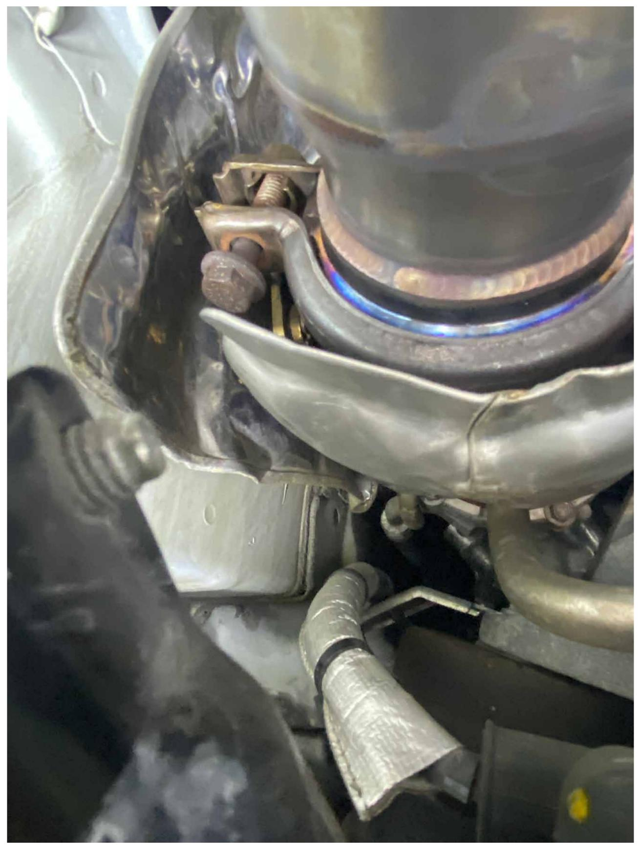
Using an extension and a 14mm socket, reinstall the vband bolt and tighten, it may be needed to pry the heat shield around the turbo open slightly to allow room for hands and tools
