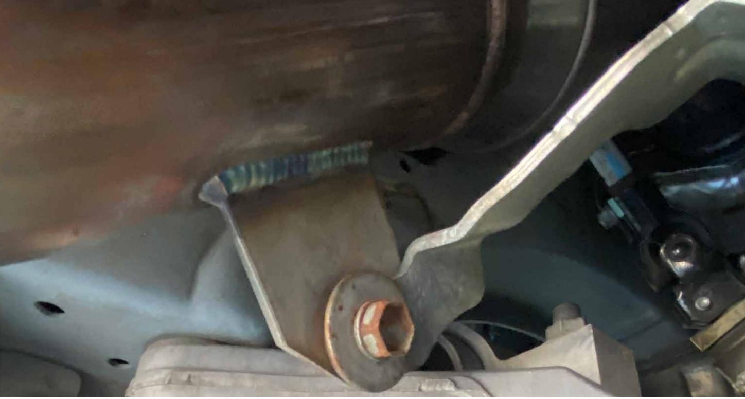
Tighten the midpipe connection and hanger connection
