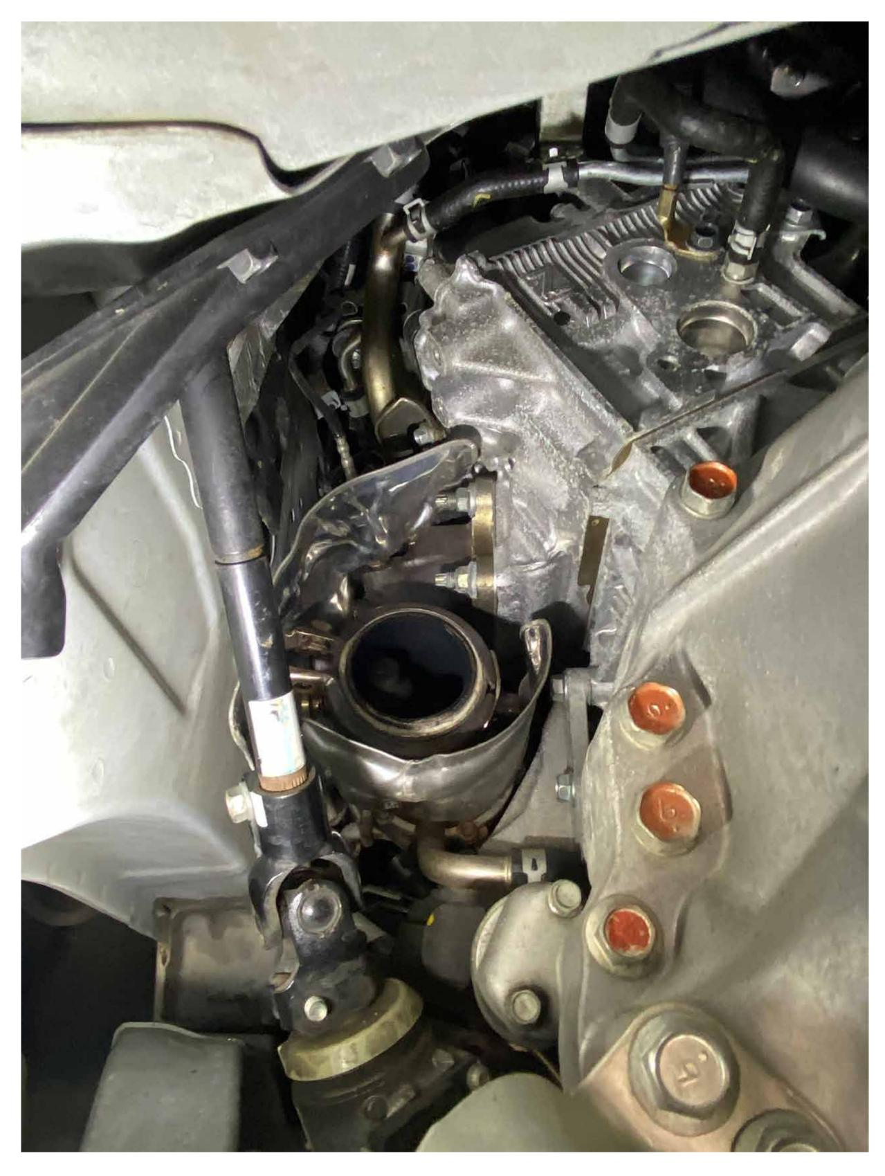
Slip vband clamp over the MAP downpipe, we have found it to be easier with the bolt removed from the downpipe
