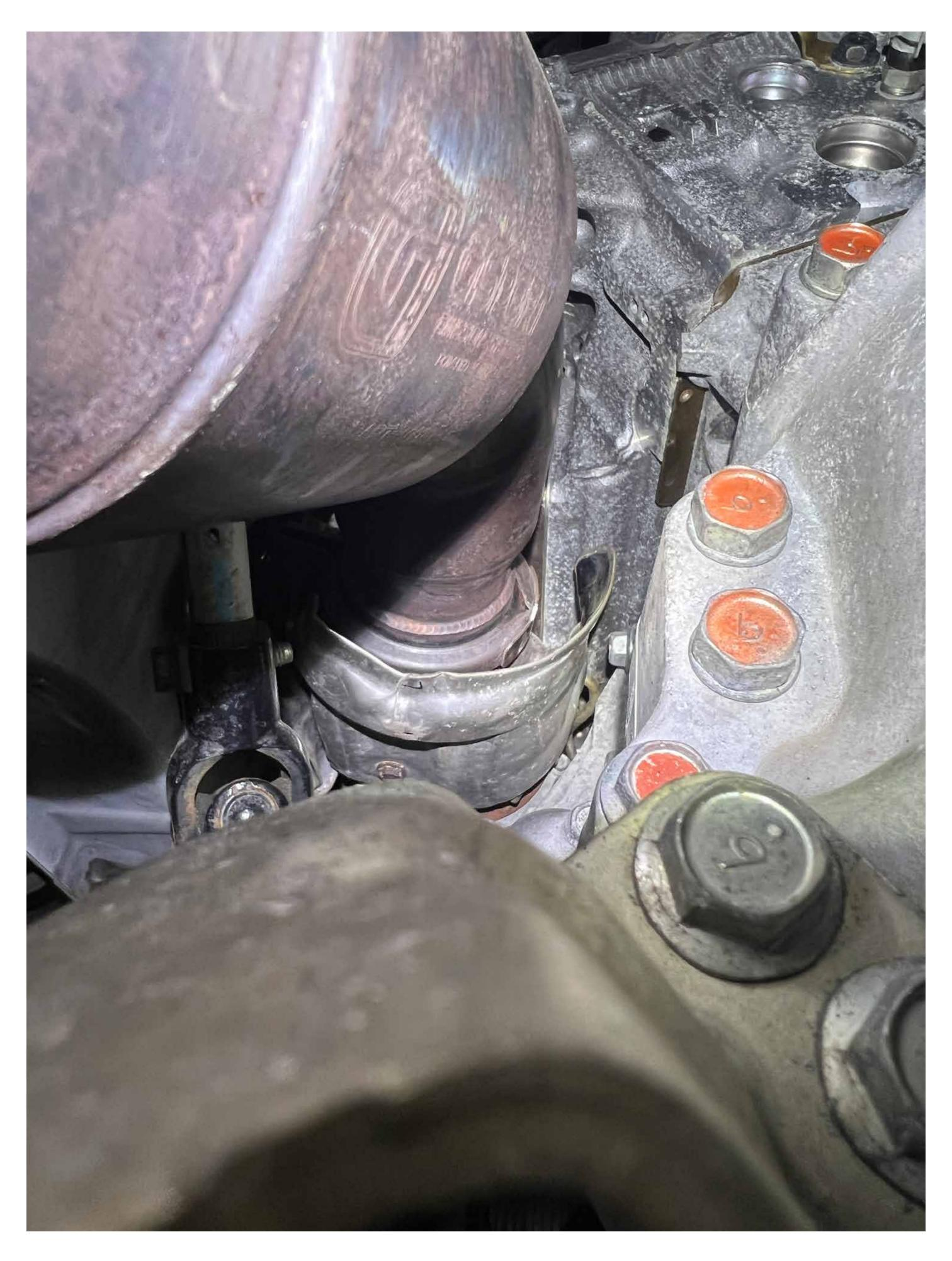
Push the downpipe upwards until the vband on the MAP downpipe meets with the outlet flange on the turbo
