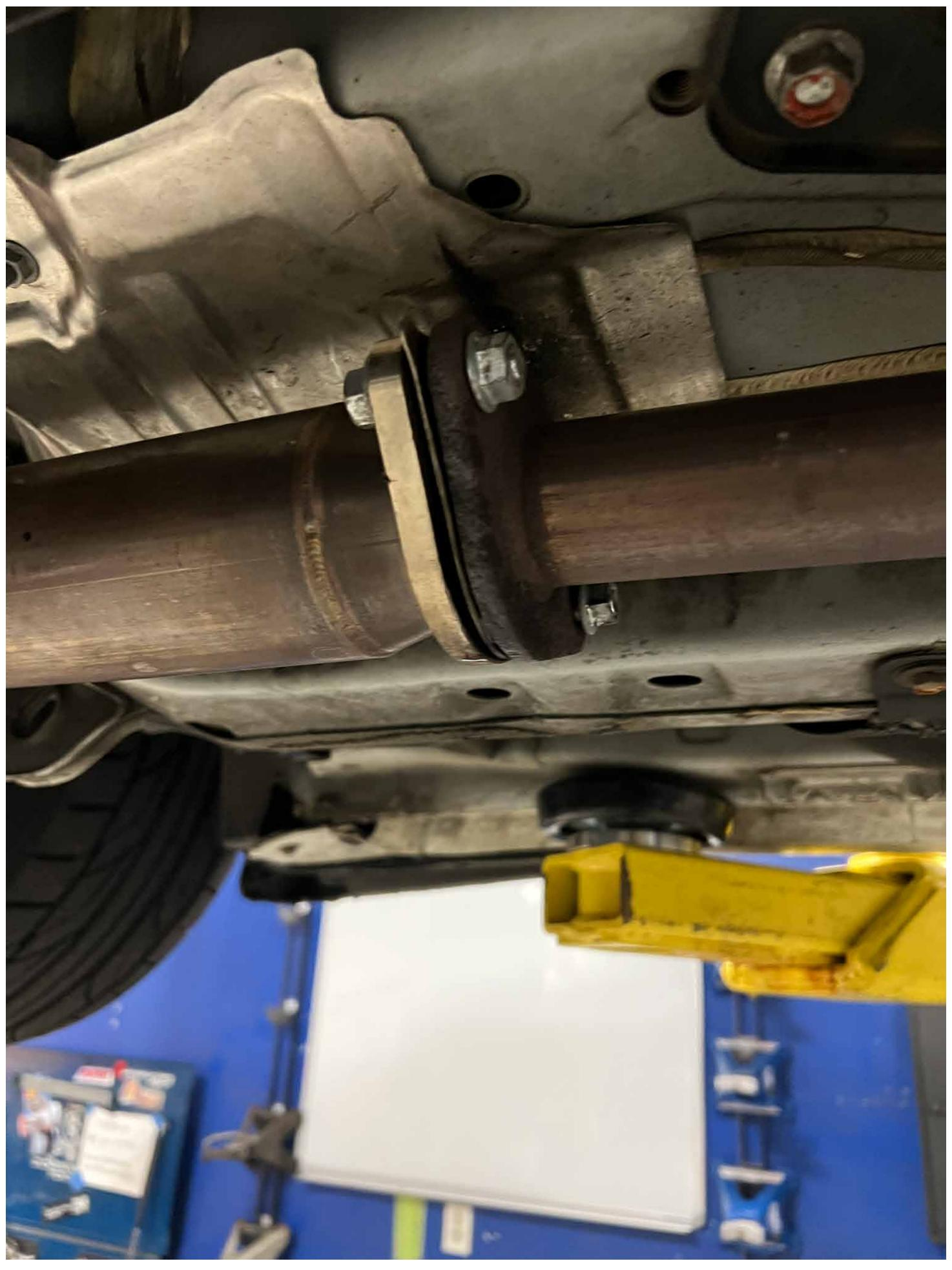
Attach MAP downpipes to the midpipes with included hardware, and leave the connection loose until a later step
