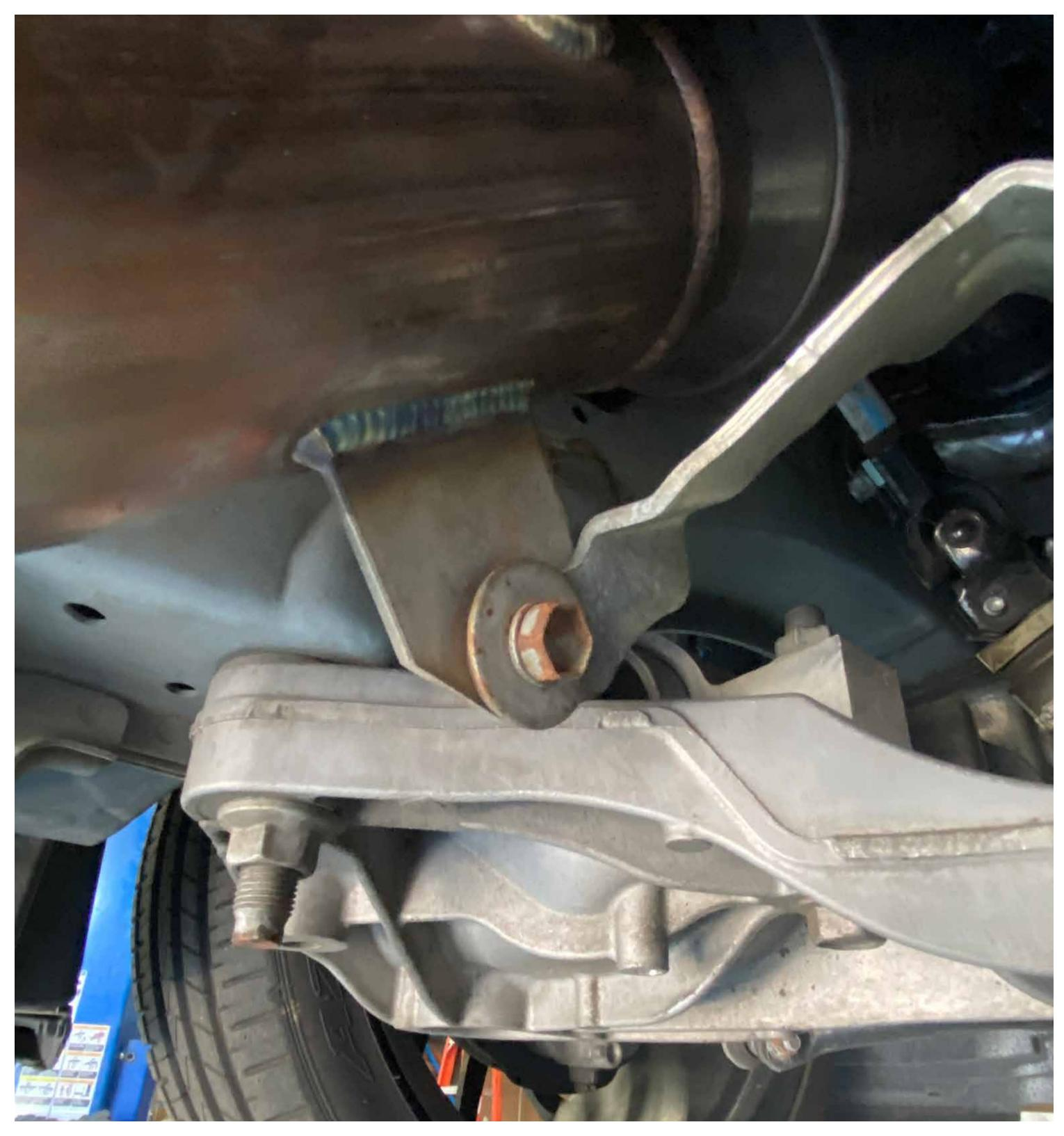
Attach downpipes to OEM downpipe hanger brackets and leave the hardware loose until a later step
