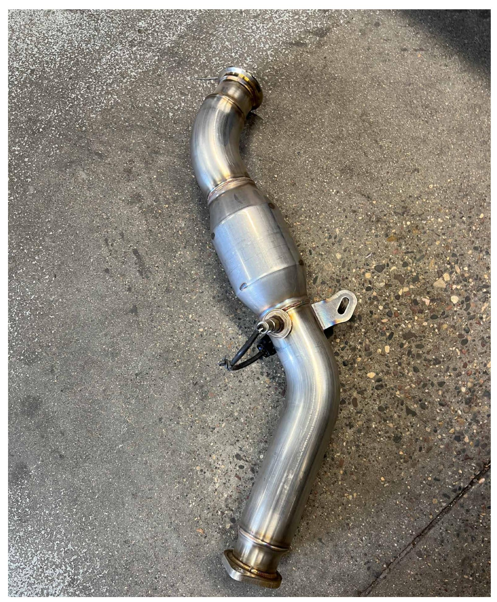
Install 02 sensors into the downpipes with 02 sensor socket to avoid damaging the sensor
