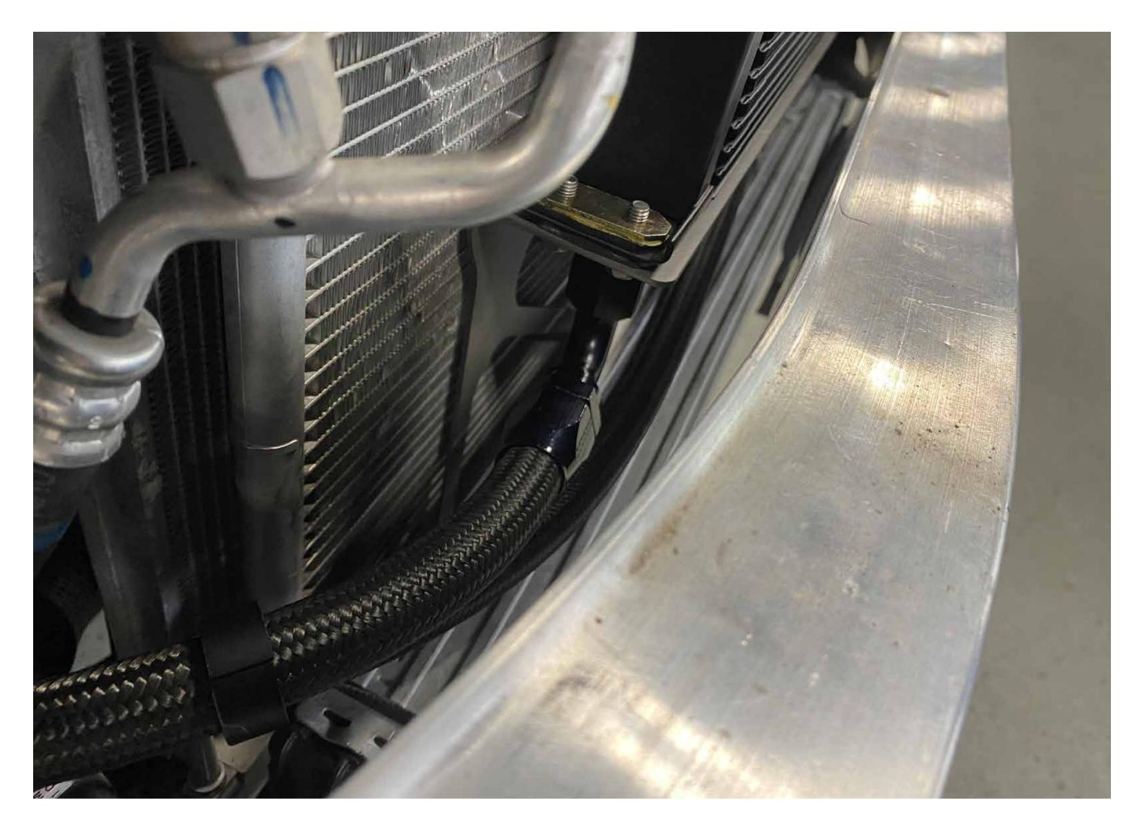
Install included oil sandwich, clock the inlet and outlet as pictured. Tighten to (ftlbs) reinstall oil filter when your finished
