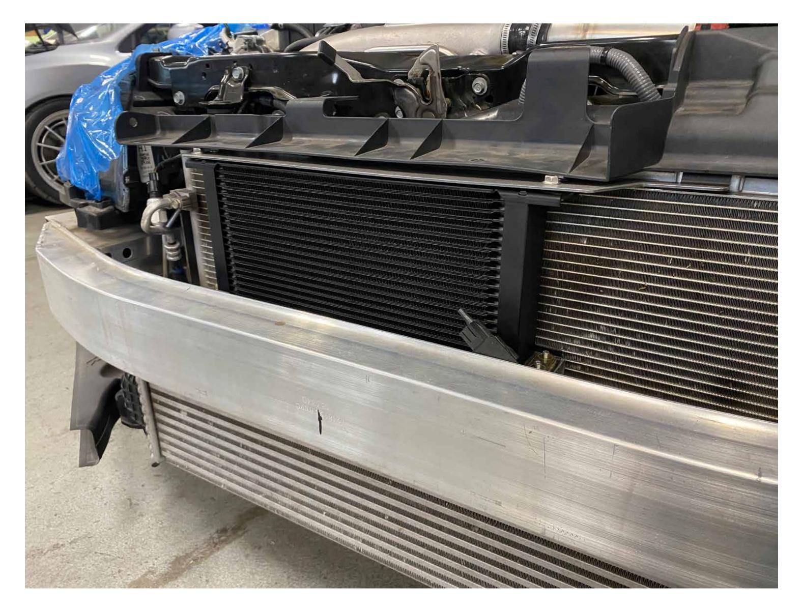
Next, attach MAP FK8 Type R oil cooler to the vehicle by securing it to the radiator condenser, using the 4 10mm bolts you removed earlier.
