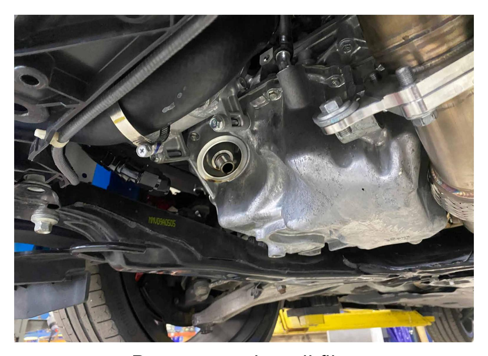
Remove engine oil filter
