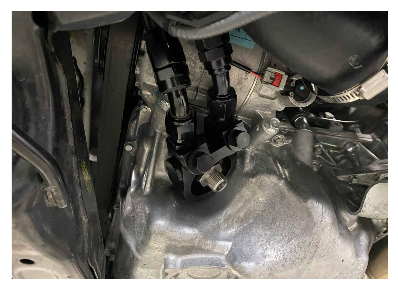
Thread AN Lines onto the oil cooler, longer line goes on drivers side and shorter line will go on passenger. Route as pictured and thread onto oil sandwich plate, once all lines are in place, tighten all fittings and hose ends.
