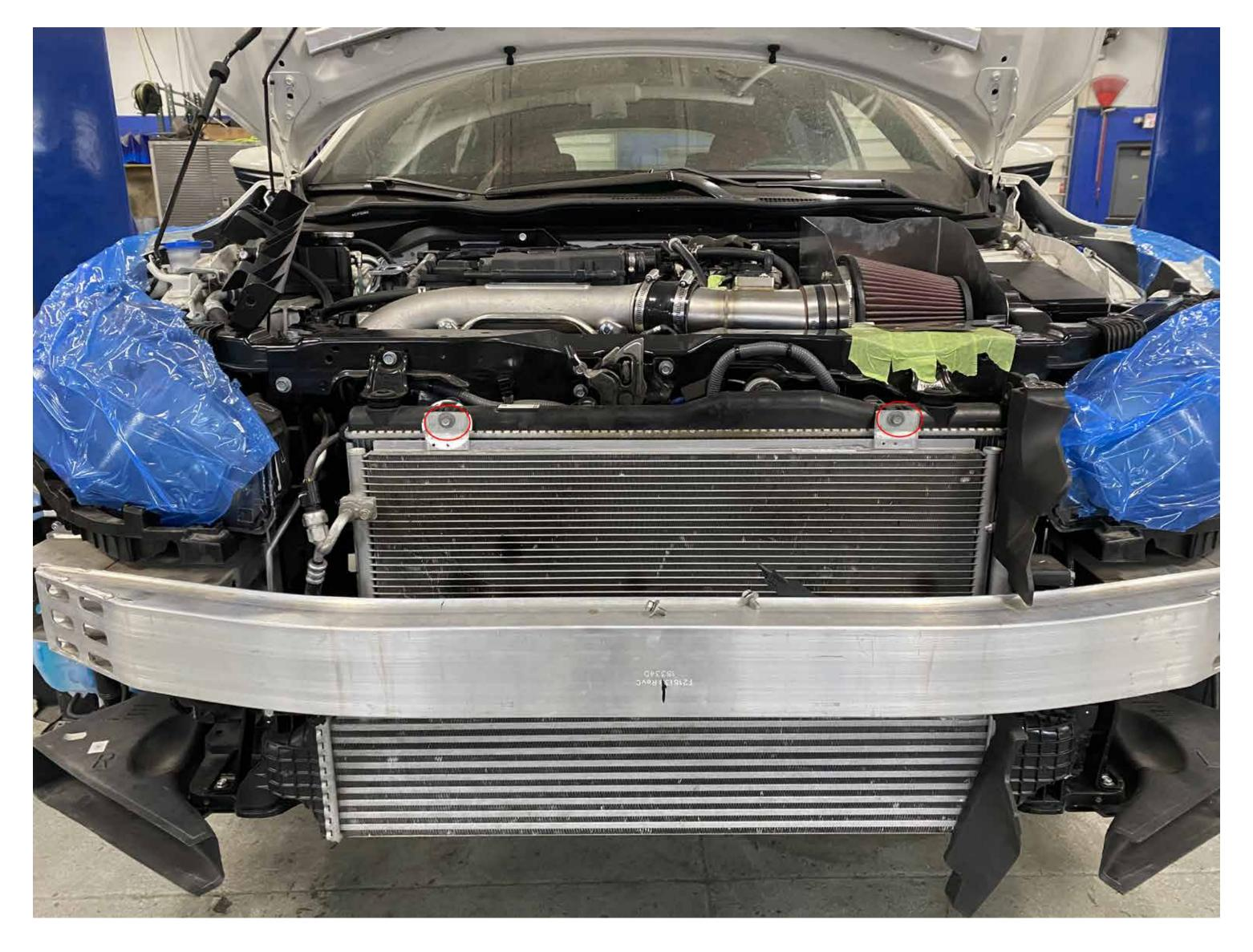
Remove 4 bolts holding AC condenser in place
