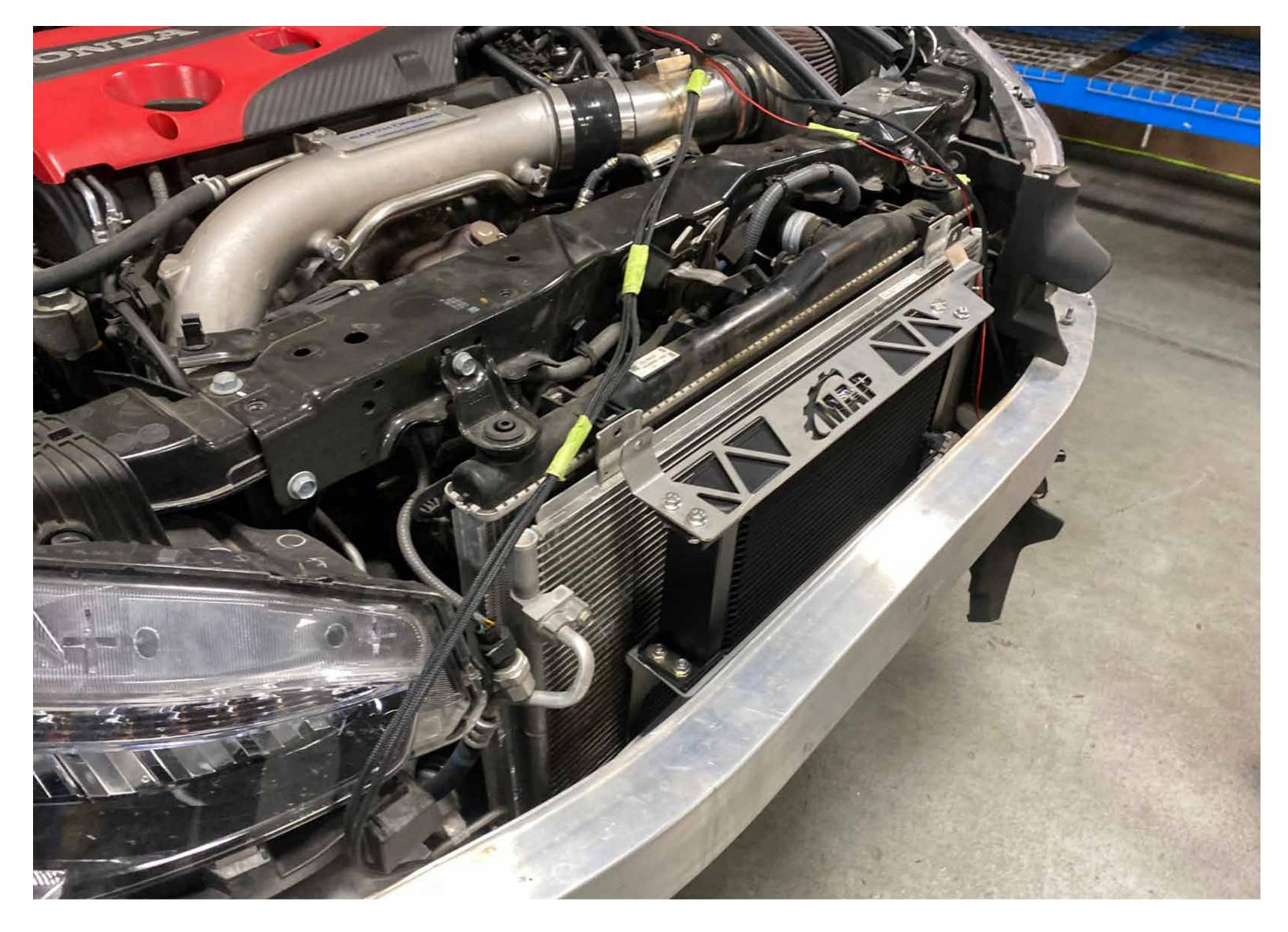
Add 1 qt of oil, start check for leaks and adjust oil level if needed
