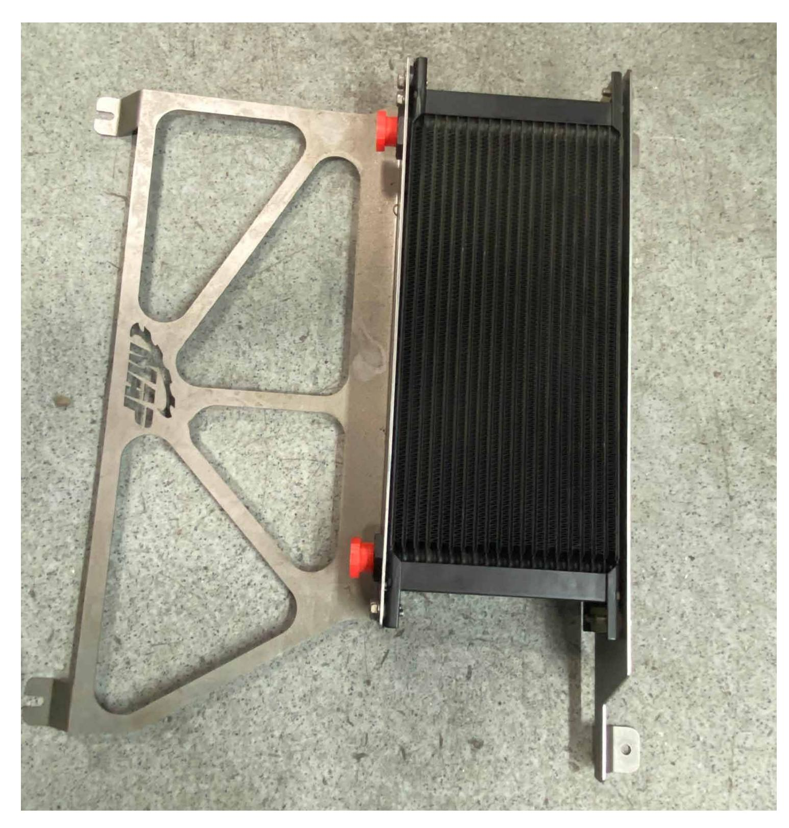
Assemble MAP FK8 Type R oil cooler as pictured, ensure you have rubber isolators on both sides of the brackets
