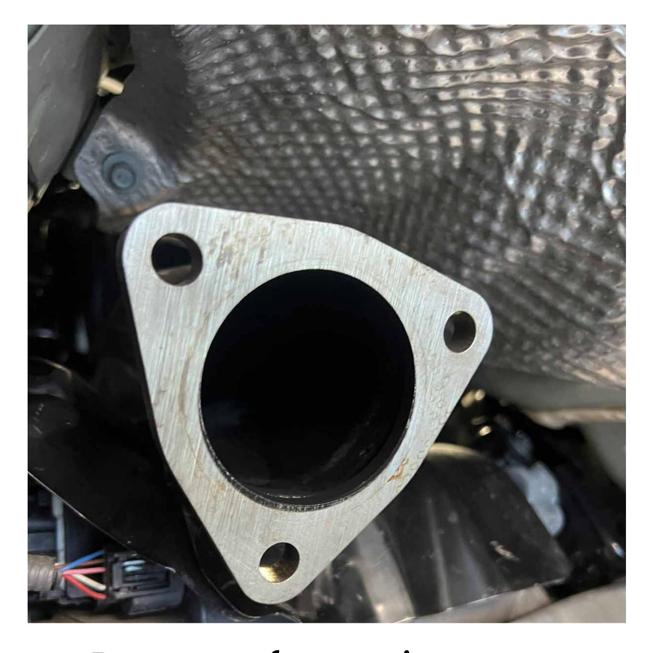
Remove front pipe nuts (14mm socket)
