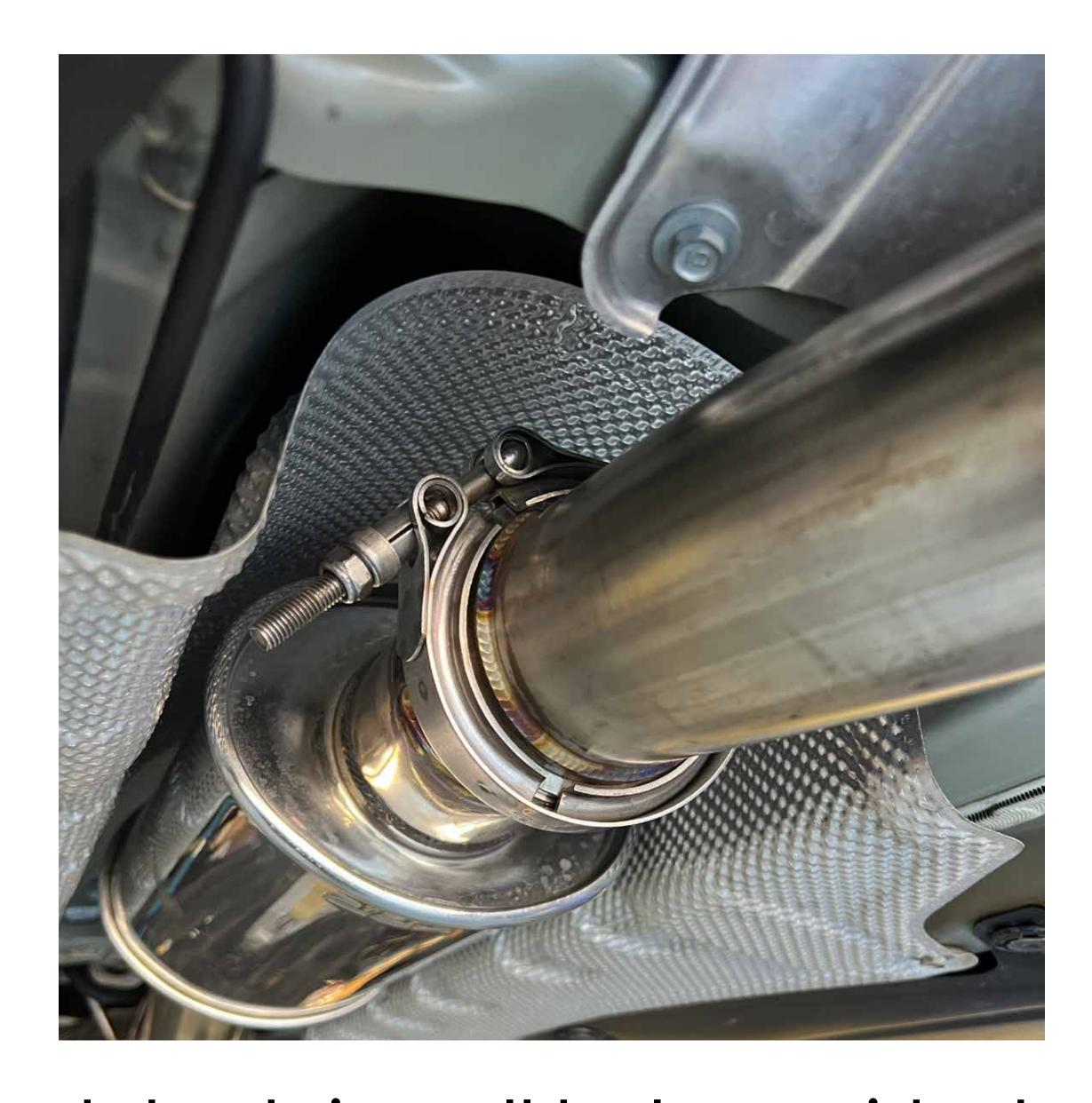
Attach both install halves with vband, align and and tighten with anti seize
