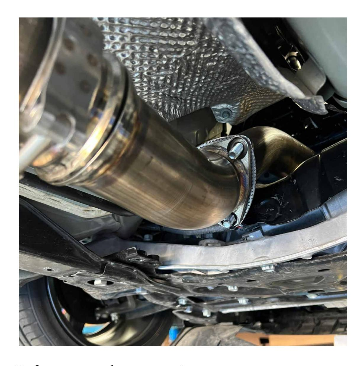
Install front pipe adapter, secure using included vband and nuts
