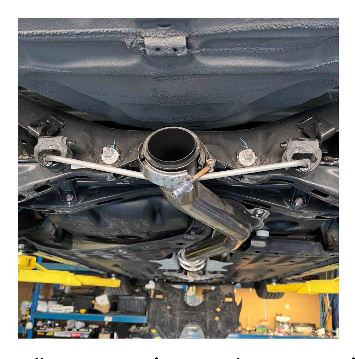
Install rear section and secure with hangers
