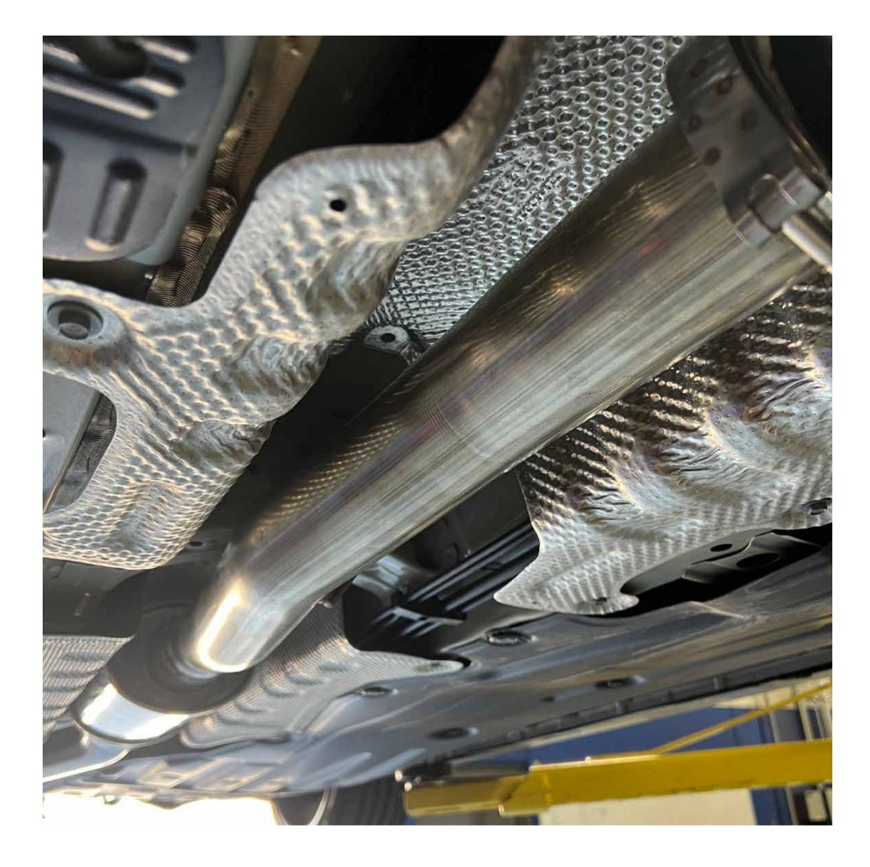
Install mid pipe section and secure with factory hanger (note the hanger has a specific "up" orientation)
