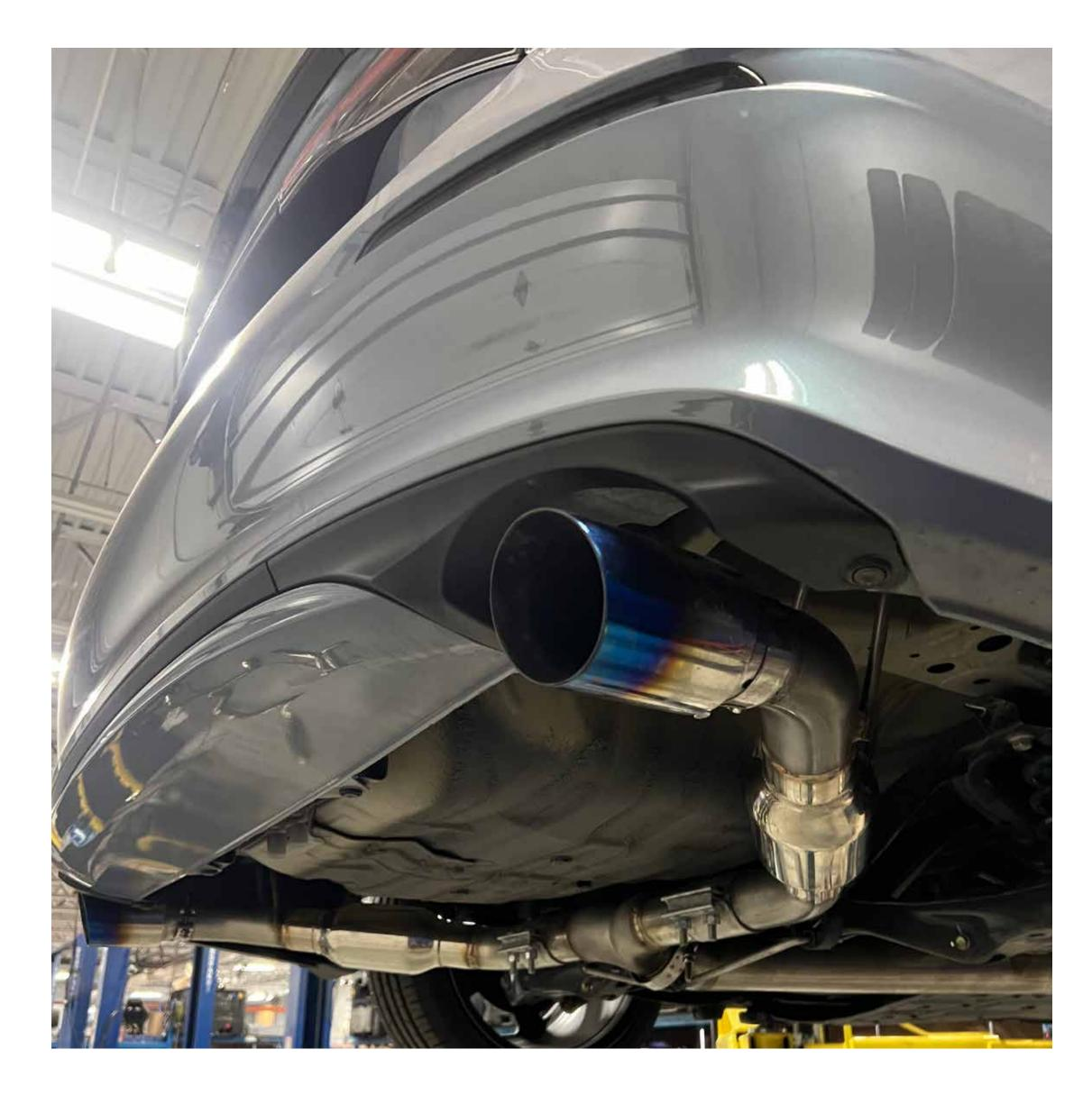
Once exhaust is level and even on both sides, install slip on tips, tighten clamps with anti seize
