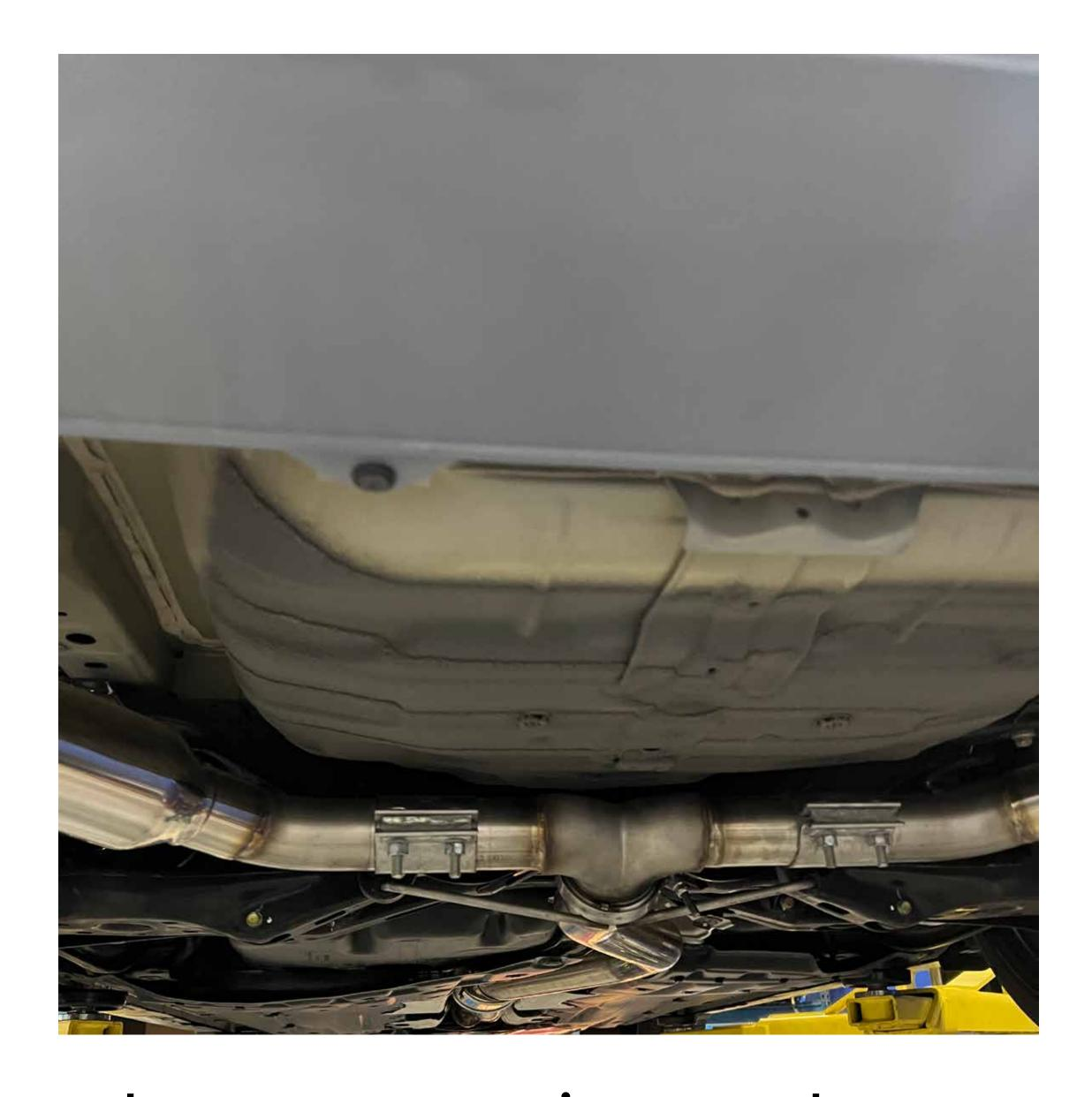
Attach rear y section and outer exhaust sections, secure with included vband and slip clamps. Be sure the outlet portion is secured to exhaust hanger
