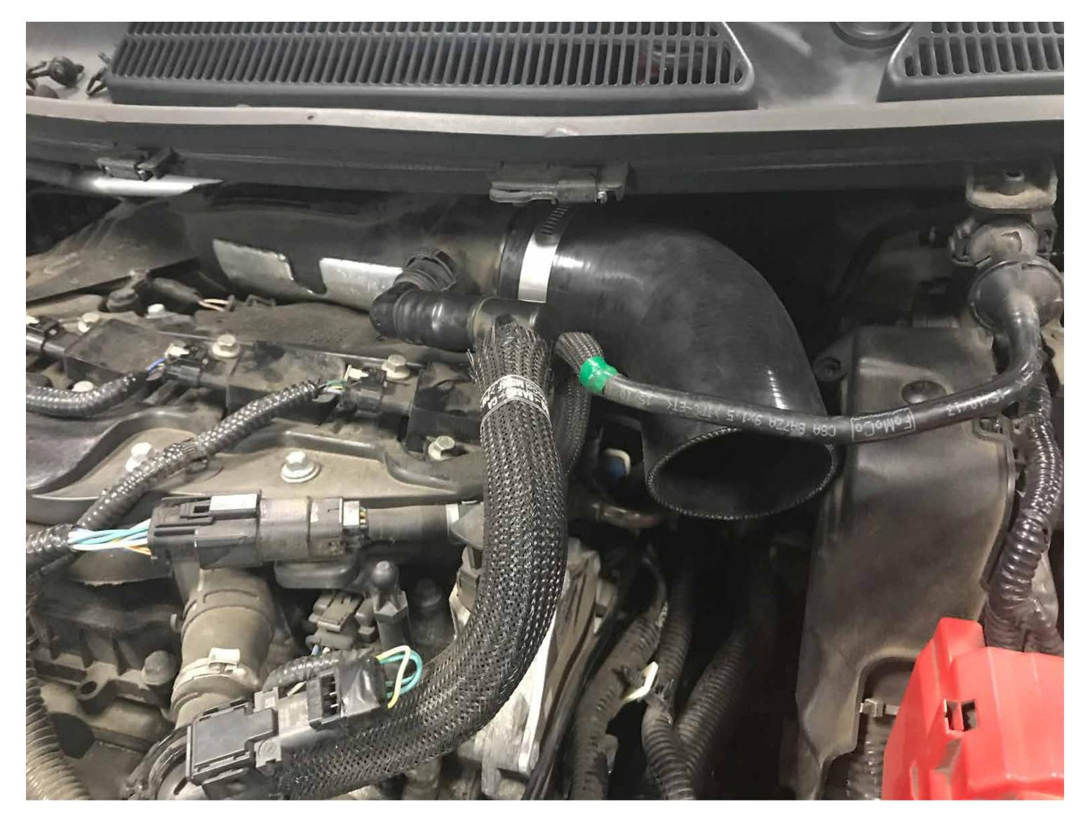
Install included coupler on the intake tube, tighten the included worm drive clamp
