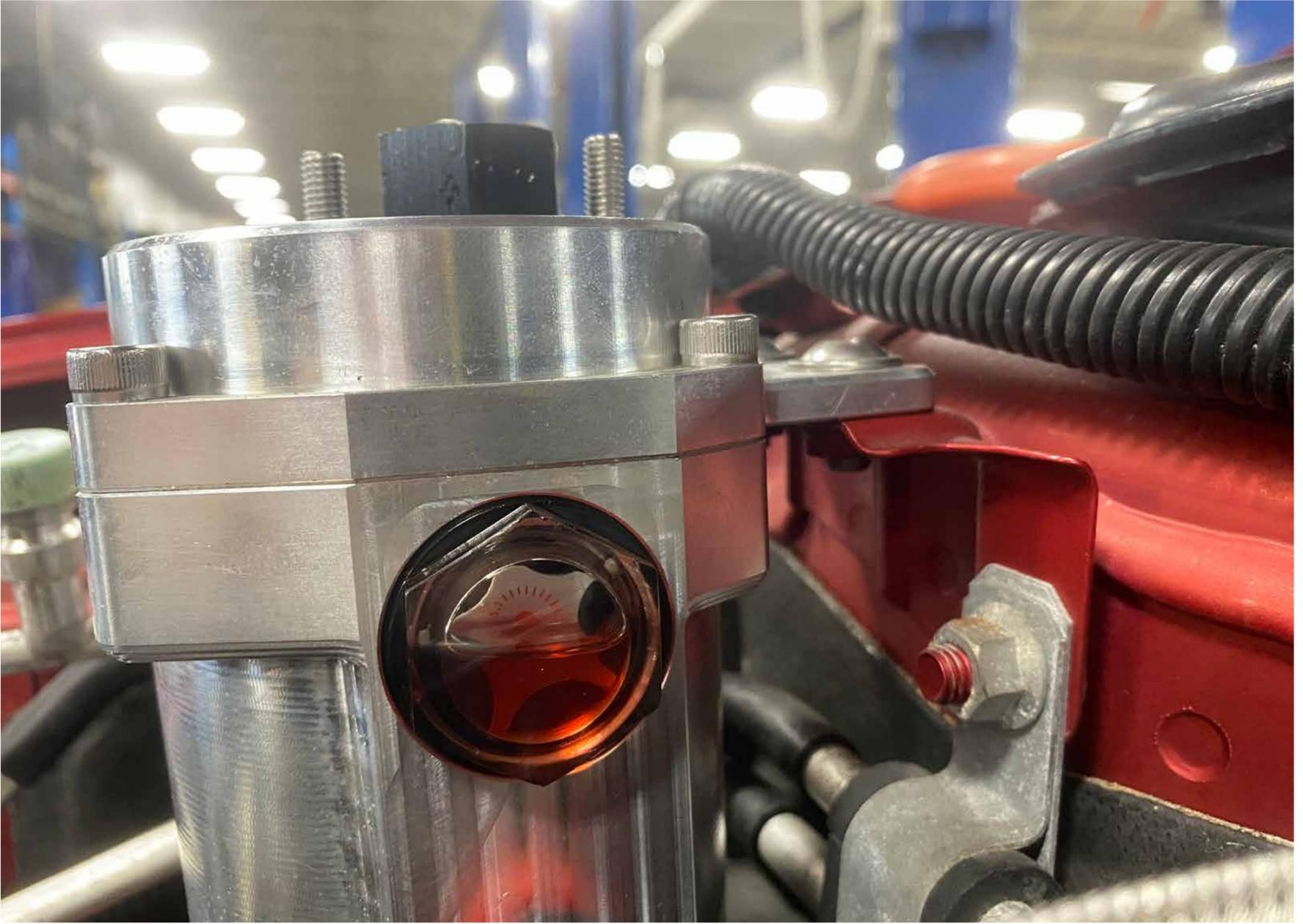
Fill PSR to the halfway point in the sightglass. It is important after install that you start the car, move the wheel side to side a few times and recheck the level to ensure the system is full.
