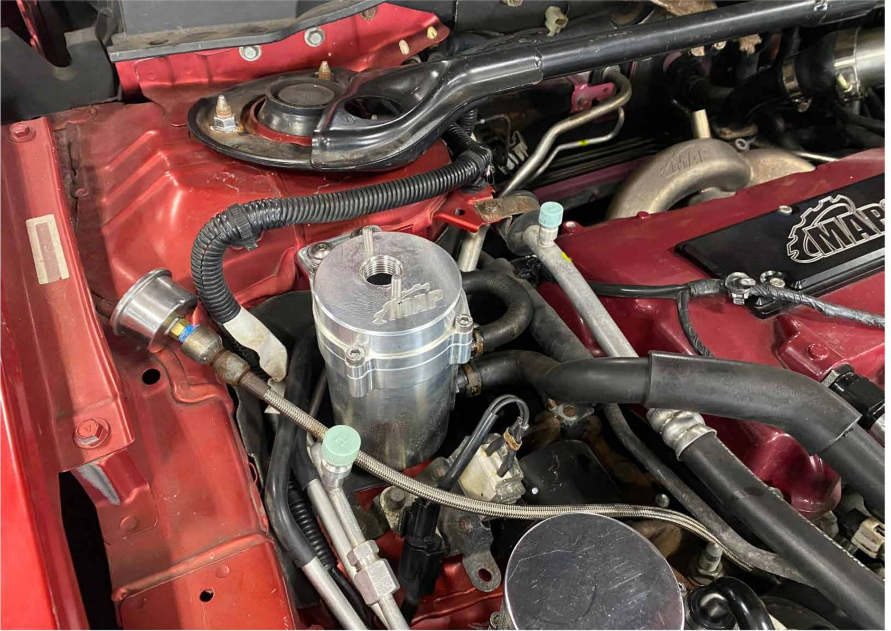
Attach MAP evox PSR to the factory reservoir mounting bracket using uncluded 5mm allen head bolts
