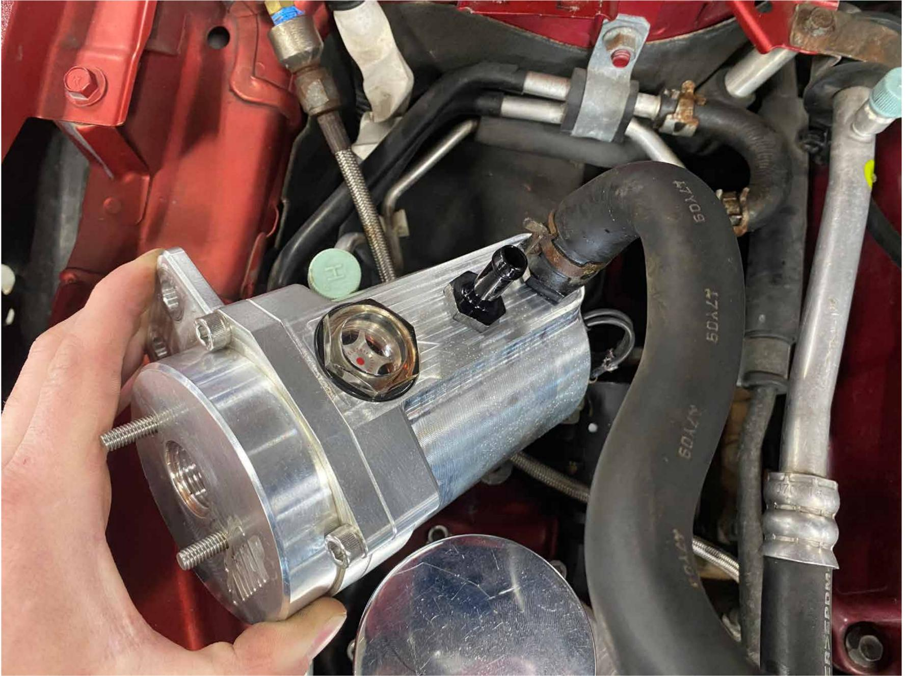
Attach lower hose to MAP evox power steering reservoir
