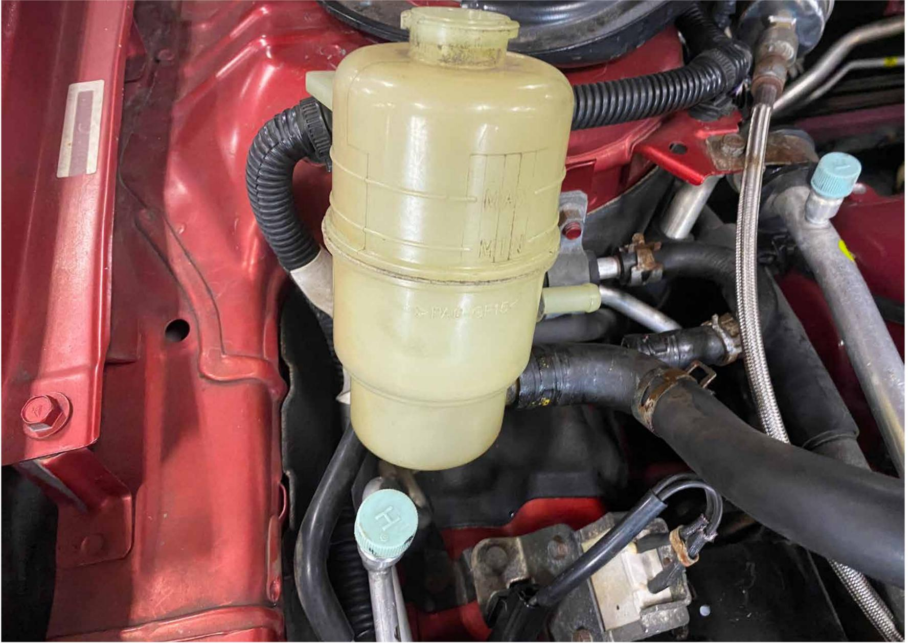
Move reservoir to the side and remove the lower hose
