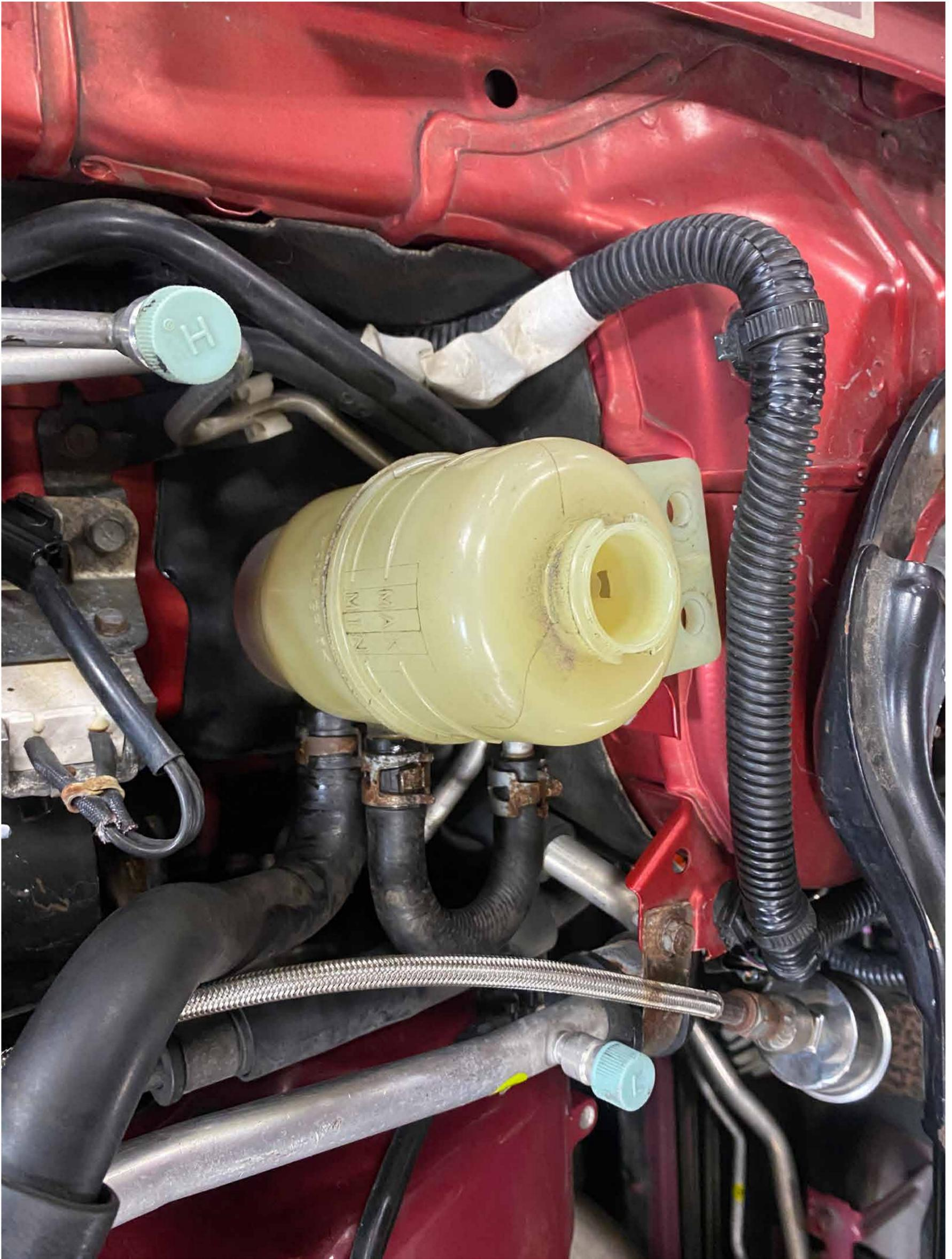
Remove 2 10mm bolts holding factory power steering reservoir to the vehicle
