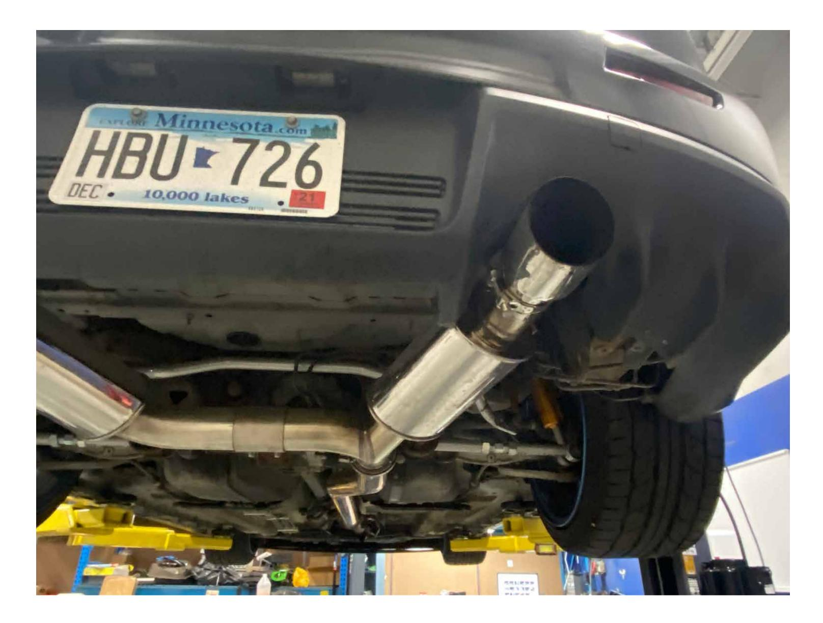
Install included slip on tips, ensure you are using anti seize grease on provided clamp to avoid galling. Start and check for leaks
