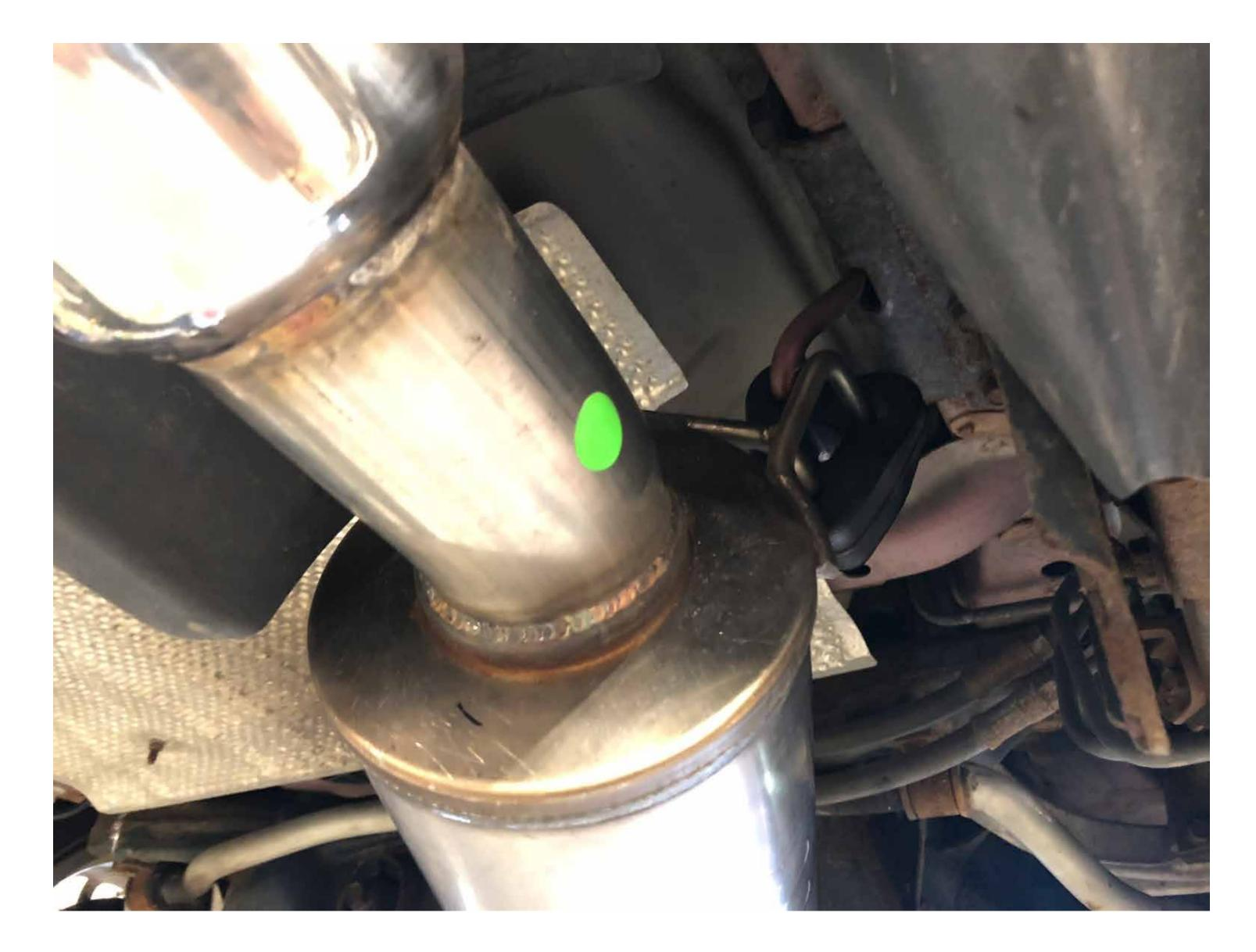
Install rubber hangers onto the muffler section, then install the mufflers into the vehicle securing It by the rubber hangers
