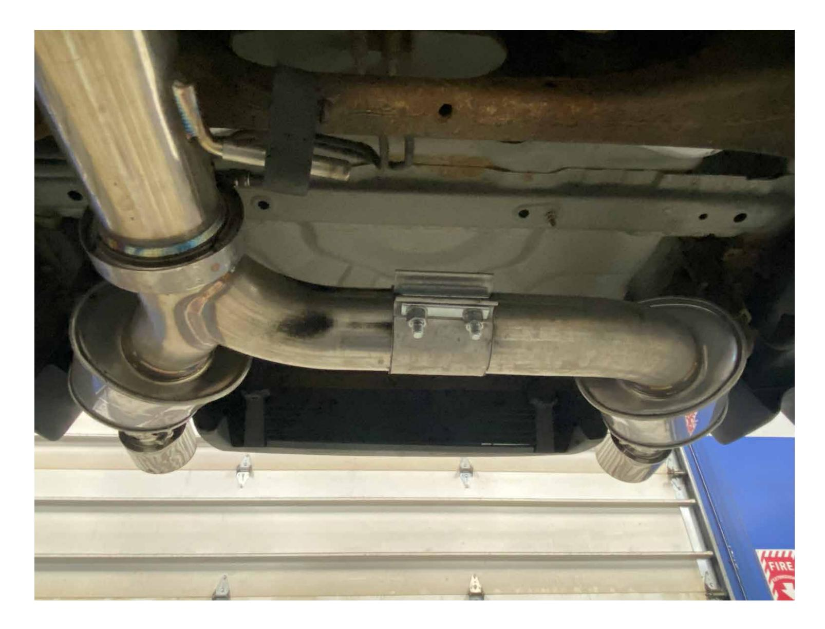
Only follow this step if you have dual exhaust option. Install slip clamp between 2 muffler sections, ensure mufflers are clocked straight before tightening clamp
