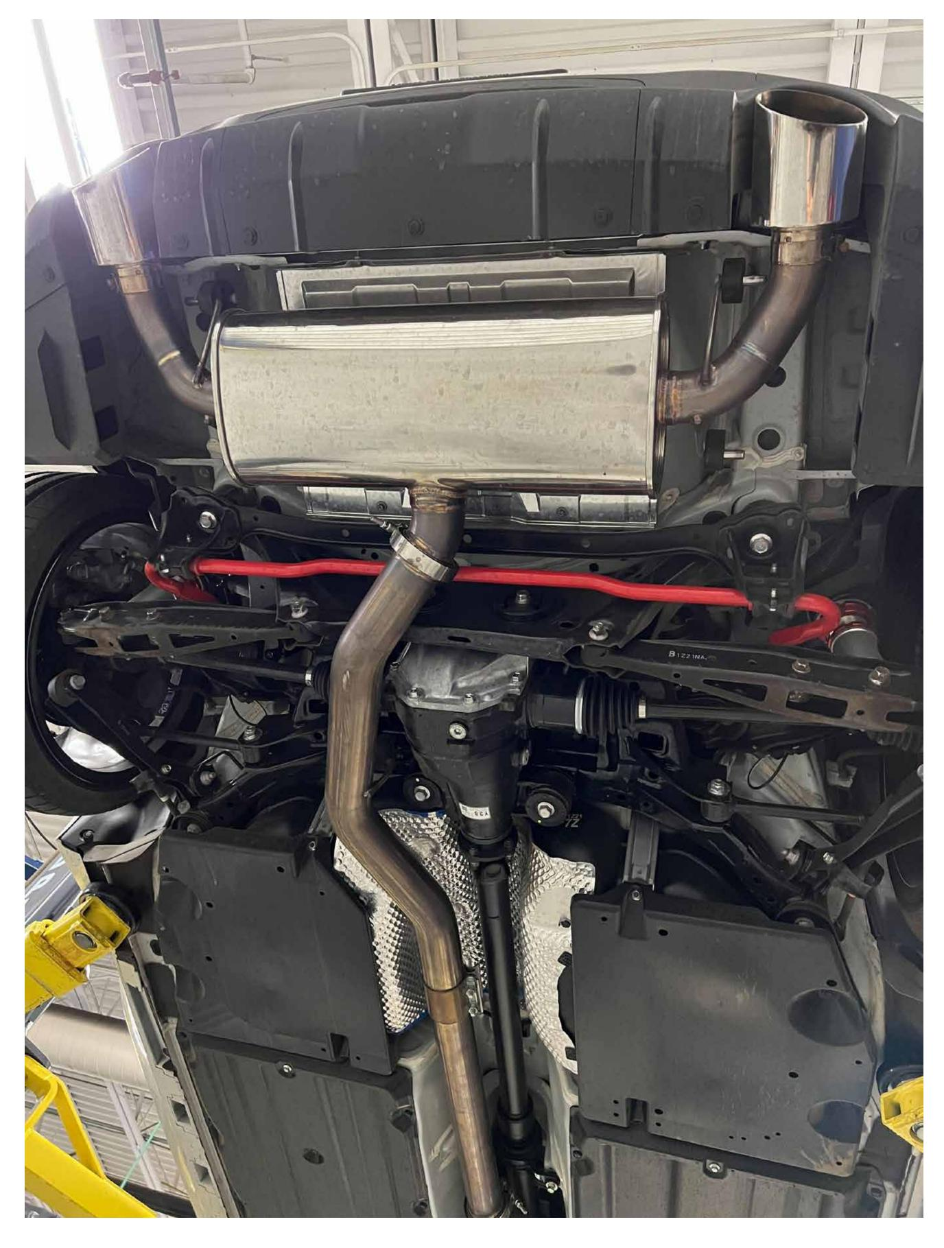
Tighten all clamps, working from front to back making sure muffler is centered in the bumper and tip cut outs
