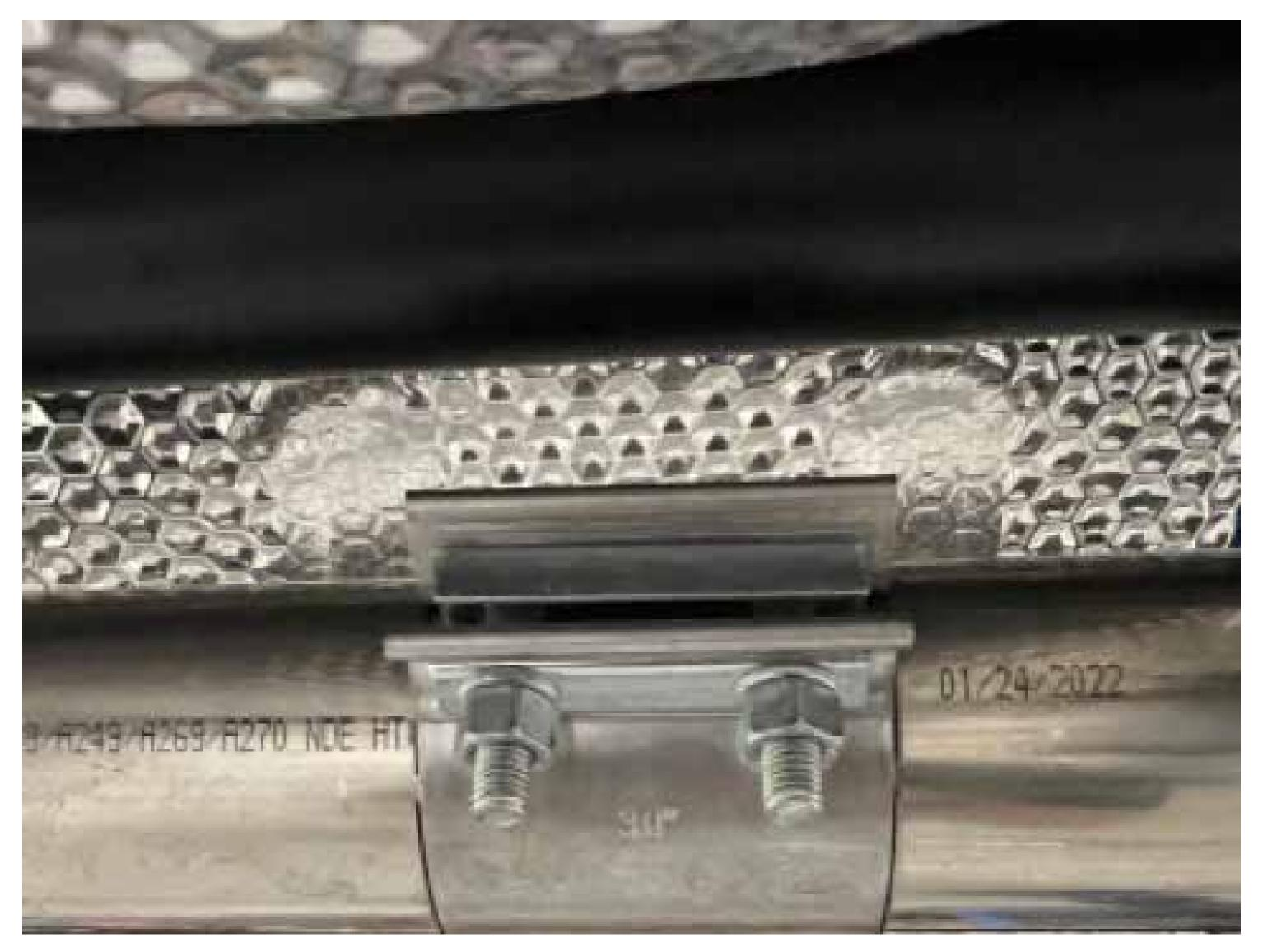
Attach All pieces of MAP catback with included vband and slip clamp if you are installing this catback on a gen 1 86, the pipes should be butted up to eachother in the slip clamp, if you are installing on a gen 2 86 there should be a slight gap. The mid pipe hanger should be perfectly straight and give reference for if you have done this right.
