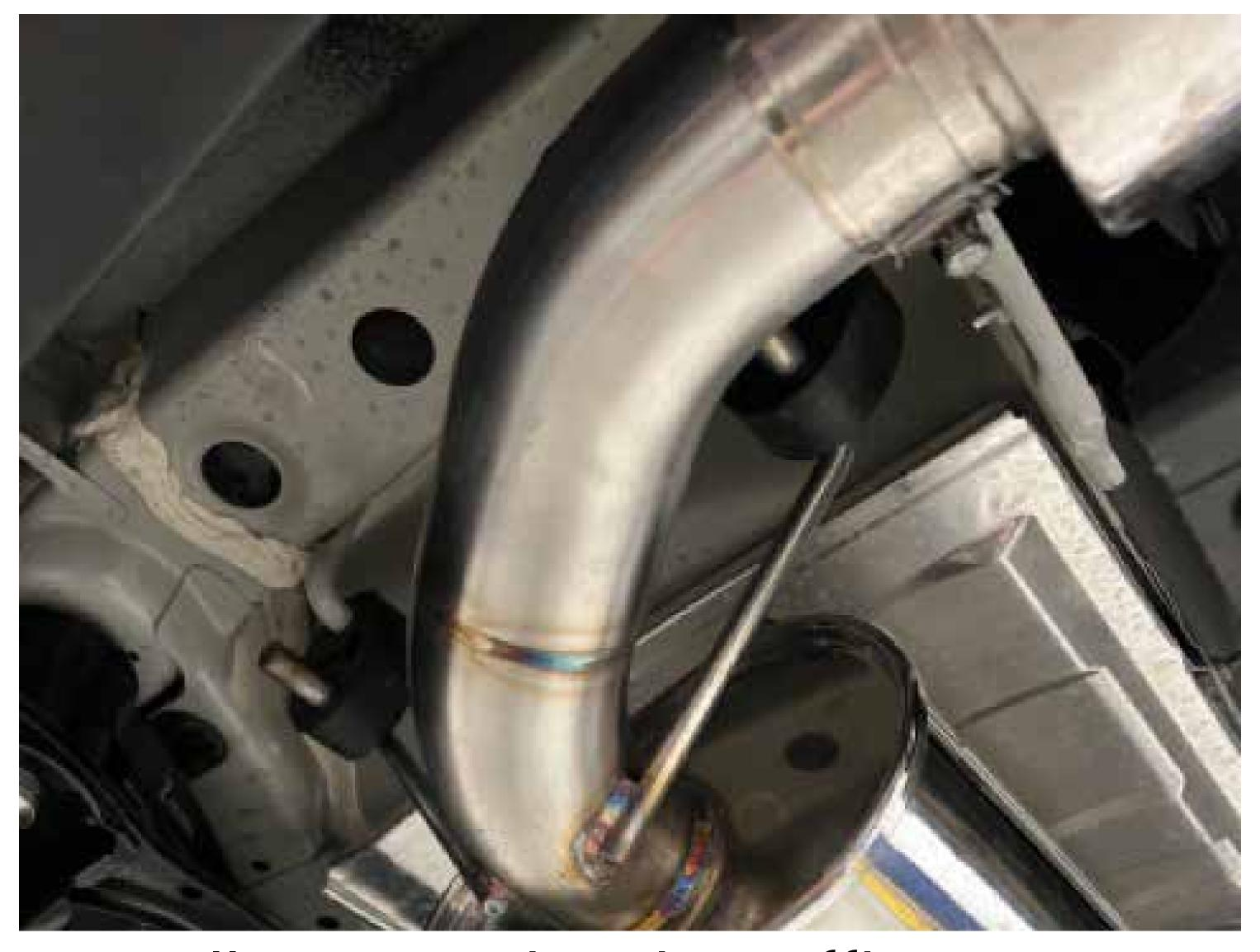
Install MAP catback muffler to 4 oem muffler hangers
