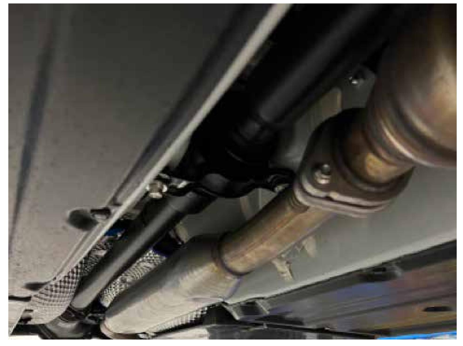
Remove 2 14mm spring bolts attaching factory catback to front pipe
