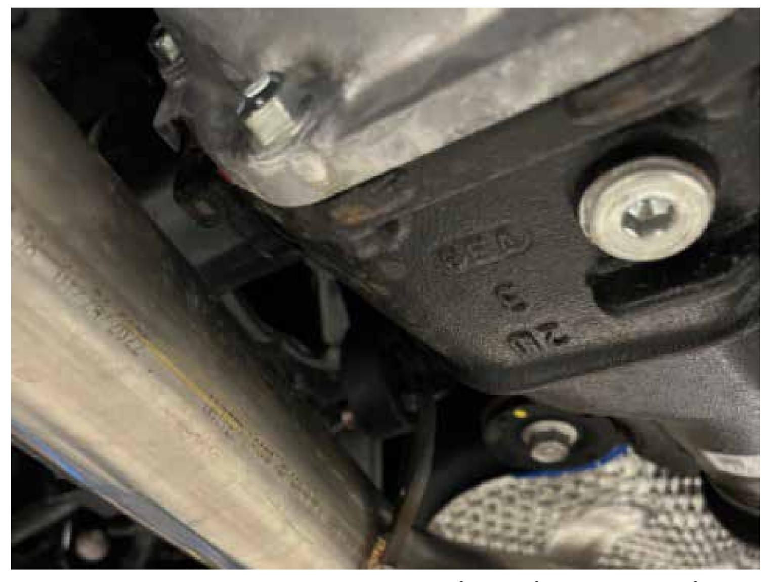
Install MAP catback mid pipe section, securing it via the oem hanger
