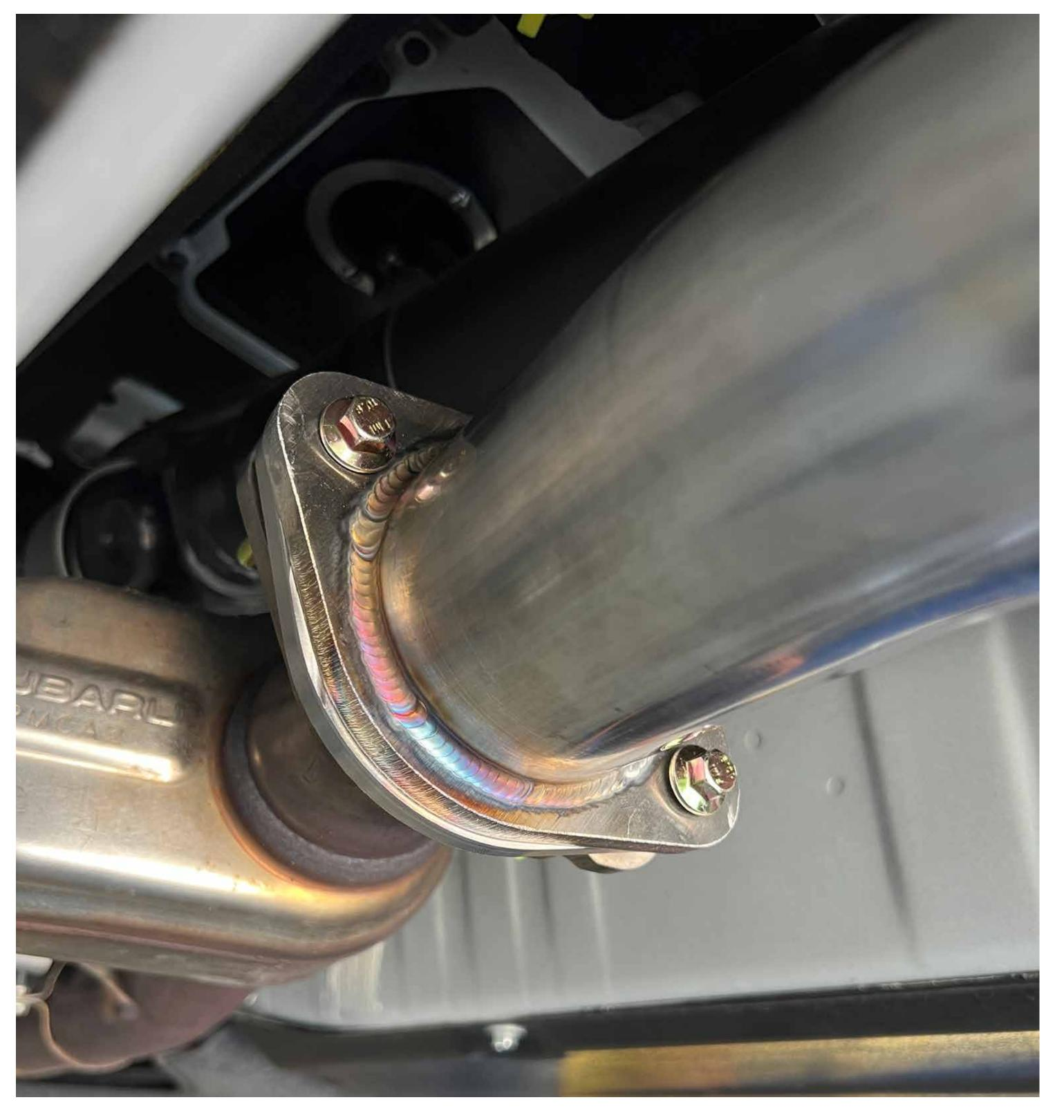
Install MAP Catback front pipe to downpipe. Do not tighten completley. Install Grimmspeed adapter flange if using factory downpipe
