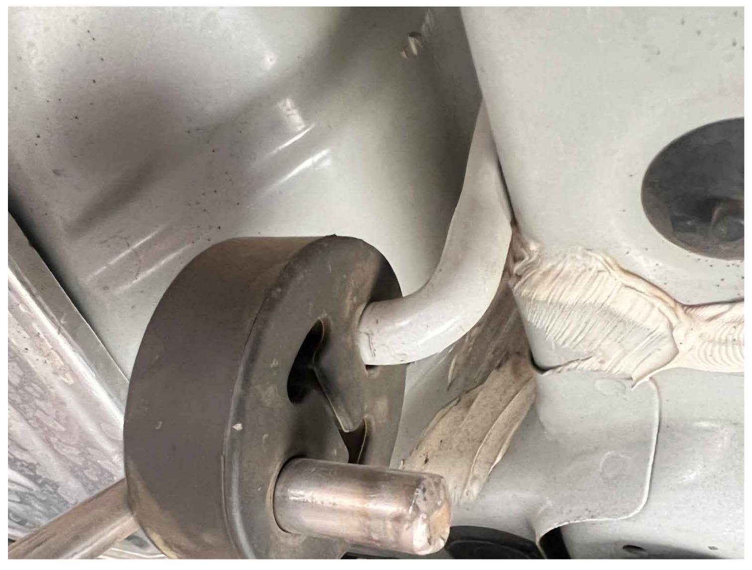
Remove 4 muffler hangers from muffler and remove muffler from car
