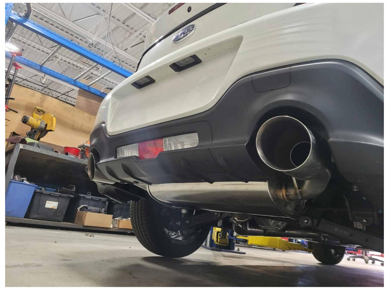
Once fitment is verified correct, install included slip on tips be sure to use anti seize on threads of tip clamps. Use hand tools to tighten
