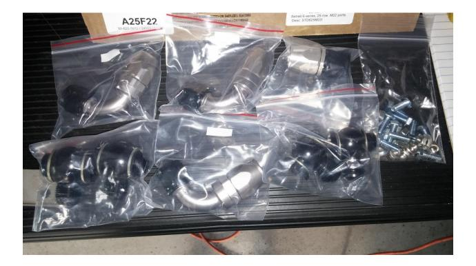
Once everything is laid out you can start to assemble your new oil cooler. First thing first is to open the bag of bolts, washers, and nuts included. You will need these for the brackets to oil cooler.
