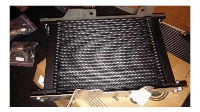
At this point you're going to want to start taking the OEM oil cooler off. This is pretty easy to do as the bolts to the cooler itself are easily accessible. 3 Bolts in total for the OEM cooler.
