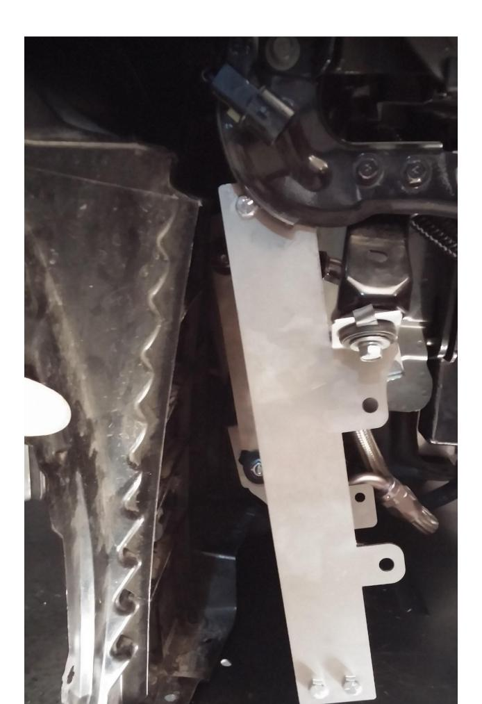
Now that everything is mounted and tightened up, you can mount the OEM air guide to the brackets; start the car up and check for leaks.
