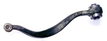
SPF3129K is a standard replacement kit SPF3130K will +/- the caster one side & standard the other SPF3131K will +/- the caster both sides of the car
