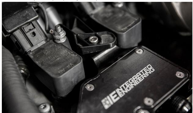
**24.** Carefully remove the clamp holding the short rubber hose to the evap solenoid on the valve cover. Replace it with the included vacuum line and check valve. Connect it to the vacuum fitting on the breather plate and secure all ends with the included zip ties. *Note: Take care to install the check valve correctly, arrow on check valve should be pointing towards from the breather plate.*
