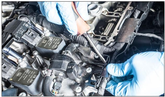
**16.** There is a single area of the wire harness wrapped with tape, which must be carefully trimmed for removal.
