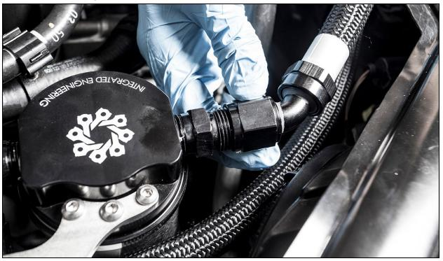
**32.** Connect the straight end of the inlet hose to the left side of the breather adapter. Tighten using an AN wrench.
