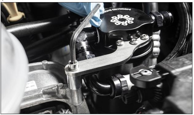
**31.** Attach the 45 degree end of the shorter hose to other catch can inlet.
