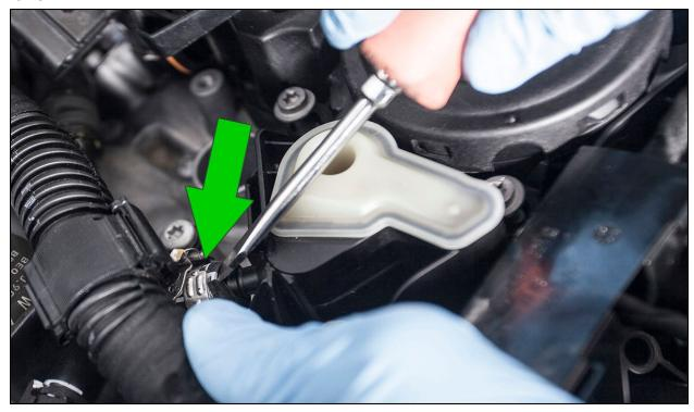
**11.** Using a torx driver, loosen the seven T30 torx bolts from the PCV valve and remove it from the valve cover.
