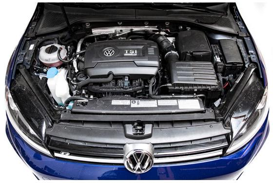
**2.** Start the installation procedure by removing the stock engine cover, pull up on the corners to release the grommets and set aside.
