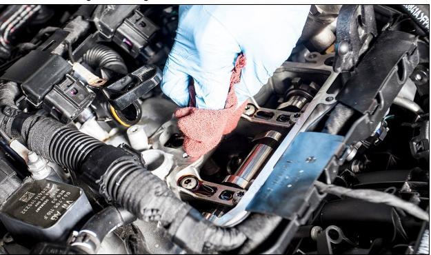
**18.** To ensure a proper seal, apply a small amount of silicone sealant to the new IE breather plate as shown below.
