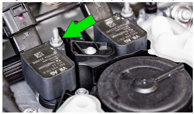
7. Using a T30 torx driver, remove the torx bolt from the PCV breather return hose.
