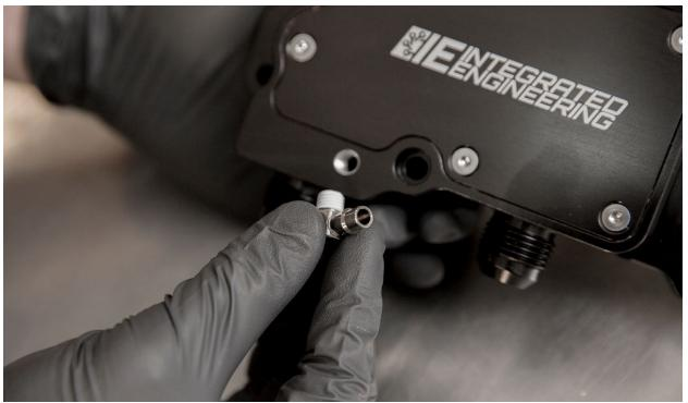
**14.** Install the vacuum fitting to the top port of the IE breather plate. *Note: Make sure the vacuum fitting is installed pointing in the direction shown below.*
