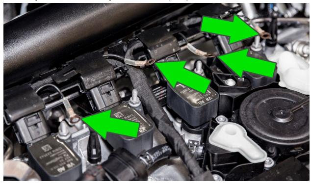
**5.** Carefully disconnect all coilpack harness connectors from the coilpacks.
