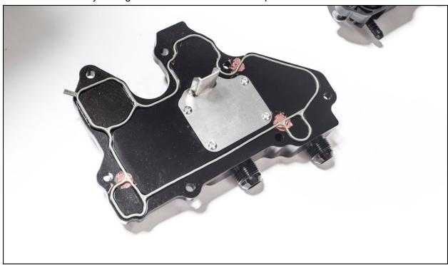
**20.** Place the IE breather plate into position, install the M6X35mm front bolt between the inlet and outlet barbs using a 5mm allen.
