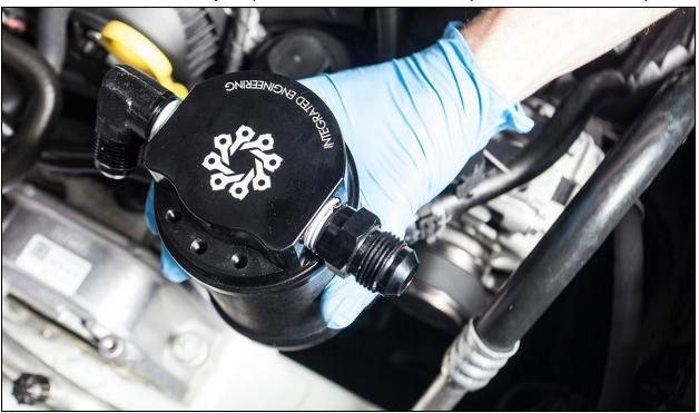
**28.** Install hose with 90 degree end onto 90 degree fitting using an AN wrench. *Note: Do not over tighten hose onto fitting, they only need to be snug to properly seal.*
