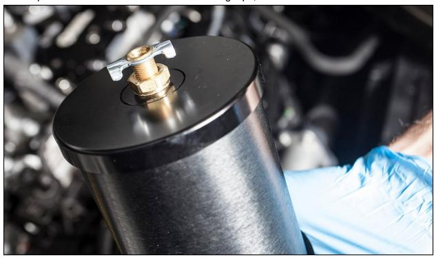
**27.** Wrap NPT threaded ends of both inlet and outlet fittings and install to catch can as shown below. *Note: Make sure to only wrap the NPT threads, do not wrap the AN threads with tape.*
