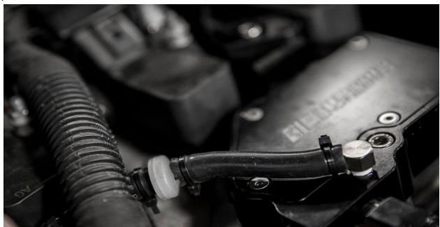
**25.** Reroute the wiring harness that runs across the front of the engine beneath the inlet and outlet of the breather plate. Secure harness to bracket near the evap solenoid using two of the included cable ties.
