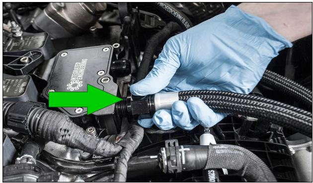
**33.** Connect the 45 degree hose end of the longer outlet hose to the right side of the breather plate. Tighten using an AN wrench
