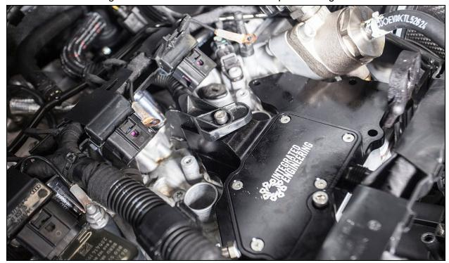
23. Reinstall coilpack, coilpack post, eyelits, coilpack harness connectors, and 10mm nuts.
