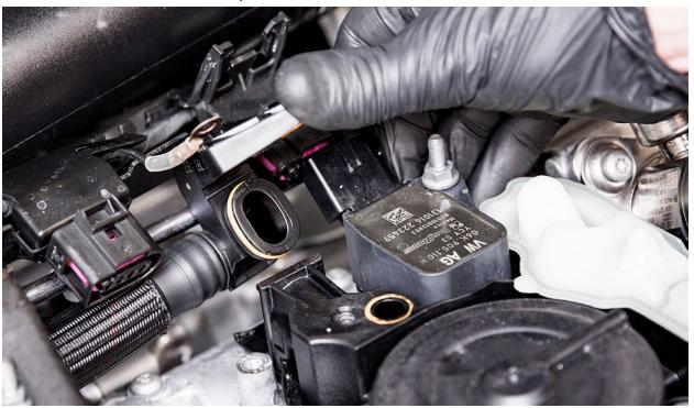
**10.** Using the OE tool or a flathead screwdriver, remove the rubber evap hose from the PCV valve.
