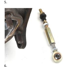
7. Screw the inline ball joint into the threaded hole on the bracket.
