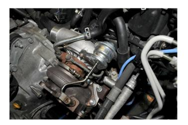
2. Remove the boost line from the top nipple on the actuator.
