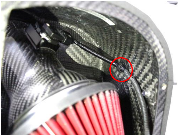
29. Push the MAF sensor wire into the clip at the back of the airbox.
