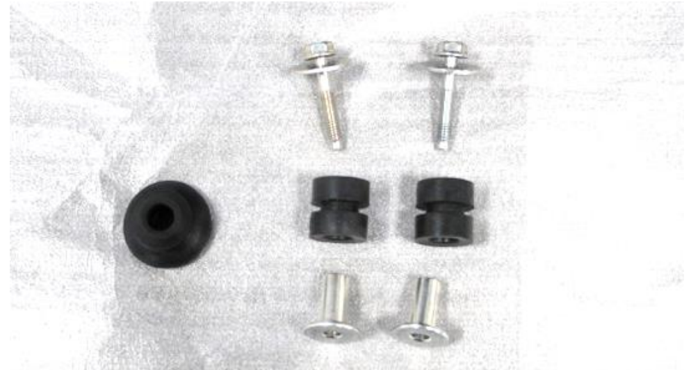
18. Here are the 2 rubber mounts with bushes and bolts and the rubber grommet removed from the airbox.
