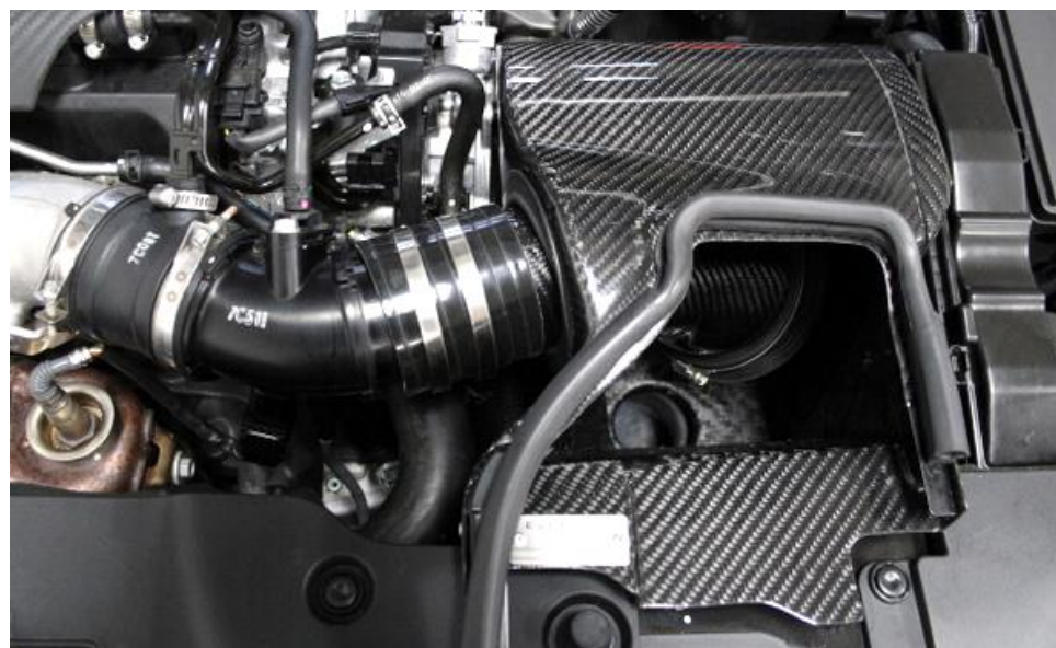
31. Carefully lower into the engine bay and locate the silicon hose onto the stock inlet tube.
