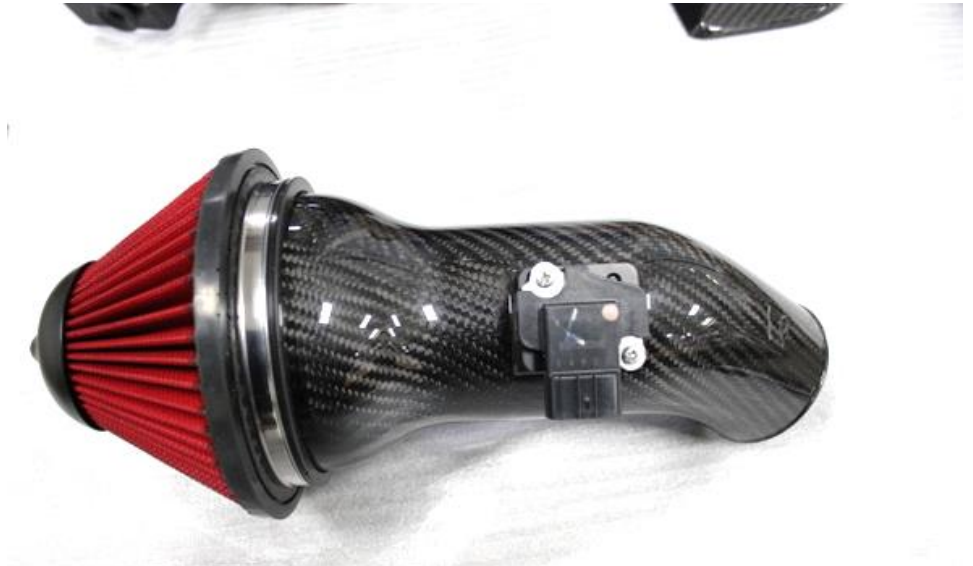
22. Install the sensor into the carbon tube and secure with the stock screws. Sensor should be oriented as shown.
