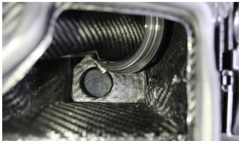
32. As you lower the airbox – make sure the scoop sits in place around the hole at the base of the airbox. The rubber edging on top of the scoop should seal against the base of the airbox.
