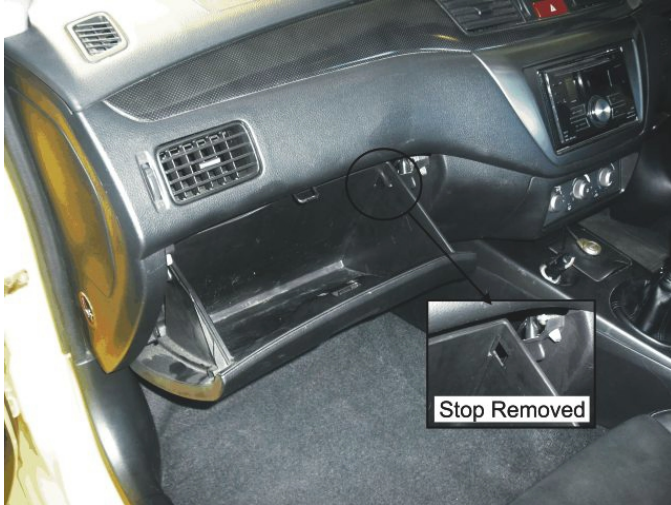
Figure 3 - Glove Compartment Removal
