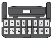
AUXILIARY CONNECTOR (16 PIN) REAR VIEW (WIRE SIDE)
