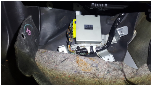
Figure 3 - Factory ECU is now ready for removal.
