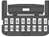
AUXILIARY CONNECTOR (16 PIN) REAR VIEW (WIRE SIDE)
